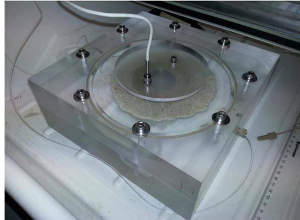
**Figure 2-40** (left): Schematic arrangement of the bentonite erosion experiment. 1. spacer 2. compacted bentonite 3. aperture of 1 mm height fracture 4. acrylic glass in contact, seals the arrangement; Arrows at top and bottom: water inlet and water outlet. (right): Bentonite erosion experiment set-up as installed in the lab. Pressure monitoring sensor on top (white cable).
