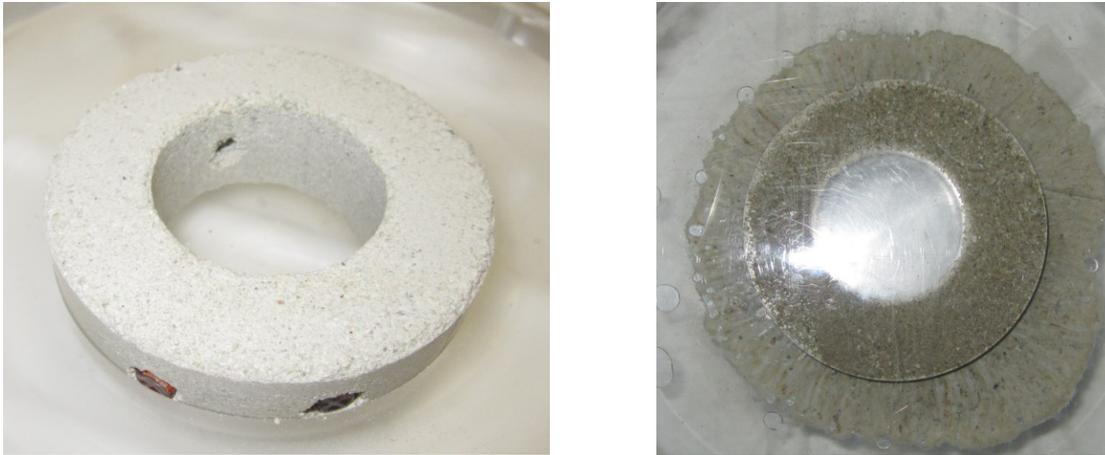
**Figure 2-41:** (right) Bentonite sample with holes on side of the ring containing filled glass vials. (left) Top view of the bentonite ring in the swelling stage.
