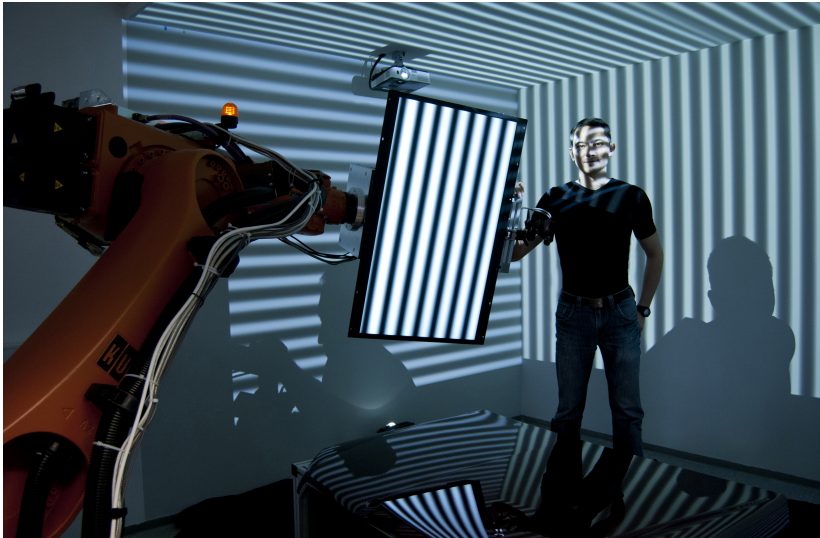
Figure 1.5: Stationary platform: KUKA robot hand for autonomous deflectometric inspection of varnish coating at IES laboratory [Leh11].
