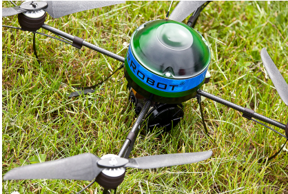
(a) Aerial reconnaissance drone; ©Fraunhofer IOSB, photo Manfred Zentsch
