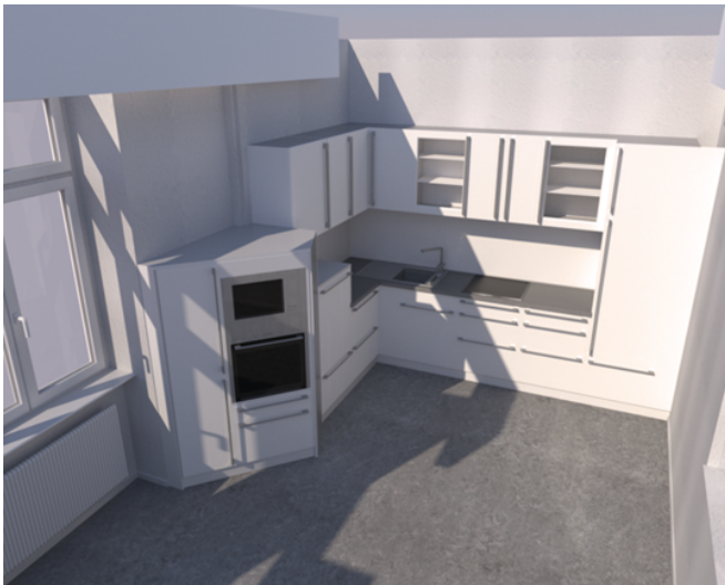
(b) 3D kitchen model after manual processing of the raw data (combining triangles into flat surfaces, segmenting and semantic labeling of representatives, etc.);
