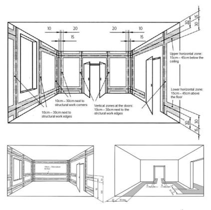
Figure 4-8: Vertical and horizontal wiring conduit zones in residential buildings<sup>15</sup>
