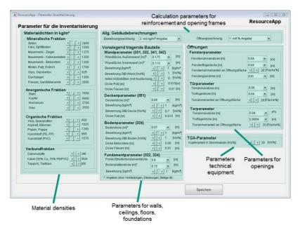
Figure 5-5: Graphical user interface for building element properties (material densities, dimensions, reinforcements)
