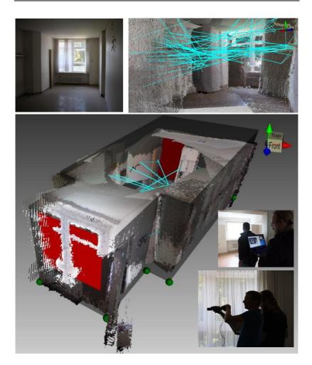
Figure 5-30: Interior patient room, top and bottom: point cloud and 3D reconstruction (Fraunhofer IGD), top right: photograph of the patient room reconstructed in images left, bottom right: 3D sensor users in a patient room Table 5-13: Numbers of automatically recognized vertices, faces and building elements (from CSV interface)
