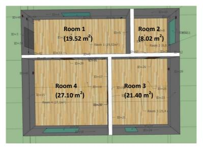
Figure 5-2: Vertical projection (floor plan) with the room numbers and their floor area [m<sup>2</sup>] in the Google SketchUp model for the exemplary four-room apartment (case study 1)
