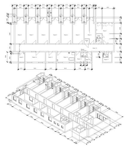
Figure 5-32: Case study 2 (2. floor of hospital) with modeled floor plan based on manually audited building elements represented in Autodesk Revit (top: floor plan; bottom: 3D view in isometric projection<sup>14</sup>)
