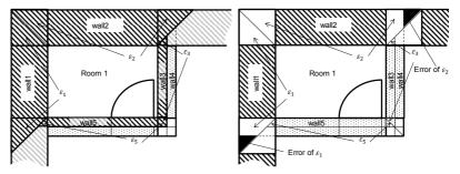
Figure 4-7: Schematic cutaway floor plan of exterior and interior walls in volume calculation (black hatched parts in left sketch) and wall error in the case of adjacent wall with differing thicknesses (black triangles in right sketch)
