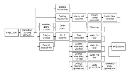
Figure 2-8: Exemplary deconstruction activity precedence in a three-storey building deconstruction project<sup>37</sup>
