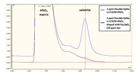
Figure 22: Se species determinations in the Double Spike solution with IC – the highest peak was caused by nitrate from the HNO<sub>3</sub> matrix, the only other peak was proved to be selenite by doping the Double Spike with pure selenite solution in high concentration.
