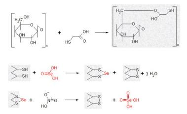
Figure 30: Purification mechanisms in method (B): Activation of cellulose powder with thioglycolic acid (upper), binding of selenite to thiol groups as innerspheric complex (central), extraction of Se from TCP with HNO<sub>3</sub> (lower) (modified from Elwaer and Hintelmann, 2008c).
