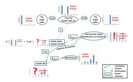
Figure 19: Schematic diagram of the Double Spike technique for the <sup>74</sup>Se/<sup>77</sup>Se Double Spike (modified from Rudge et al., 2009).
