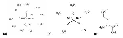
Figure 40: Molecular structure of all three Se species used – (a) sodium selenate  $(Na_2SeO_4 x 10 H_2O)$ , (b) sodium selenite  $(Na_2SeO_3 x 5 H_2O)$  and (c) selenomethionine (SeMet) (C<sub>5</sub>H<sub>11</sub>NO<sub>2</sub>Se).
