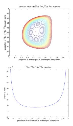
Figure 20: Graph of error dimension depending on the <sup>74</sup>Se/<sup>77</sup>Se mix in the Double Spike and the Double Spike/sample mix; calculated with MatLab (provided by John Rudge, personal communication) (exemplarily for inversion with <sup>74</sup>Se, <sup>76</sup>Se, <sup>77</sup>Se and <sup>82</sup>Se).
