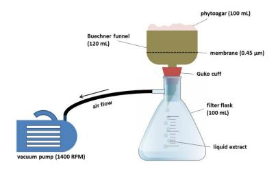
and funnels were used for each concentration and species, and cleaned with 5 %  $HNO_3$  followed by  $H_2O$  (millipore) after and before any usage.
