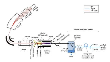
Figure 18: Scheme of HG-MC-ICP-MS analytics for Se isotope measurements (in parts modified from ThermoScientific (2015) and NRM (2015)).
