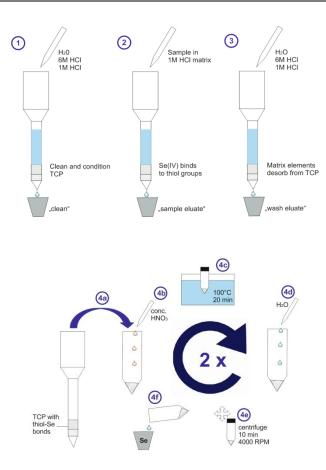
Figure 31: The four steps of purification according to method (B) – optimized from Elwaer and Hintelmann (2008c): 1) Activation of packing material in the column, 2) retention of Se in the packing material, 3) removal of matrix elements and 4) extraction of Se from the packing material by a) transferring to centrifuge tube, b) addition of HNO<sub>3</sub>, c) boiling in water bath, d) addition of H<sub>2</sub>O, e) centrifugation, f) removal of supernatant (afterwards repetition of b) to f)).
