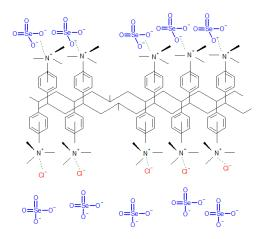
Figure 27: Molecular structure and retention/desorption mechanism in purification method (A) – selective outerspheric sorption of selenate (SeO<sub>4</sub><sup>2</sup>) ions and subsequent desorption by more competitive chloride (Cl<sup>-</sup>) ions.
