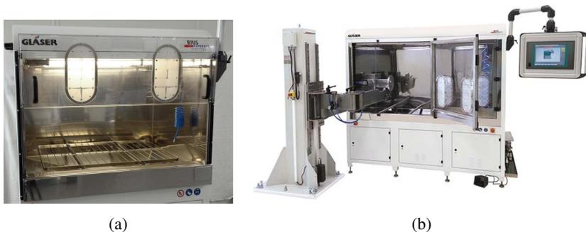
**Figure 1.1:** In the extraction step dirt particles are washed out of the examined technical good (a). A complete cleaning setup can be seen in (b). Images source: Gläser Company (Horb).
