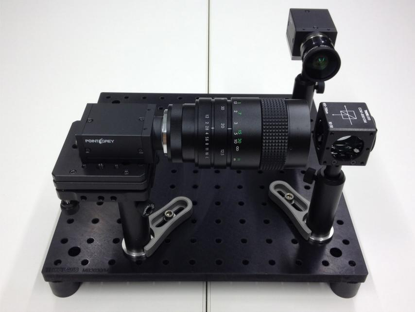
**Figure 2.3:** Prototype of the proposed system for capturing ground truth SR data
