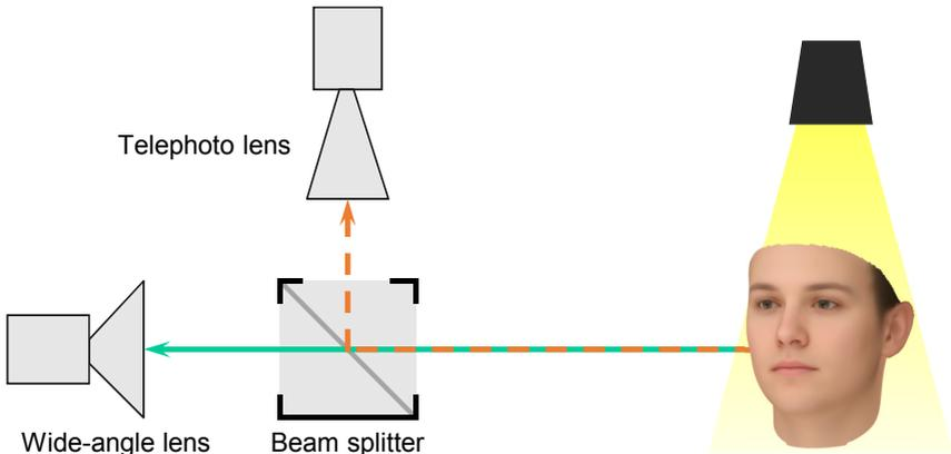
**Figure 2.1:** Scheme of the proposed system for capturing ground truth SR data
