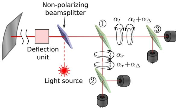
**Figure 3.1:** Design of the PSD with quarter-wave plates.
