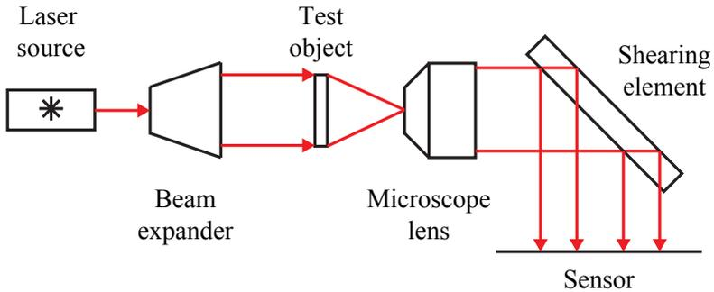
**Figure 6.1:** Transmissive optical shearing interferometer: An expanded coherent laser beam illuminates the test object. The transmitted light is collected by a microscope lens that magnifies the test object. A shearing element tilted by  $90^\circ$  directs the light onto a sensor, where the reflections from the shearing element's front and back surface interfere with each other. The resulting hologram is captured by the sensor.
