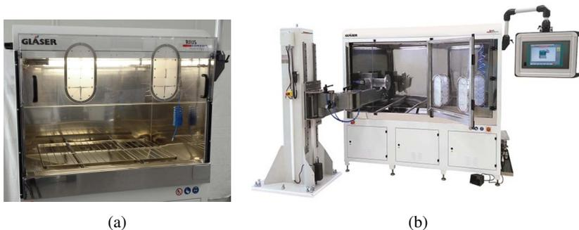
**Figure 1.1:** In the extraction step dirt particles are washed out of the examined technical good (a). A complete cleaning setup can be seen in (b). Images source: Gläser Company (Horb).
