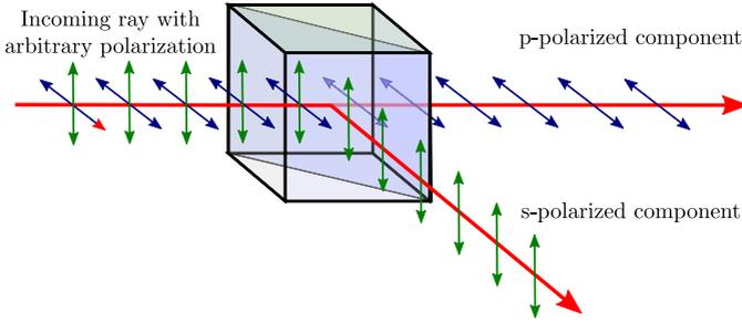
**Figure 2.1:** Transmission and reflection at a polarizing beam splitter.
