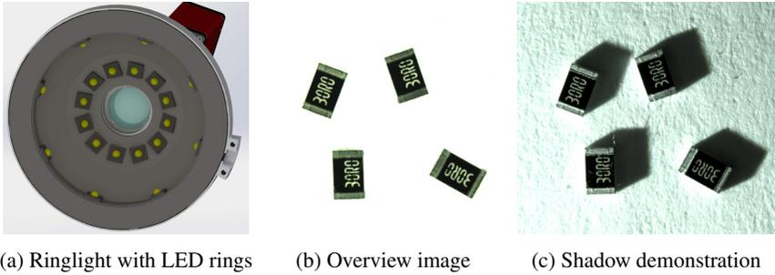
**Figure 1.4:** The illumination ring consists of two separately controllable LED rings (a). It can be used for uniformly illuminated overview images (b), while the lower ring produces sharp shadows (c).
