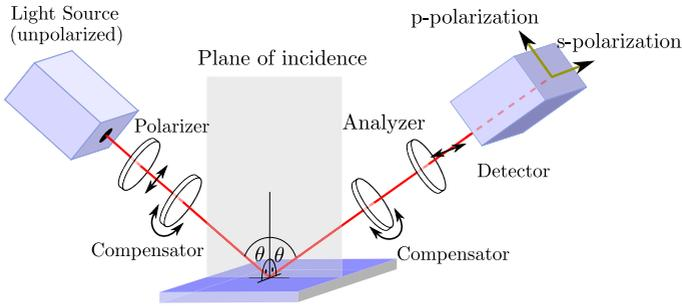
**Figure 1.4:** Conventional configuration of an ellipsometer.
