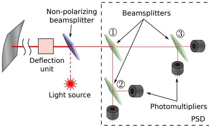
**Figure 1.2:** Design of the PSD inside the transceiver.
