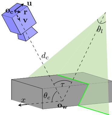
**Figure 2.1:** Geometry of a laser line scanner.
