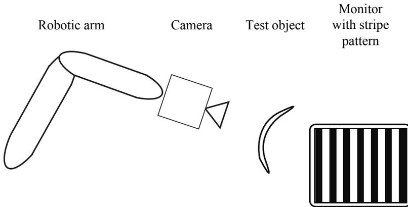
**Figure 5.1:** Structured illumination setup: A monitor realizes the ‘binary active lighting system’ and illuminates the test object. A camera observes the transmitted light. In order to inspect the whole test object, a robotic arm moves the camera to precomputed positions.
