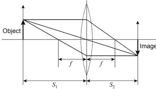
**Figure 2.2:** Image formation with a thin lens
