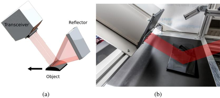
**Figure 1.1:** Scheme of the beam path with retroreflection (a) and an image of the ellipsometry scanner (b).
