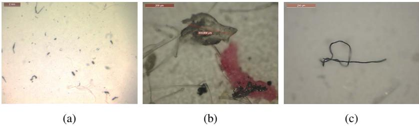
**Figure 1.2:** An overview acquired with a Leica Z-16 microscope is shown on (a). A detailed view of a conglomerate of particles in (b). It is further mandatory to unwrap eventual threads as seen in (c).
