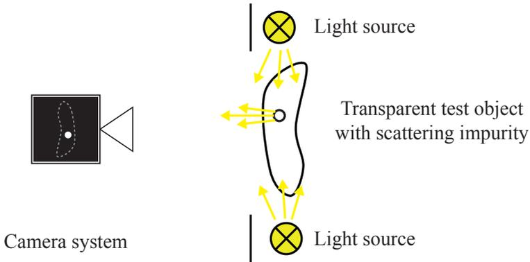
**Figure 3.1:** Conventional dark field inspection setup: One or more light sources, which are not in the camera’s view, illuminate the test object. Any scattering impurity inside or on the test object will scatter some light into the camera and will result in bright structures in the observed image.
