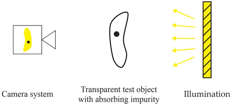
**Figure 2.1:** Conventional transmission inspection setup: An undirected light source illuminates the test object from one side. The transmitted light is observed by a camera system from the other side. Absorbing defects present in the test object appear as dark structures in the camera image.
