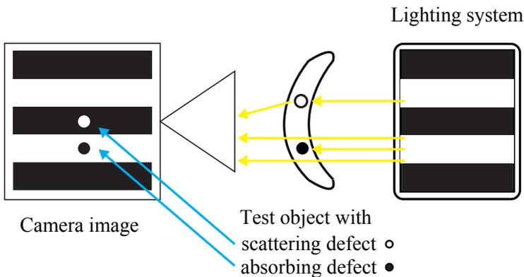
**Figure 5.2:** Defect visualization by means of the ‘binary active lighting system’: Absorbing defects are imaged to dark structures if illuminated by a bright stripe. Scattering defects are visualized by causing bright regions in the images of adjacent black stripes.
