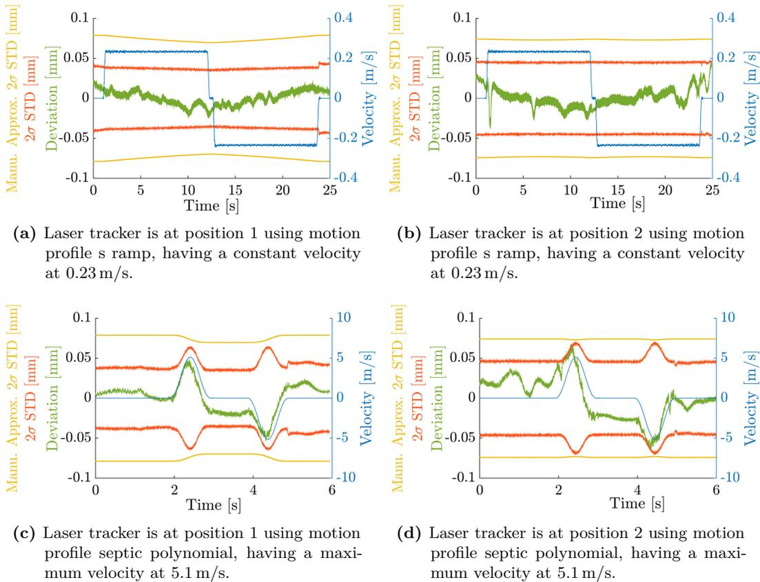
**Figure 6.18:** The results of the experiments using a s-ramp motion profile in the first row and a septic polynomial motion profile in the second row, while the laser tracker is at position 1 and 3.
