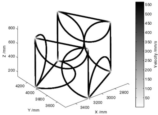
Figure 6: The reached speed for each point of the experiment.
