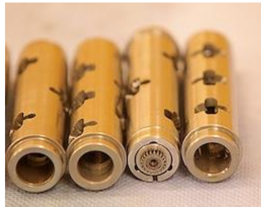
Figure 50: Hollow Shafts with Camshaft and Pawl Free-wheels (Staudt, 2011)
