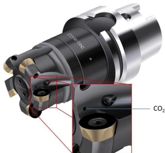
Figure 73: CO 2 Cooling Technology (Walter, 2013)
