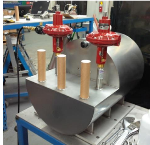
Figure 70: Sub-Cooler (5ME, 2014i, p. 35)
