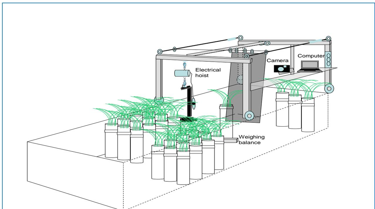
**Figure 6. Illustration of the IRRI lysimeter facility used in this study.** Water uptake was monitored by weighing of lysimeters using an electrical hoist suspended by a custom gantry crane. Lysimeter weights and digital images of shoots were acquired simultaneously to calculate Water Use Efficiency (WUE).
