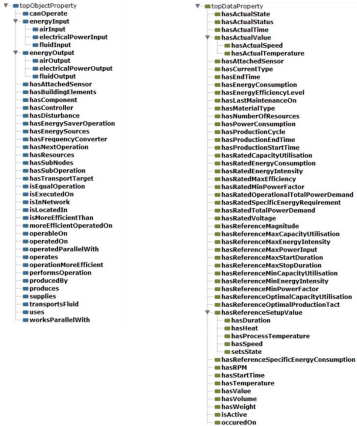
Figure 5.4 The object type and data type properties of manufacturing energy management ontology SERENE
