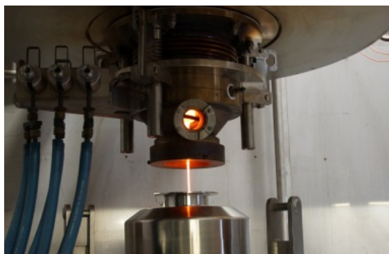
Fig. 9: Glass pouring operation to empty the PVA test melter after 6 years of idling conditions
