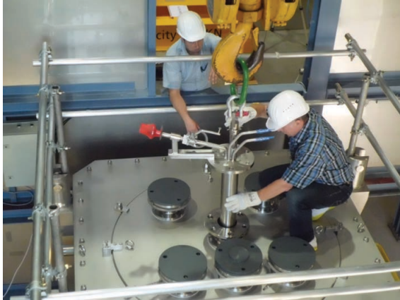
Fig. 2: Performance of the FAT. Adjustment of the feed inlet tube (see Fig. 1, position 8)
