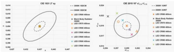
Figure 2: Identical color coordinates in the CIE 1931 2° compared to variations in the new 2015 10°. A visual evaluation of the shown spectra would lead to different visible white tones even if the measured color coordinates are exactly the same.
