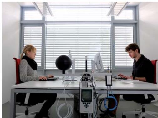
Fig. 4: Test room in the test facility LOBSTER. The workplaces are equipped with a luminance camera, illuminance sensors, a spectroradiometer, several temperature sensors and a humidity sensor.
