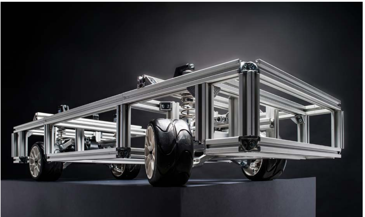
New drive and steering concepts for electric cars are tested with a scale model demonstrator.
