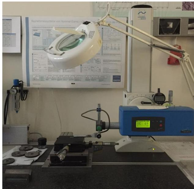
Figure 3.6: The photograph of a profilometer.
