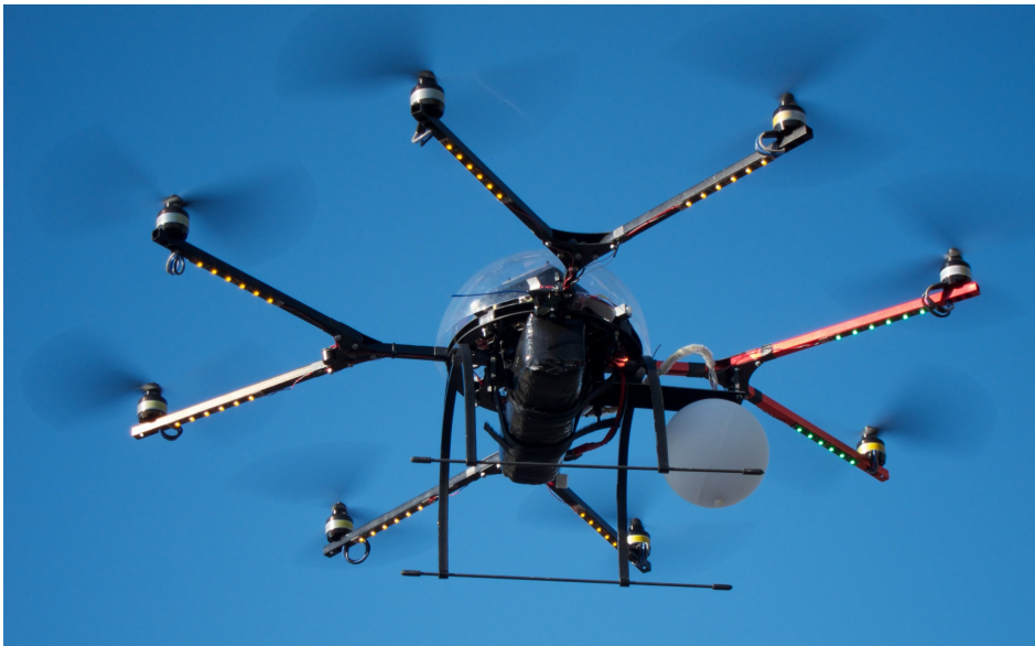
FIG. 5.3 Hovering Octocopter. The light source is mounted at the bifurcation of the two front arms (red), and the green and orange LED strips allow a visual cross-check of the orientation in the dark. All electronic boards are housed in the plastic dome. The black “brick” attached just below is the thermally isolated battery pack. Photo courtesy of Radomír Šmída.
