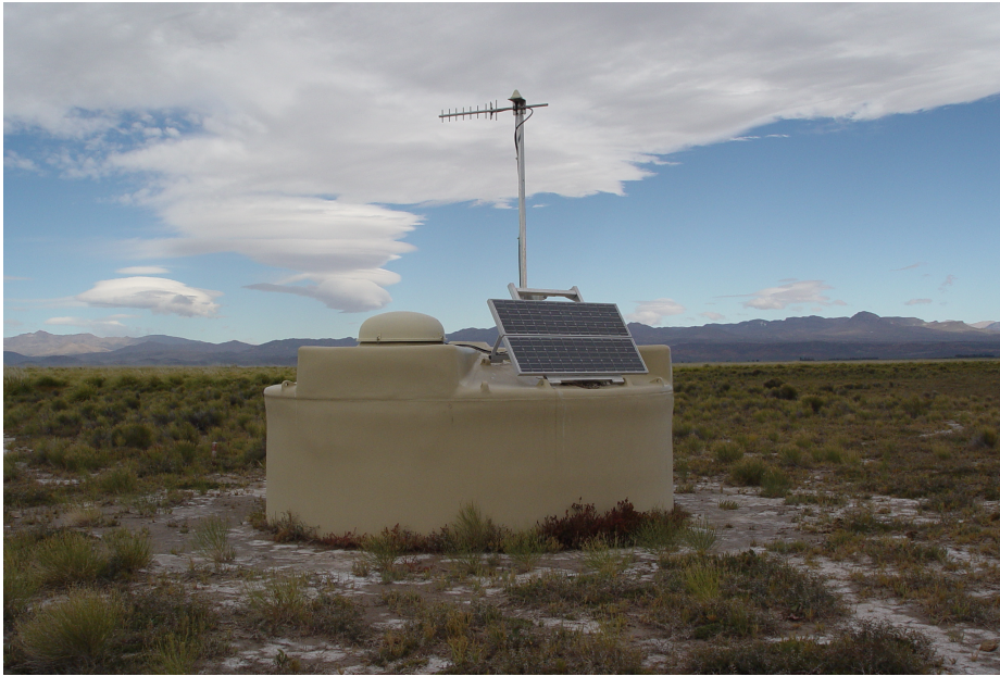
FIG. 2.10 One of 1660 surface detector stations of the Pierre Auger Observatory. The 1.2 m high vessel is filled with 12 000 liters of purified water, viewed from above by three large hemispherical PMTs. Mounted on top are a solar panel, and a communications and GPS antenna on a small mast. Photo courtesy of Radomír Šmída.
