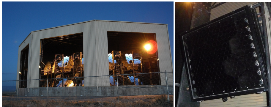
FIG. 2.23 Left: The Black Rock Mesa FD site at the Telescope Array. In contrast to the Auger fluorescence telescopes, here the aperture is fully open and photons impinge directly on the mirrors. Right: A UV filter covers the telescope camera directly. Photos courtesy of Radomír Šmída.
