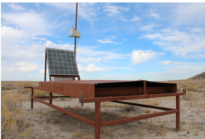
FIG. 2.21 A surface scintillator station at the TA site in Milard County, UT. The scintillator is protected by an iron housing, which also supports a solar panel, a battery and electronics box just underneath, and a small mast with a WLAN antenna. Photo courtesy of Ralph Engel.
