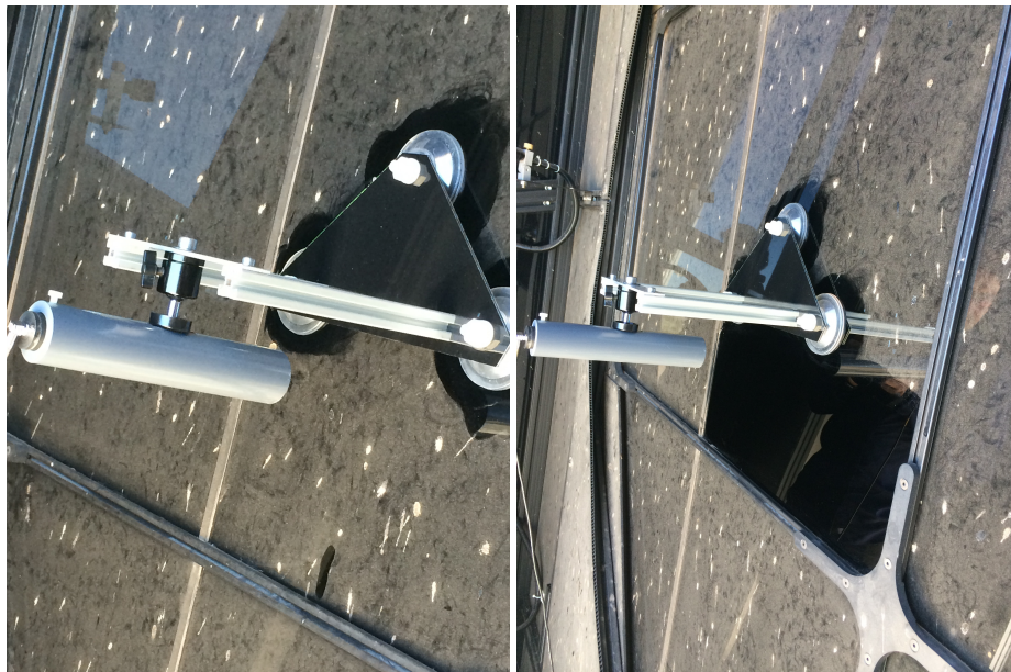
FIG. 4.26 The condition of the MUG-6 filter at LA1 in March 2014 before (left) and after (right) cleaning. The white spots on the uncleaned filter are bat droppings. Photos courtesy of Kai Daumiller and Hans Klages.
