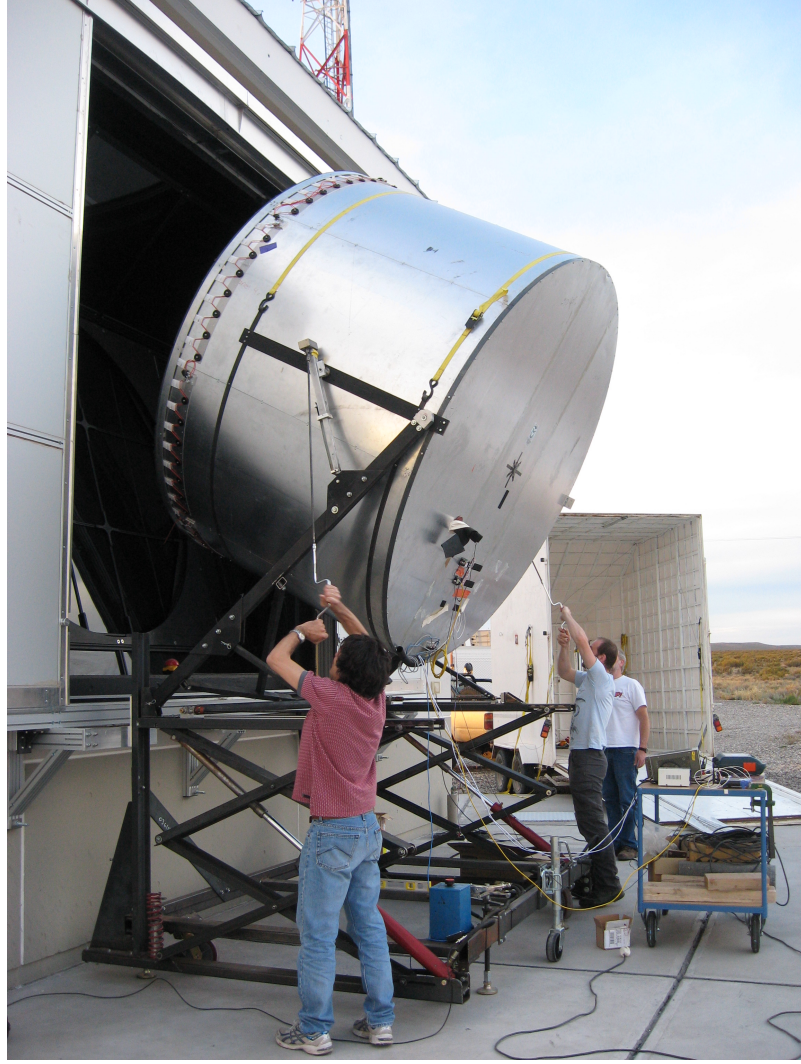
FIG. 3.2 The large-aperture light source used to absolutely calibrate the Auger fluorescence telescopes end-to-end is, for obvious reasons, referred to as the drum. Photo courtesy of Julia Bäuml.
