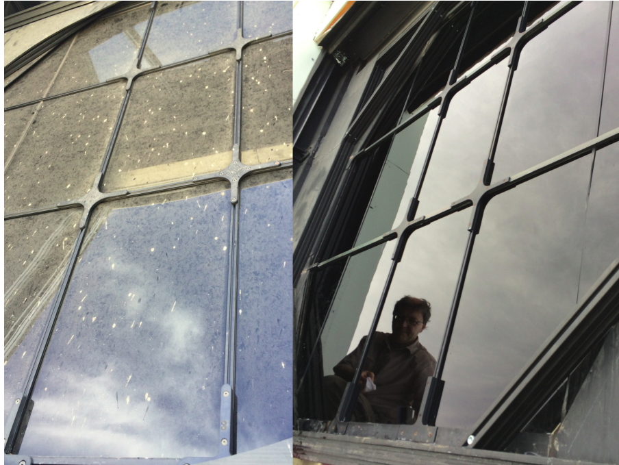
FIG. 4.26 The condition of the MUG-6 filter at LA1 in March 2014 before (left) and after (right) cleaning. The white spots on the uncleaned filter are bat droppings. Photos courtesy of Kai Daumiller and Hans Klages.
