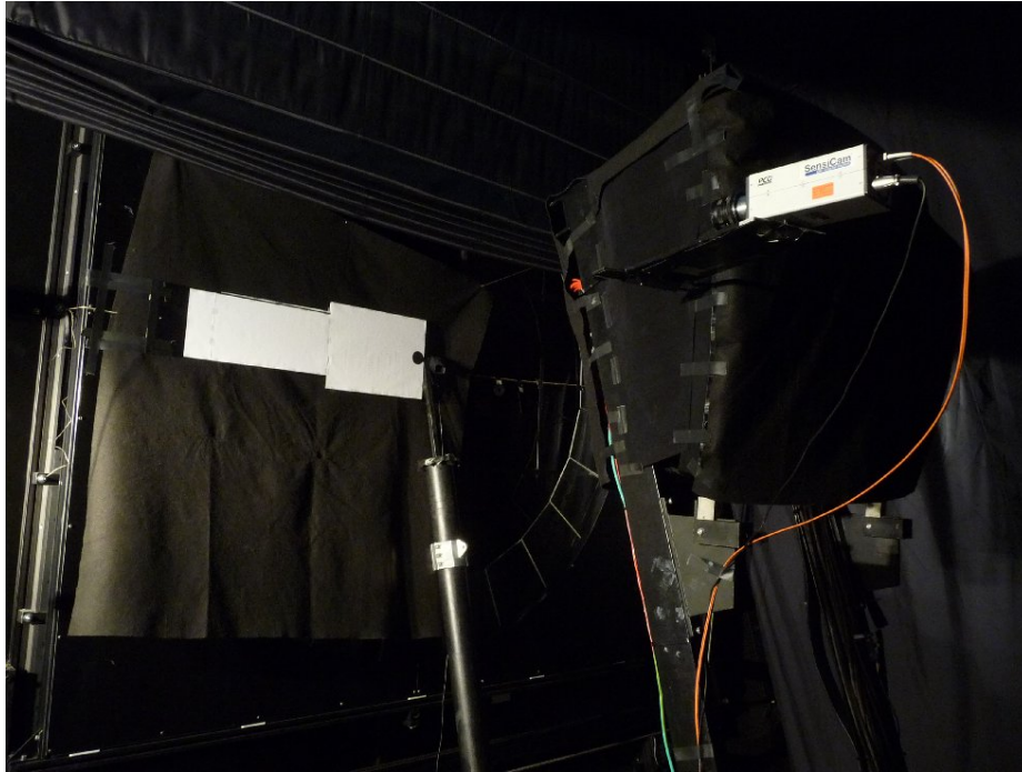
FIG. 4.4 The setup for the mirror measurement in CO5. The screen is positioned to the left of the CC, the light source just to the right. The CCD camera is mounted on the side of the actual FD camera. Both, the aperture and the FD camera are covered with black cloths to minimize multiple reflections.
