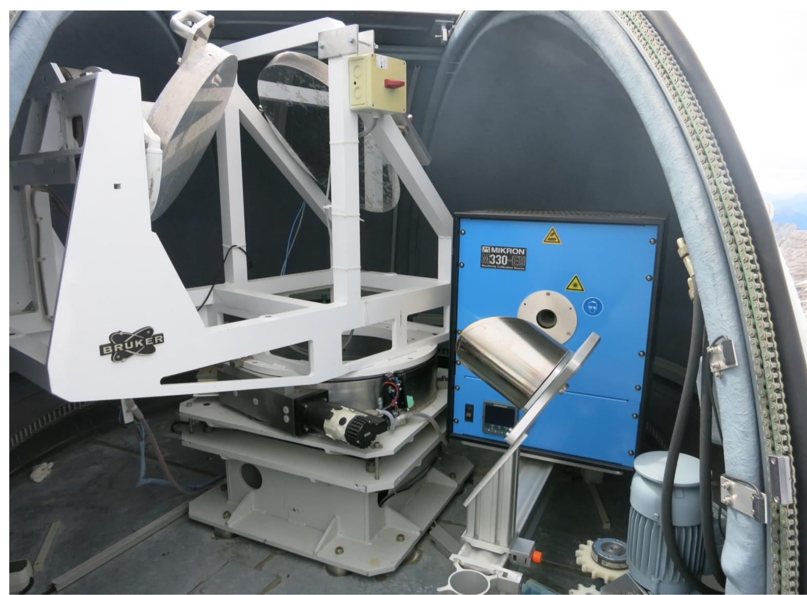
← NIR spectral radiance measurements: **Solar FTIR** (2500-7800 cm<sup>-1</sup>, Bruker IFS125HR interferometer)
