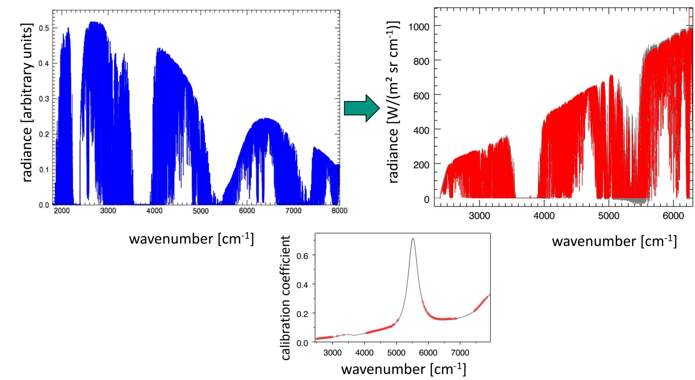
↑ Solar FTIR measurement (blue), calibration coefficients (middle panel) and comparison of calibrated spectrum (grey) with LBLRTM calculation (red)
