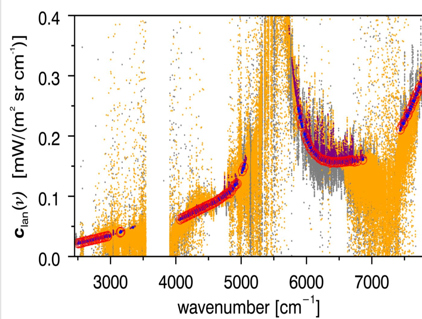
← Selection of suitable spectral points from initial Langley calibration results (grey). Selection based on avoiding solar lines (orange), low fit uncertainty (purple) and stability of fit result (blue). Final Langley results are averaged over 10 cm<sup>-1</sup>-bins (red circles)
