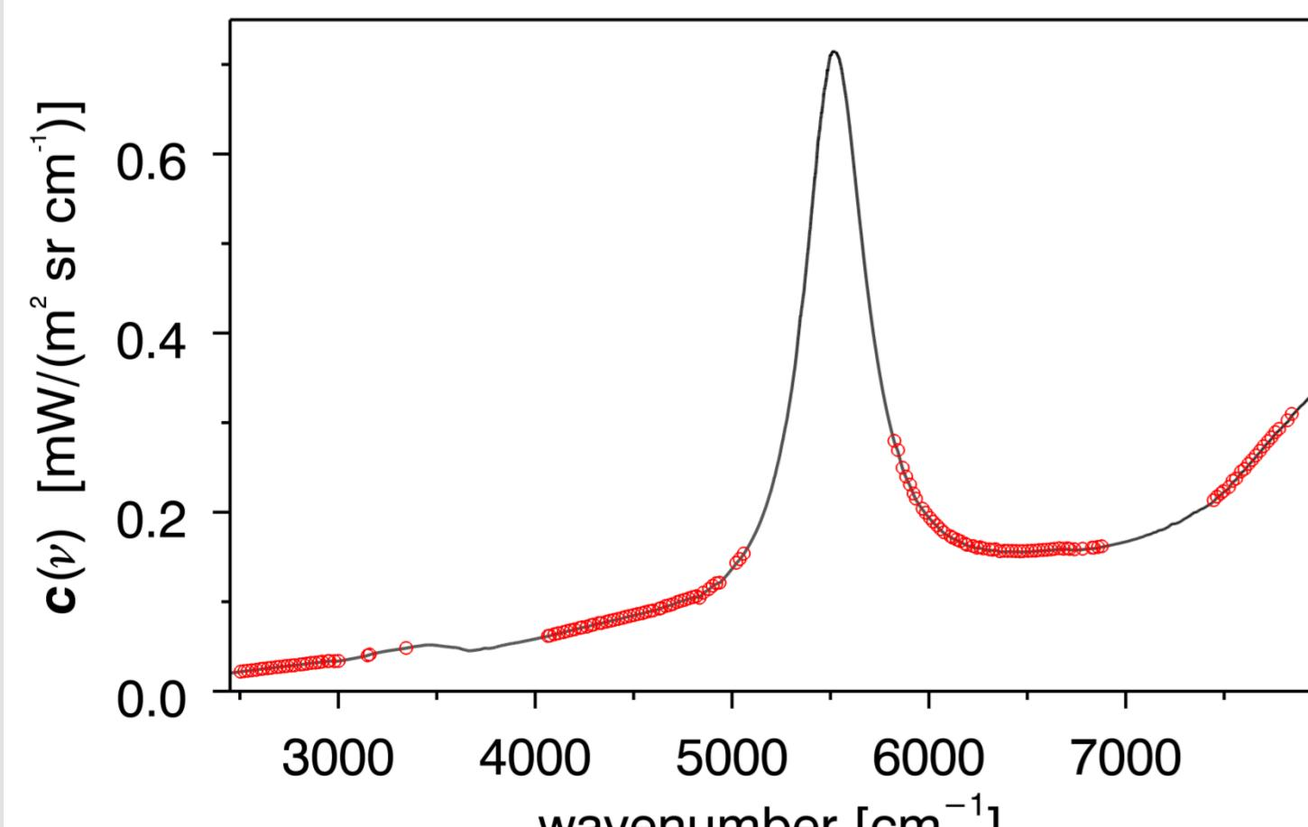
← Combined calibration curve constructed from Langley fit results in suitable windows (red circles) in combination with blackbody measurements (black line)
