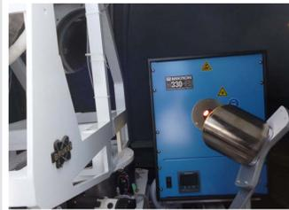
← High-temperature (1970 K) calibration blackbody source in the Zugspitze FTIR dome
