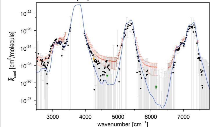
↑ Mean NIR water vapor continuum absorption coefficients derived from Zugspitze measurements (black), MT\_CKD 2.5.2 model (Mlawer et al., 2012) (blue), CRDS measurements of Mondelain et al. 2015 (orange), calorimetric-interferometric measurements of Bicknell et al. (2006) (green) and FTIR measurements of Ptashnik et al. (2012; 2013) (red)
