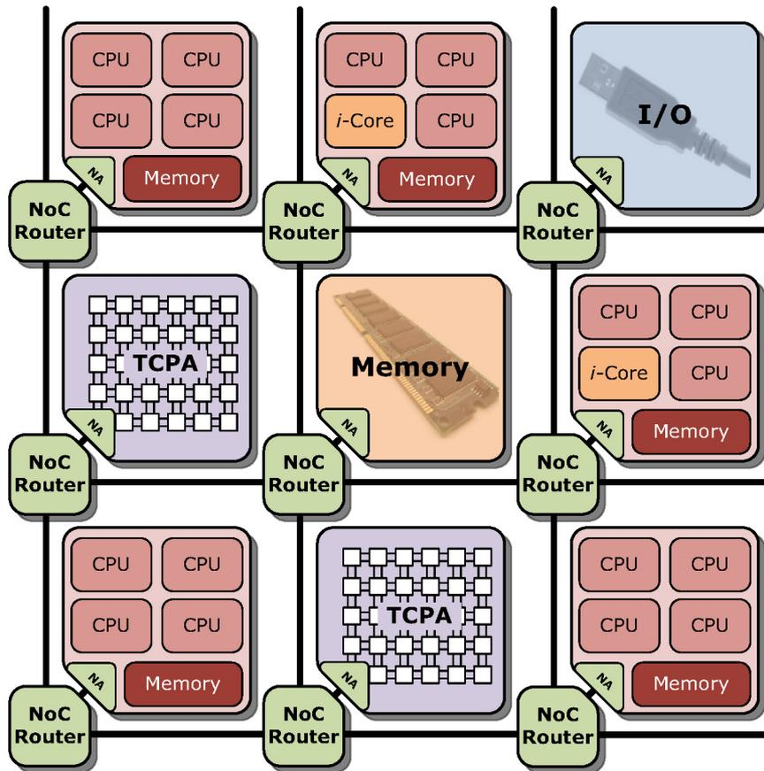
Figure 2.26: Tiled many-core developed in the scope of the Invasive Computing project (from [Hei14]). This 3x3 tile configuration shows the heterogeneous tiles used for computing, storage and I/O, connected by a NoC. the *i*-Core reconfigurable processor is available in two of the tiles.
