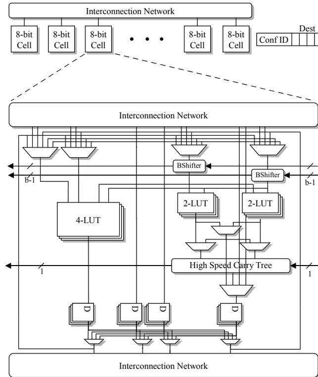
Figure 2.7: A row of logic cells in the ReMAP fine-grained reconfigurable fabric (from [WA10]).
