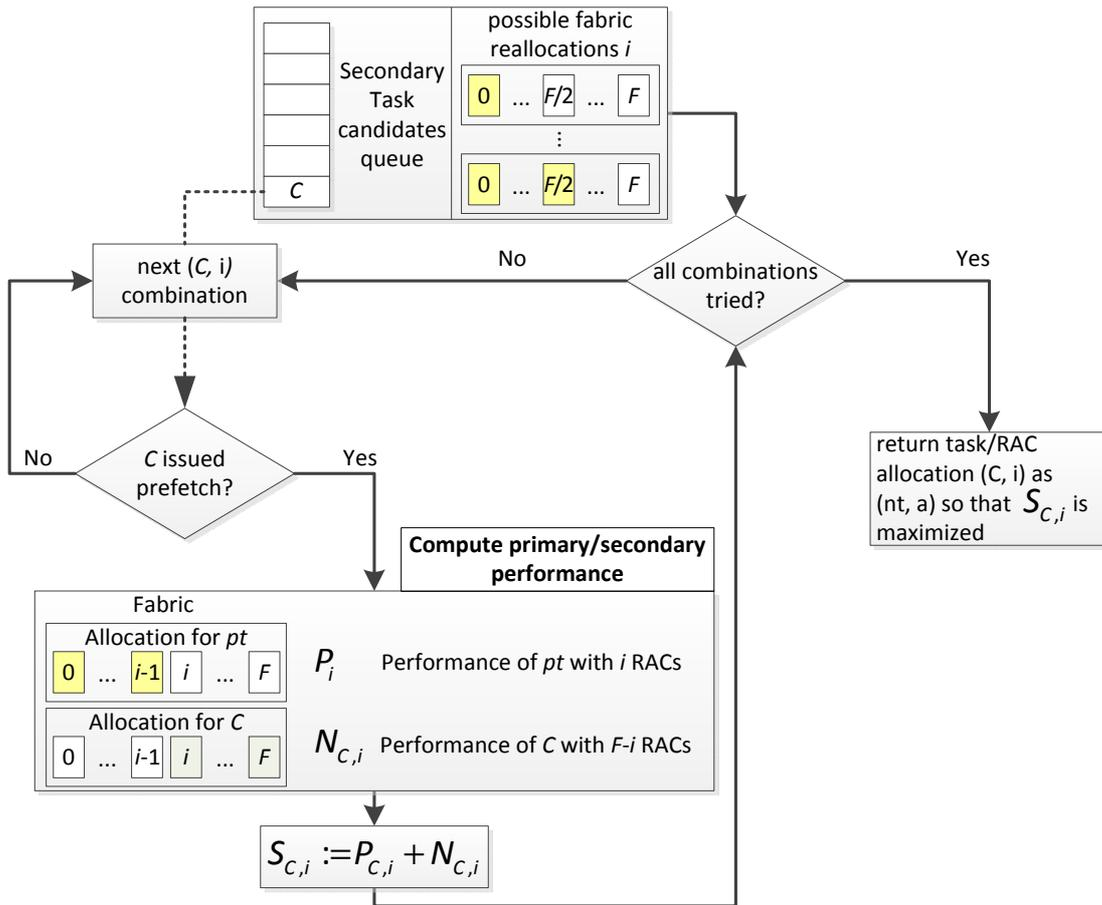
Figure 3.7: *Select Secondary Task* algorithm to determine a secondary task and amount of fabric for it to bridge the prefetch of the primary task.
