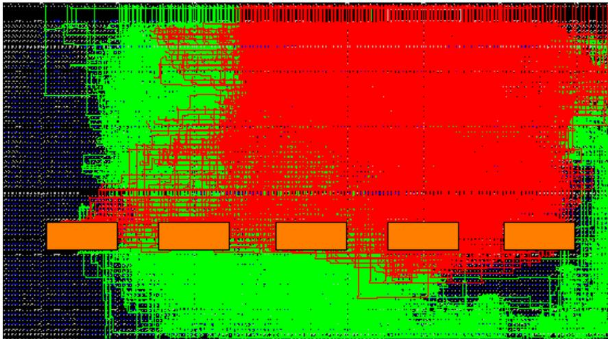
Figure 6.1: Floorplan of the *i*-Core on the Virtex-5 LX110T FPGA with routing resources highlighted. Red: Fabric and Interconnect, Green: GPP core, Orange: RACs.
