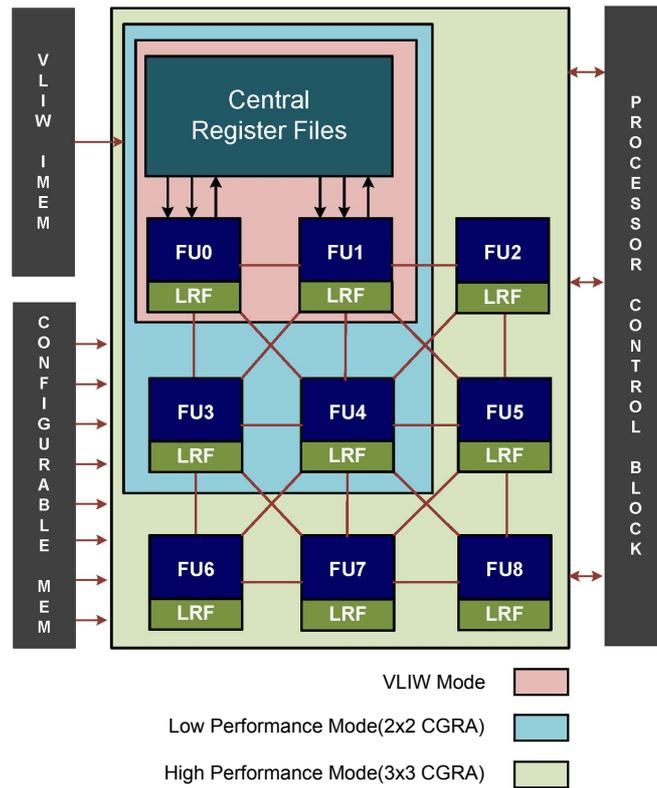
Figure 2.3: Ultra-Low Power Samsung Reconfigurable Processor with a 3x3 array of the coarse-grained ADRES fabric (from [KCCK+12]).
