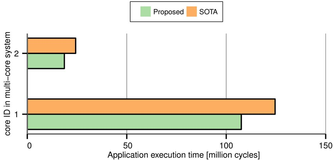
Figure 6.15: Comparison of the proposed Multi-tasking Reconfigurable Multi-Core Processor with a state-of-the-art approach.
