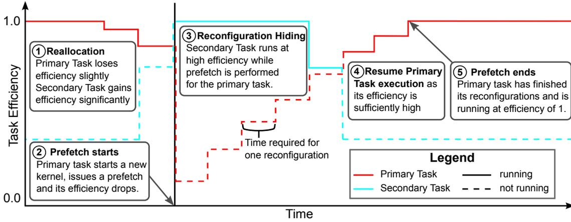
Figure 3.8: Efficiency of primary and secondary tasks in the proximity of a primary task prefetch.
