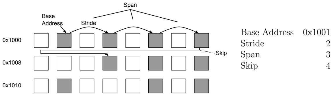
Figure 2.22: Example address pattern generated by programming the memory port with the parameters on the right.
