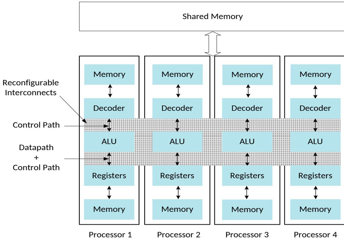
Figure 2.13: QuadroCore processor with reconfigurable interconnect between cores (from [Pur10]).
