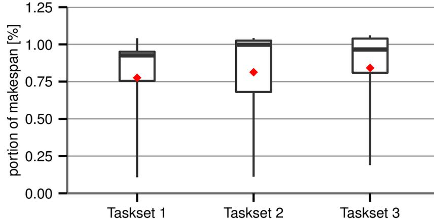
Figure 6.9: Overhead of MORP as share of the total makespan.
