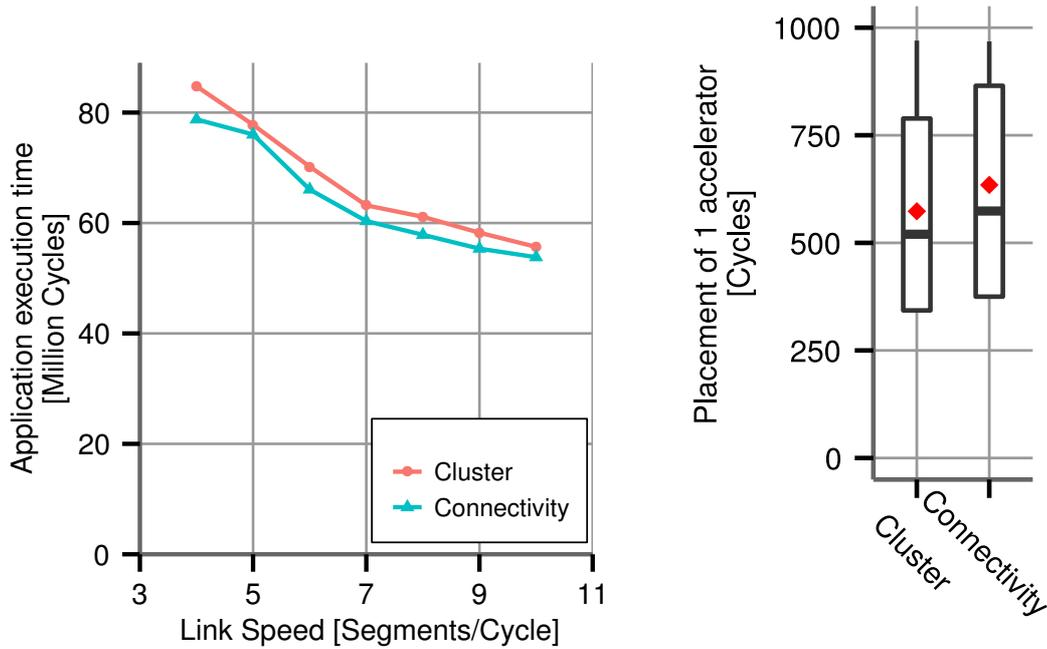
(a) Execution time of an H.264 video encoder using Cluster and Connectivity placements.
