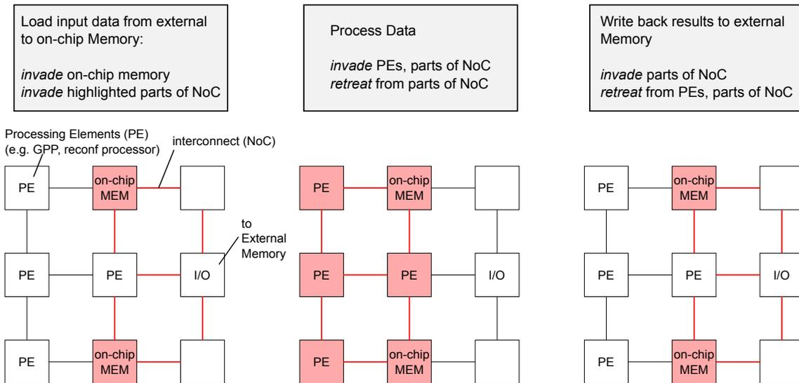
Figure 2.25: Example of an application with three distinctive phases running on an Invasive Computing platform. In each phase the application can request (“invade”) and release (“retreat”) resources.
