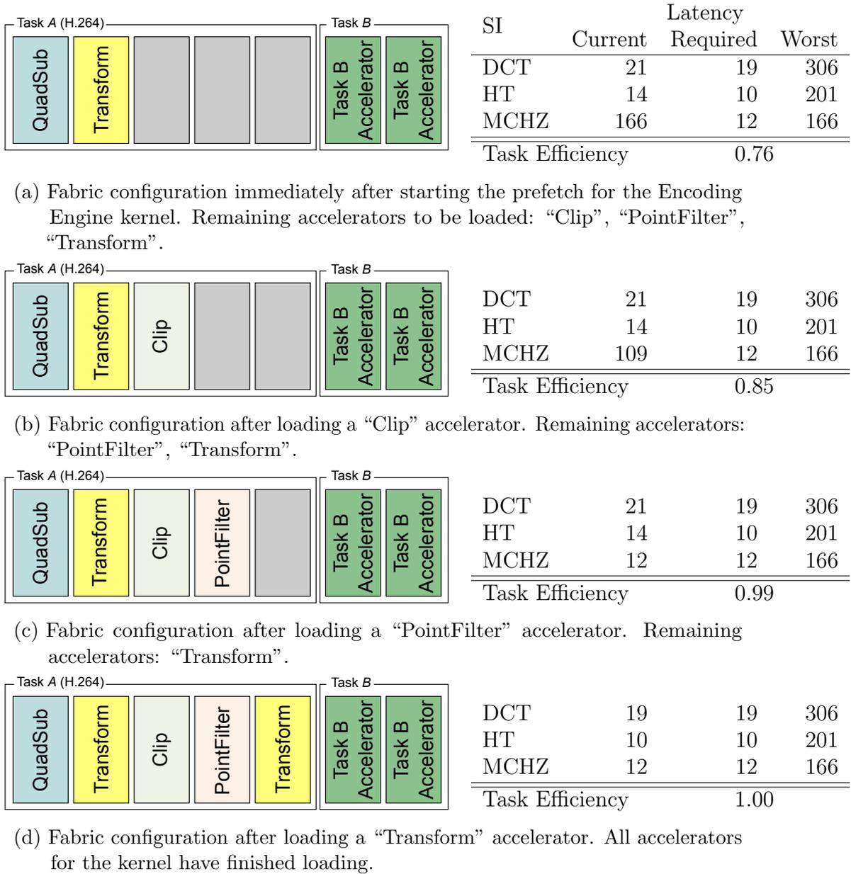
Figure 3.3: Varying task efficiency for an H.264 video encoder during loading of accelerators for the kernel “Encoding Engine”.
