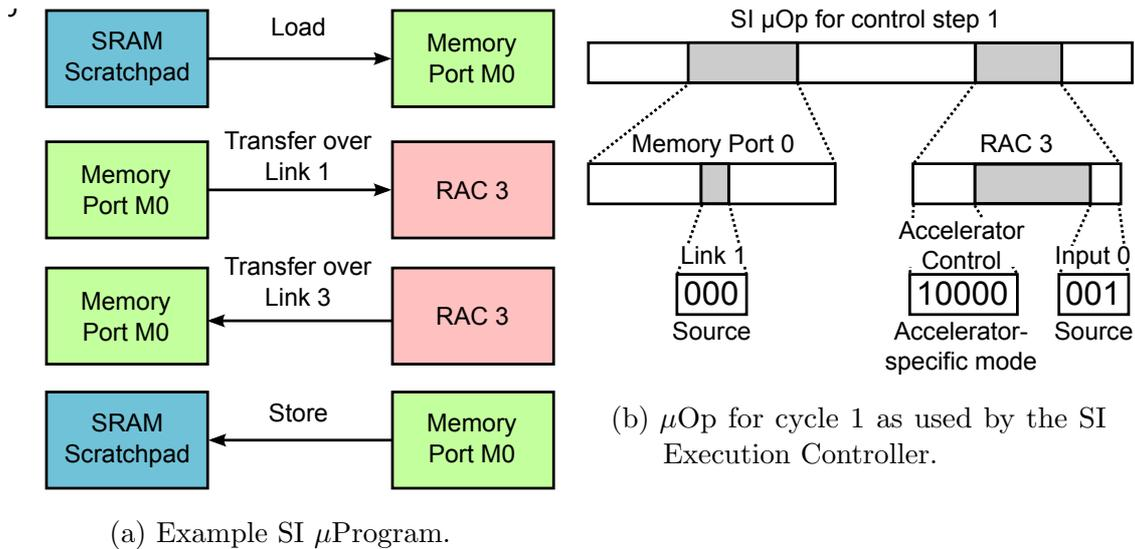
Figure 2.23: Example SI  $\mu$ Program and  $\mu$ Ops.
