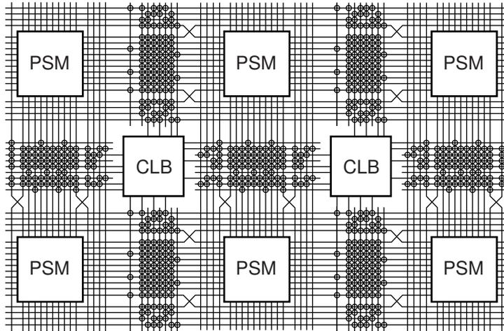
Figure 2.5: Fine-grained reconfigurable fabric in Xilinx Spartan FPGAs (from [Xil08]). CLBs (Configurable Logic Blocks) are used to implement logic. PSMs (Programmable Switch Matrices) are used to connect multiple CLBs to implement larger circuits.
