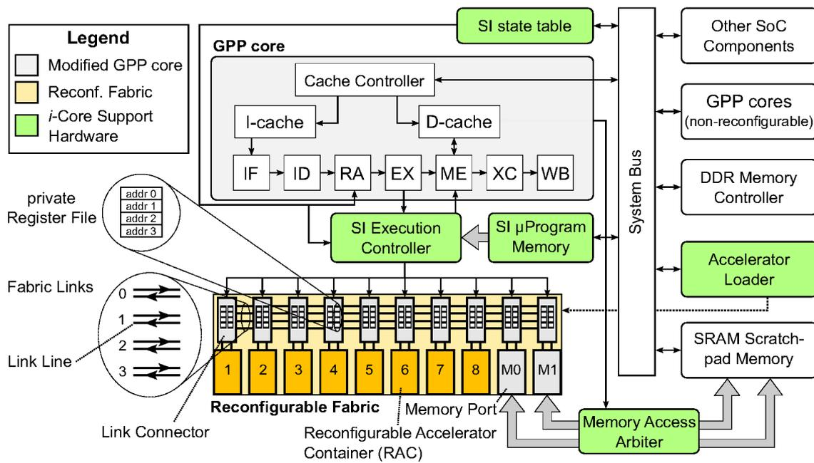
Figure 2.19: Architecture of the *i*-Core reconfigurable processor SoC.
