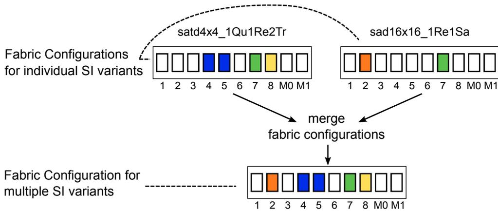
Figure 5.8: Merging of fabric configurations during placement for improved  $\mu$ Program cache hitrates.
