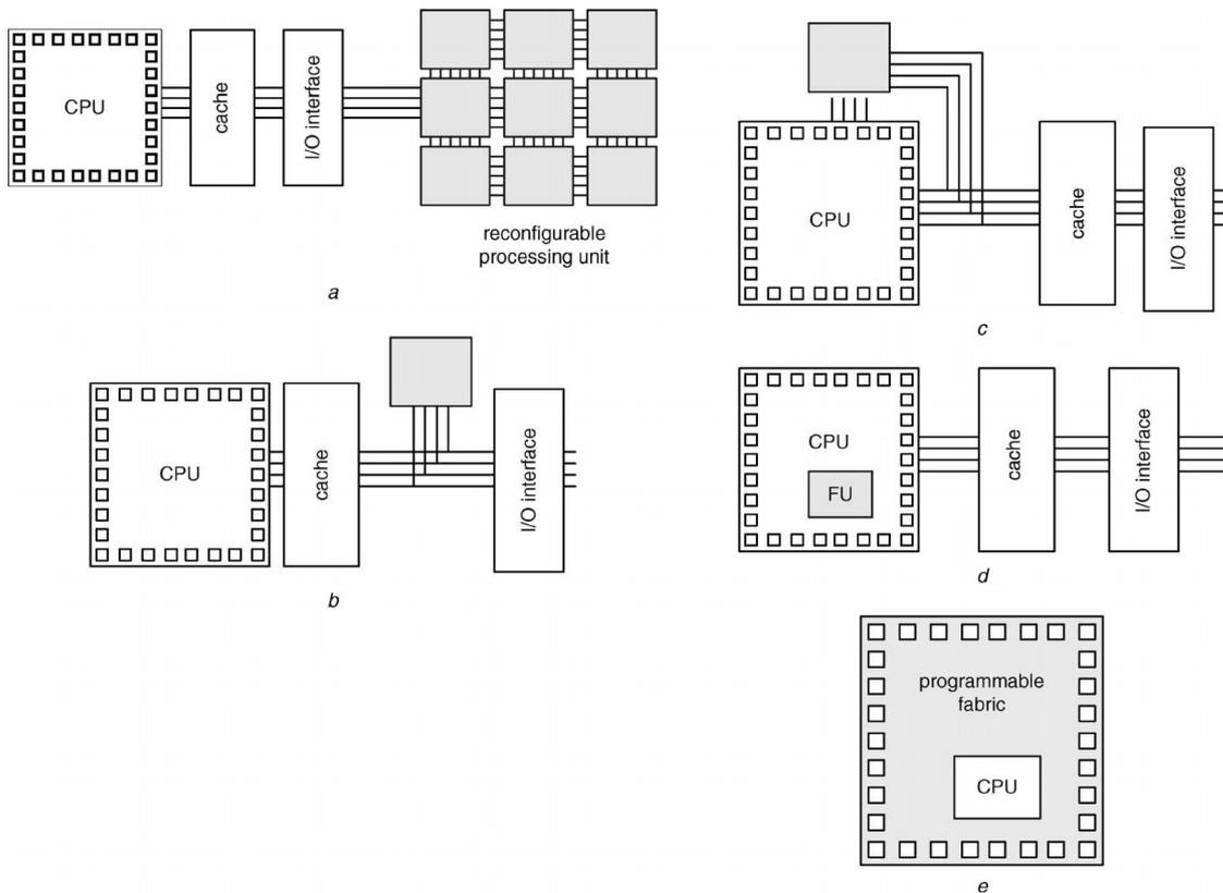
Figure 2.1: Different types of coupling (from [TCWM+05]). a) External stand-alone processing unit. b) Attached processing unit. c) Co-processor. d) Reconfigurable functional unit. e) Processor embedded in reconfigurable fabric.
