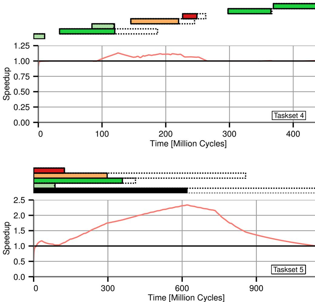
Figure 6.14: Comparison of a reconfigurable processor using partial online generated SI  $\mu$ Programs (proposed approach) vs. one using offline generated SI  $\mu$ Programs in a several multi-tasking scenario.
