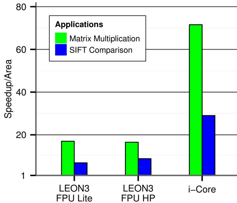
Figure 6.2: Matrix Multiplication and SIFT kernels on the *i*-Core. Comparison of area efficiency of *i*-Core SIs to LEON-3 with two different Floating-Point Unit (FPU) implementations (HP – High Performance).
