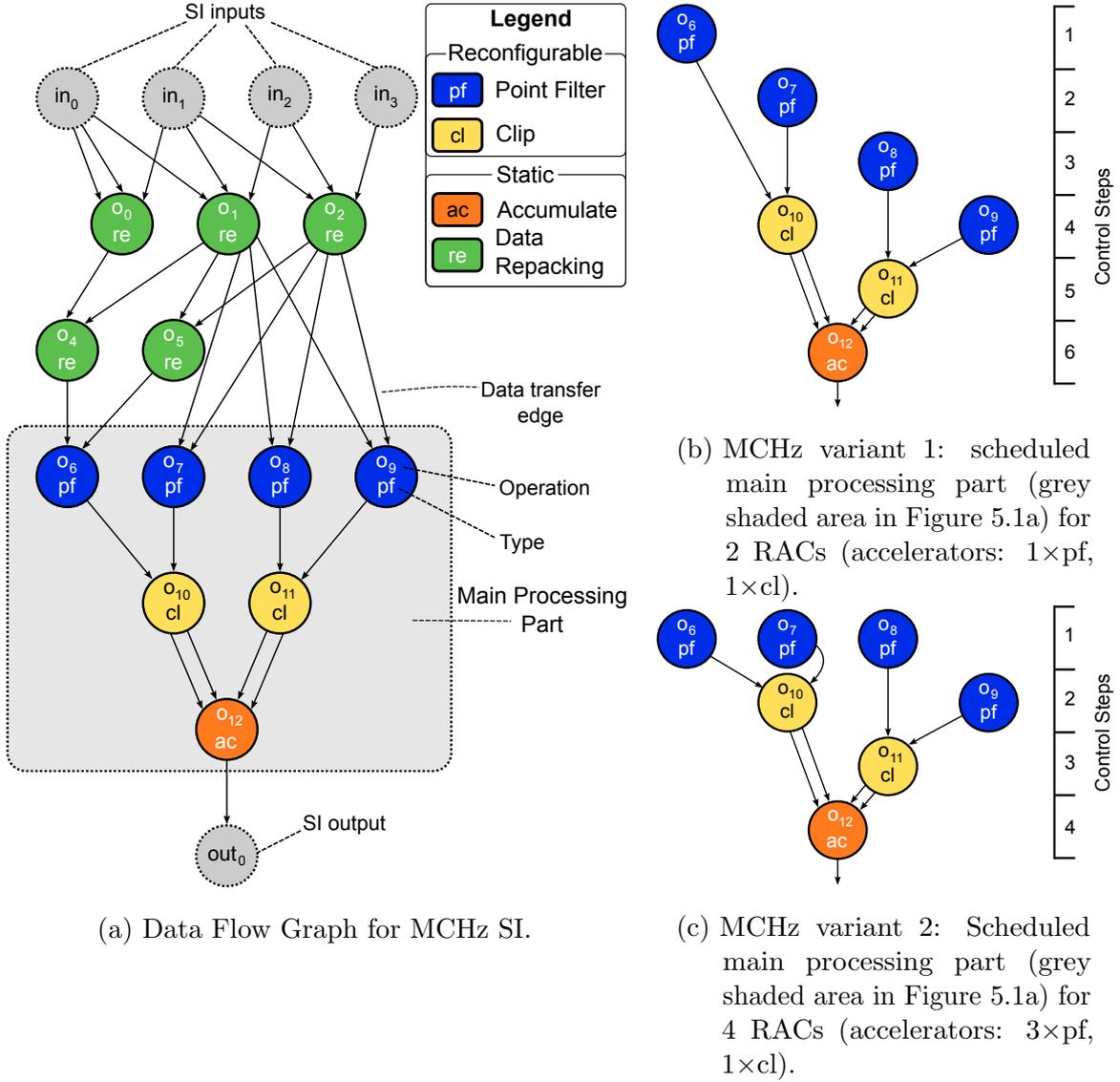
Figure 5.1: Data Flow Graph and schedules for 2 variants for the SI Motion Compensation – Horizontal from the H.264 Video Encoder application.
