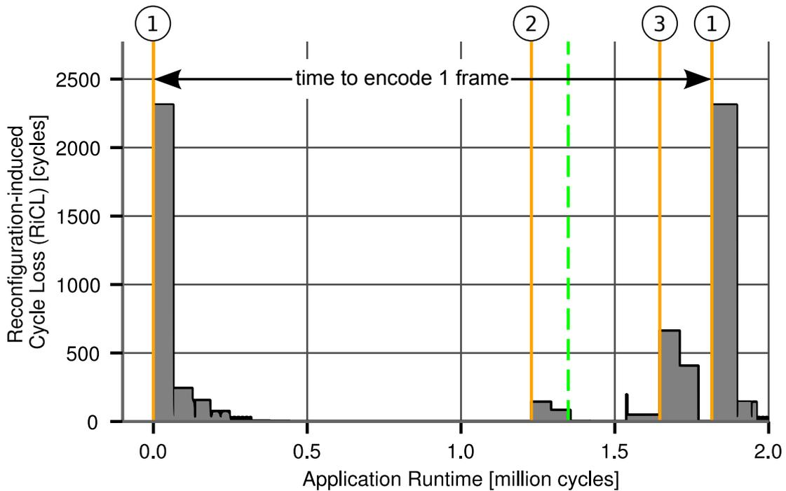
Figure 3.2: Performance loss in the H.264 video encoder due to reconfiguration overhead. The green dashed line shows when encoding would be finished if RiCL was zero.
