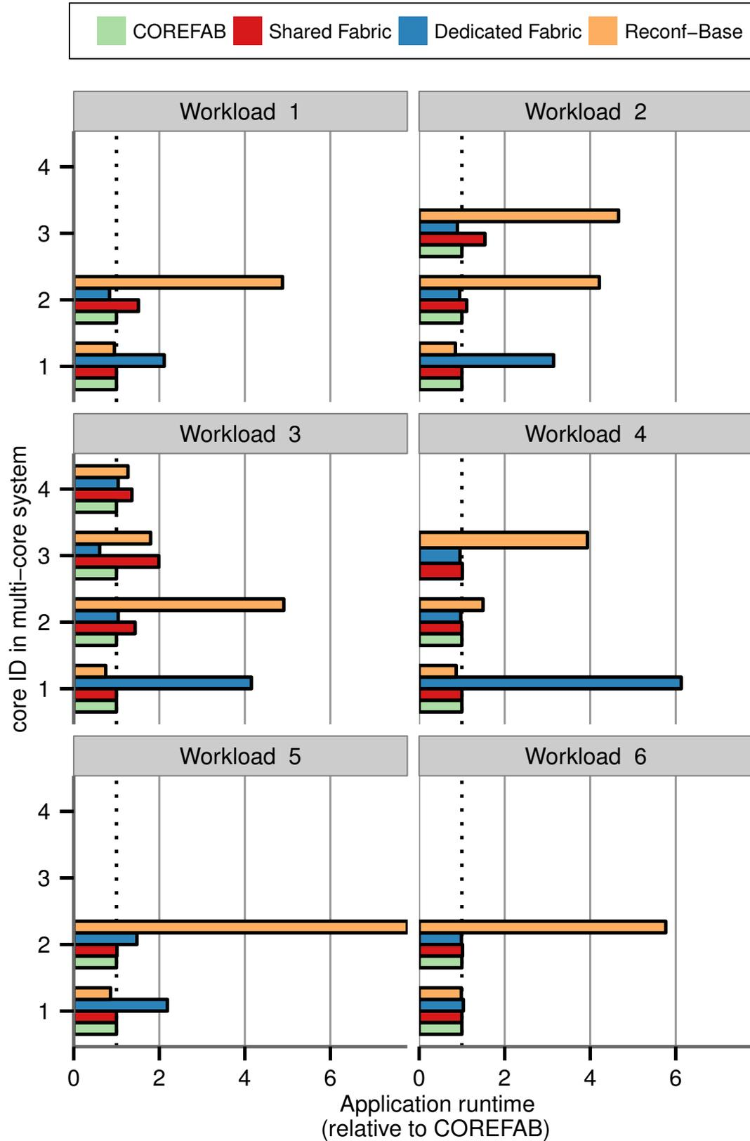
Figure 6.10: Normalized application execution time per-core (lower is better) of state-of-the-art fabric sharing strategies compared to COREFAB (dotted line at 1.0). Core ID 1 is the reconfigurable core, other cores are GPPs.
