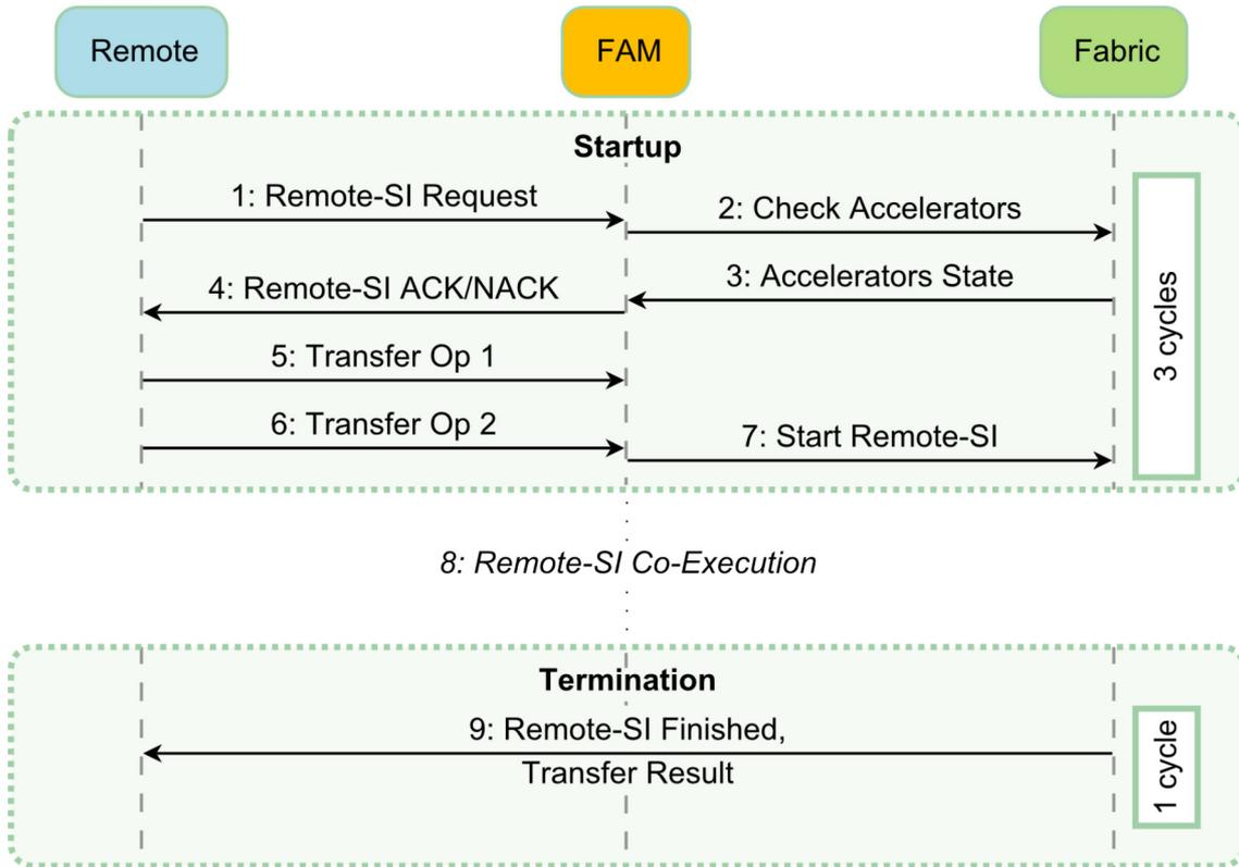
Figure 4.5: Message-Sequence chart for executing a Remote-SI. Communication between the remote core starting the Remote-SI, the Fabric Access Manager (FAM) and the Fabric is shown. The vertical axis is time.
