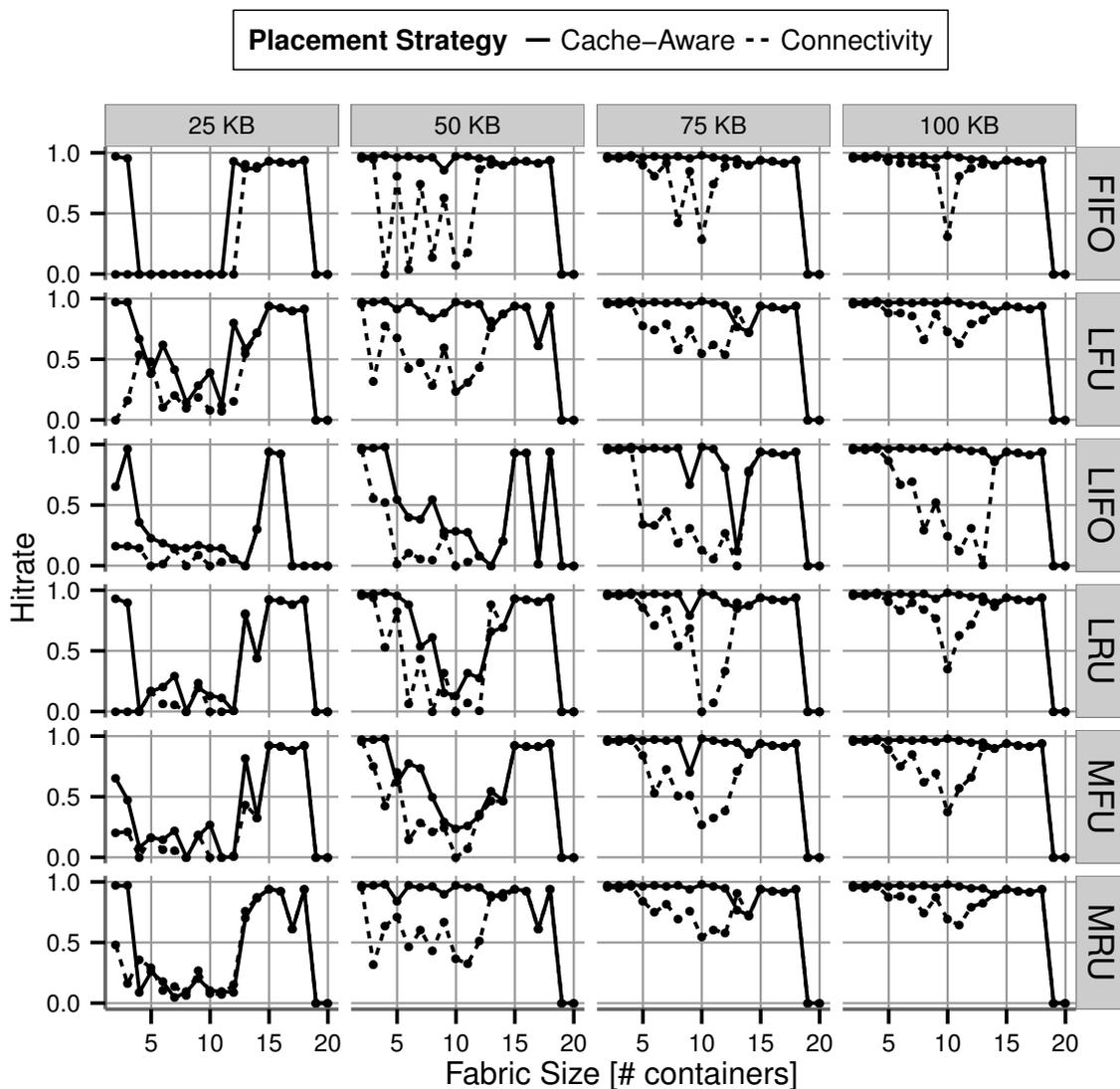
Figure 6.13: Hitrates for different  $\mu$ Program cache sizes, cache replacement policies and accelerator placement policies. A cold cache was used, thus the hitrates of 0 for 19 and 20 RACs are due to the fact that the cache was not accessed at all (the  $\mu$ Programs were generated once, and no further reconfigurations were performed due to the large fabric size).
