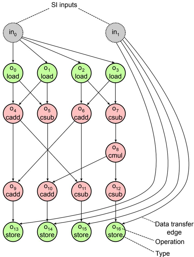
Figure 2.8: Data-flow graph for a 4-input FFT SI.
