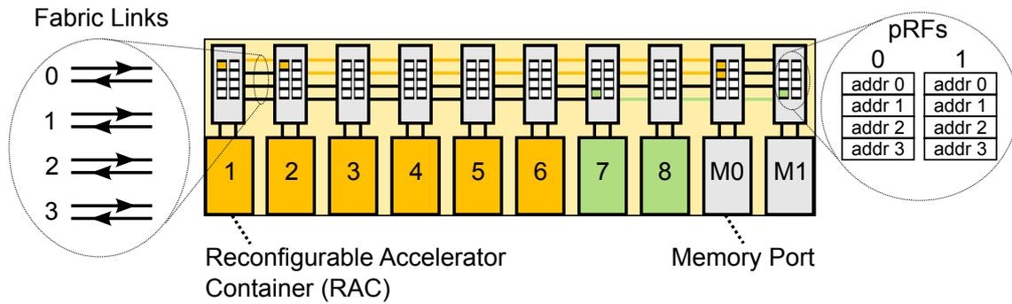
Figure 4.8: Example of fabric resources allocation for Primary-SI and Remote-SI  $\mu$ Programs.
