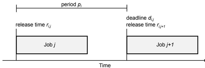
Figure 2.17: Release times, deadlines and period for periodic task  $T_i$  with implicit deadlines.
