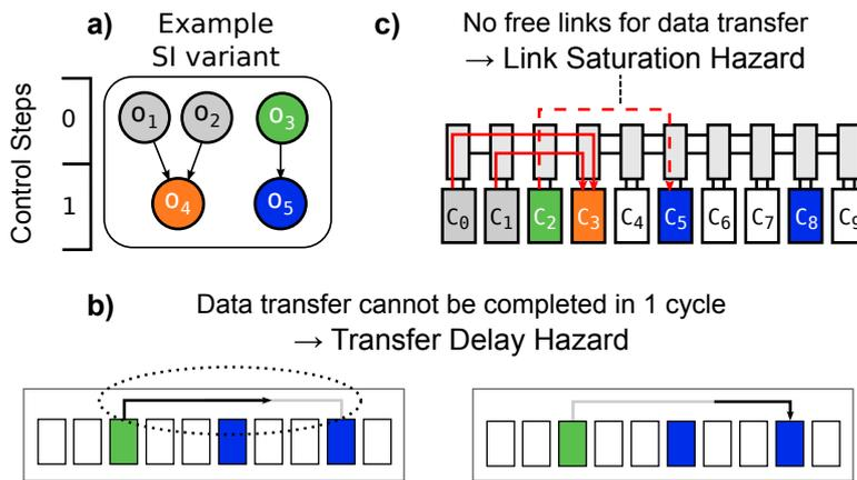
Figure 5.4: Examples for a Link Saturation Hazard (LSH) and Transfer Delay Hazard (TDH).
