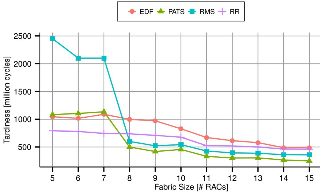
Figure 6.6: Tardiness (absolute value) for different fabric sizes (here shown for Taskset 4). Performance improves with increasing fabric size, resulting in improved tardiness as deadlines are met better.
