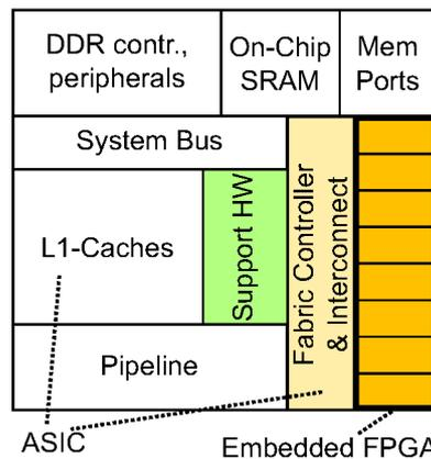
Figure 2.20: Envisioned floorplan of the *i*-Core reconfigurable processor SoC with the fabric implemented as an embedded FPGA.
