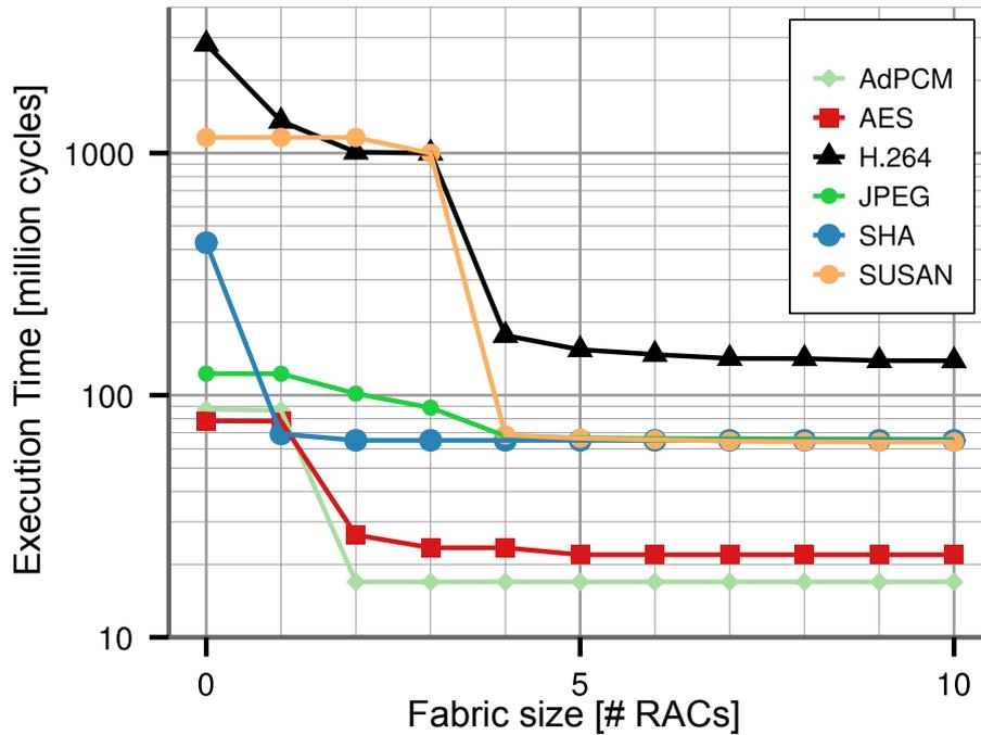
Figure 6.4: Application performance when run as single tasks on a reconfigurable processor. Speedup depends on fabric size and saturates for larger fabrics.
