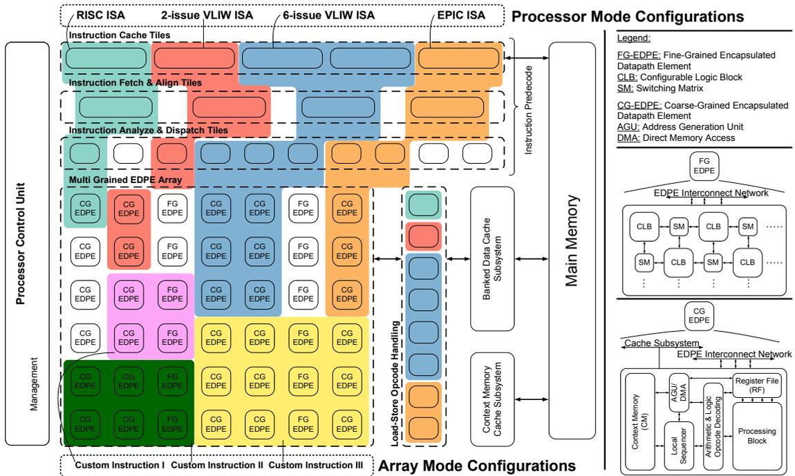
Figure 2.14: KAHRISMA reconfigurable system. Processor cores can be dynamically instantiated by combining front-end elements (“tiles” at the top) and coarse-grained reconfigurable processing elements (CG-EDPE) from the multi-grained EDPE array. The array can additionally be used to implement SIs (from [KBSS+10]).
