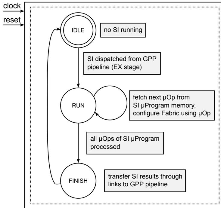
Figure 2.24: SI Execution Controller finite state machine for executing SI  $\mu$ Programs on the reconfigurable fabric.
