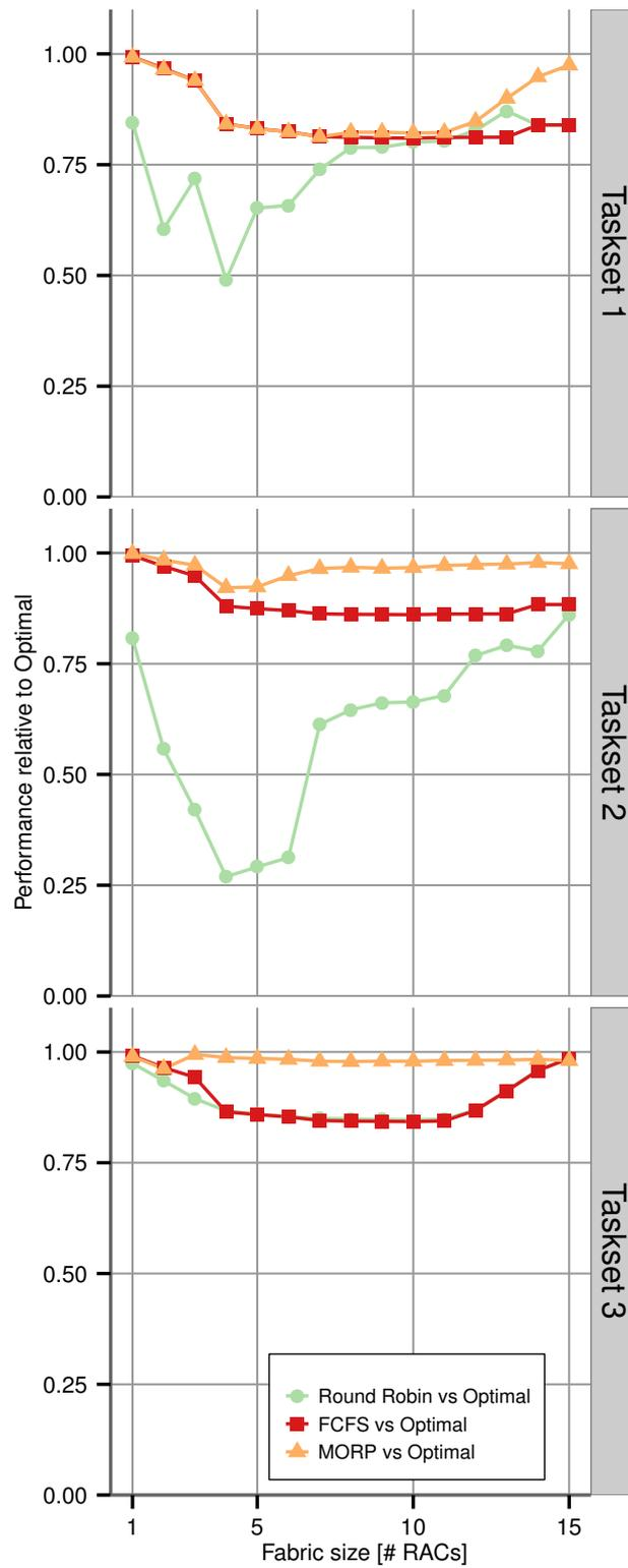
Figure 6.8: Relative speed of MORP, Round Robin and FCFS schedulers compared to Optimal.
