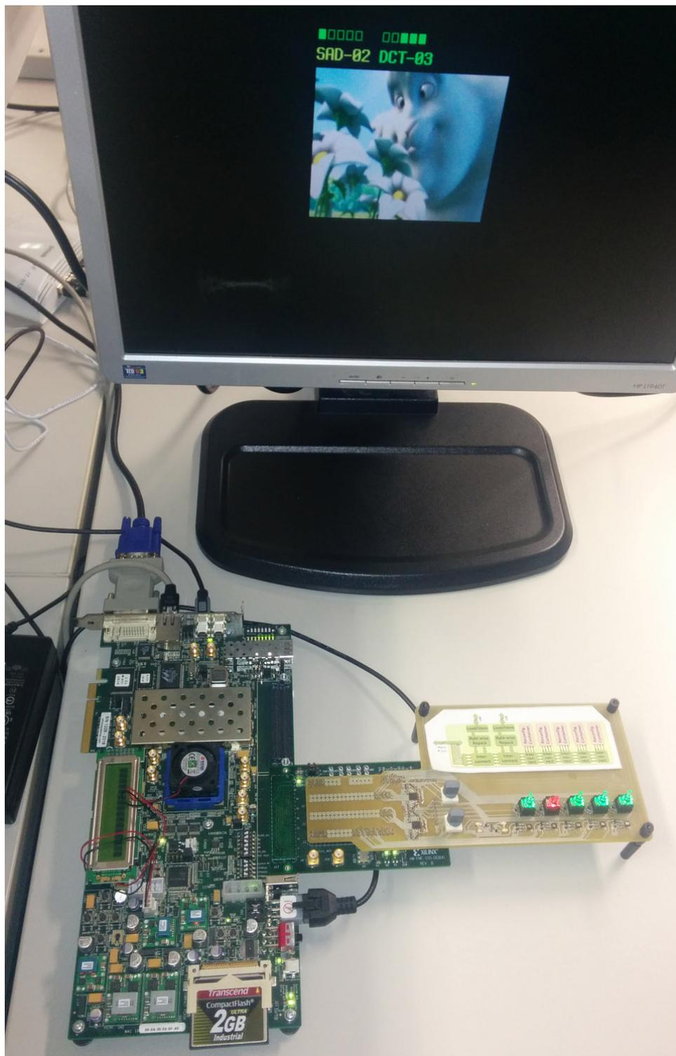
Figure 6.3: Demonstration setup of the *i*-Core as part of a small (2 tiles) Invasive Computing architecture configuration. The prototype is implemented on a Virtex-6 FPGA (ML605 board on the lower right) and is connected to a custom interface to allow interaction with each of the 5 RACs. The demo setup is running a modified H.264 Video Encoder.
