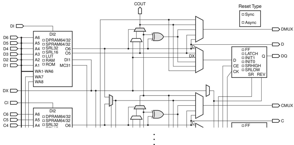
Figure 2.4: Excerpt from a SLICE (part of a CLB) diagram, which is used to implement logic on the fine-grained fabric of a Virtex-5 FPGA (from [Xil12]).
