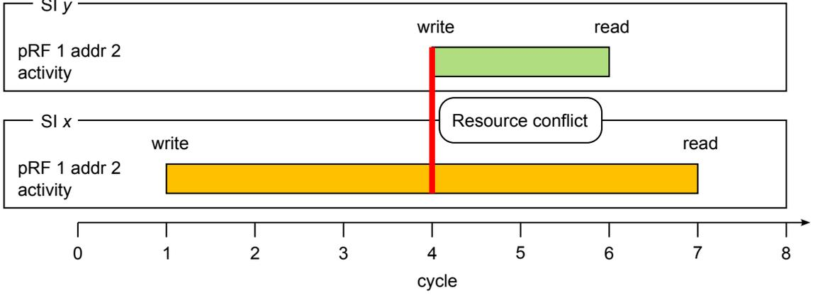
Figure 4.3: Resource conflict due to SIs  $x$  and  $y$  using the same private Register File (pRF) address.
