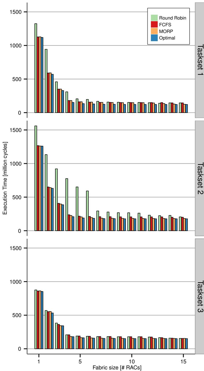
Figure 6.7: Makespan of 3 tasksets when scheduled by different schedulers.
