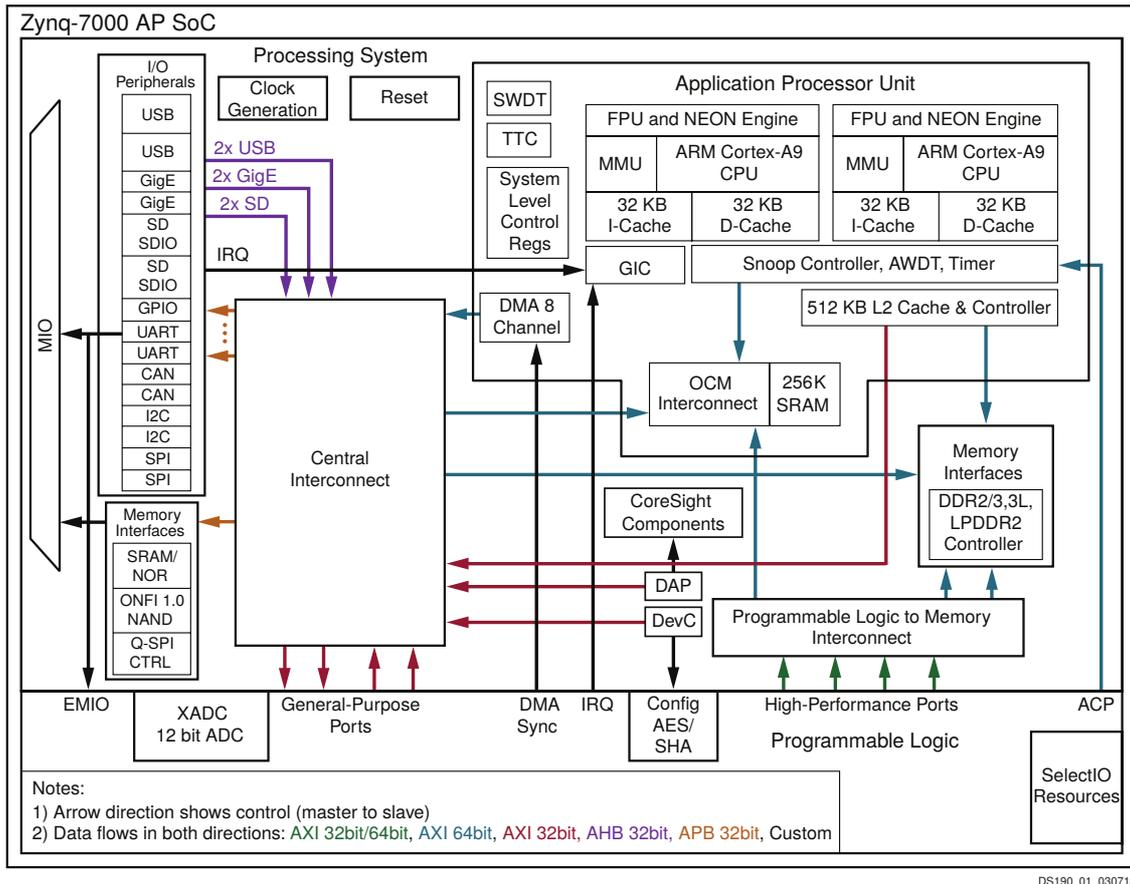
Figure 2.16: Zynq reconfigurable multi-core, consisting of an ARM Cortex-A9 dual-core (upper right) and a Xilinx Kintex reconfigurable fabric (bottom) (from [Xil]).
