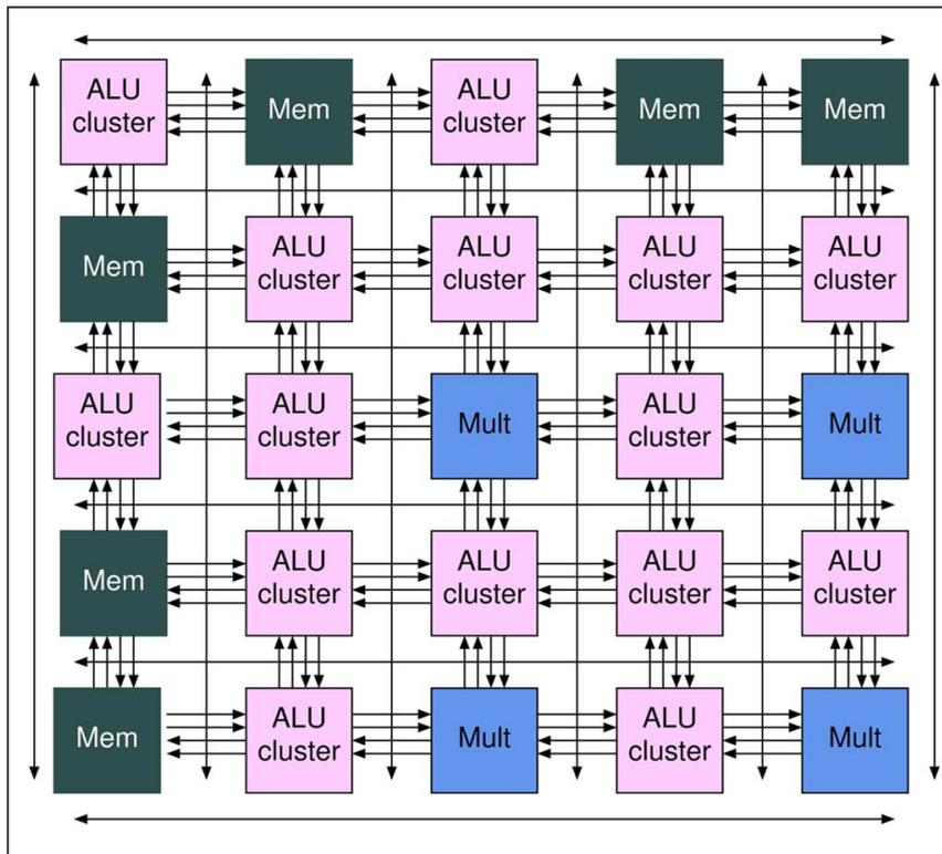
Figure 2.2: Example configuration of a EGRA heterogeneous coarse-grained architecture (from [ABP11]).
