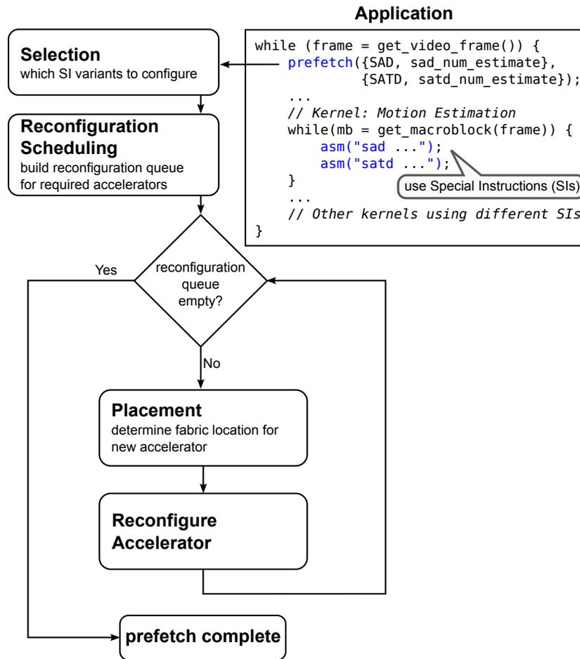
Figure 2.10: Prefetch of a kernel during execution of an application.
