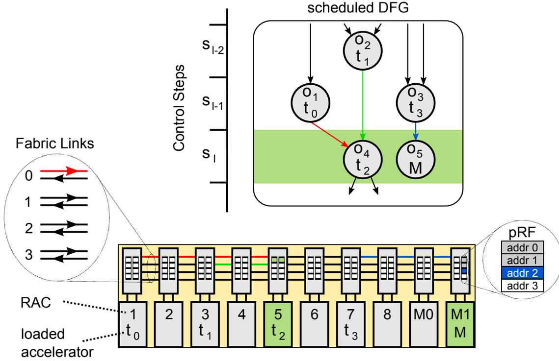
Figure 5.6: Binding of data transfers and intermediate results for control step  $s_l$  (highlighted light green) to fabric links and pRF addresses. Binding of operations to RACs has been performed already.
