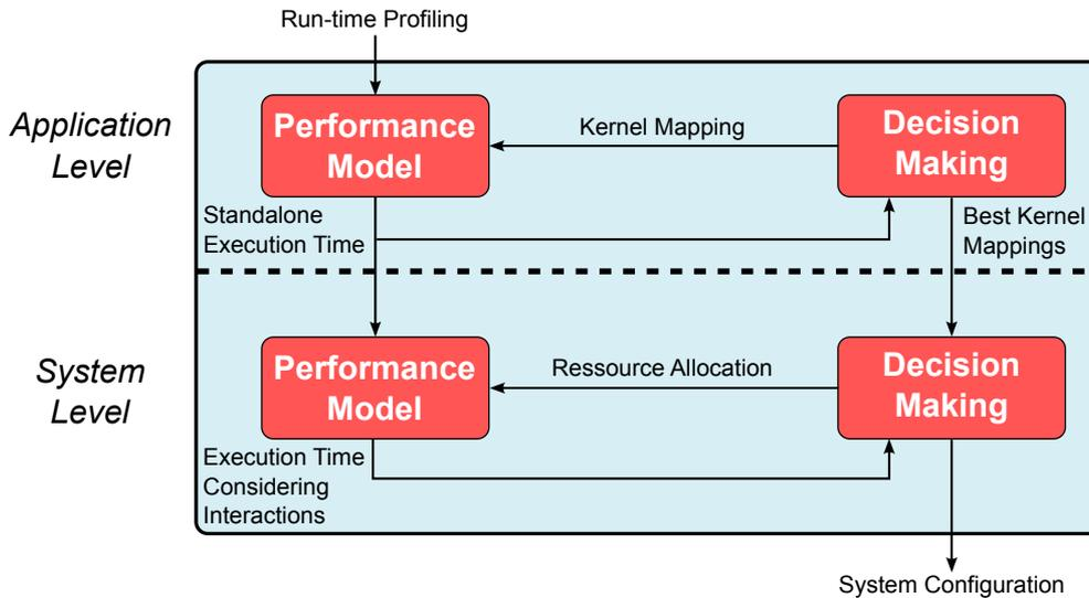
Figure 2.11: Two-layer run-time system for the MOLEN reconfigurable processor (from [MSPZ+13]).
