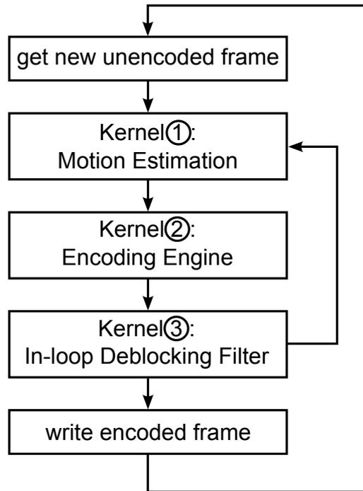
Figure 3.1: Flow of H.264 video encoder, showing its dynamic nature. 3 different kernels are continuously executed in sequence, resulting in a large amount
