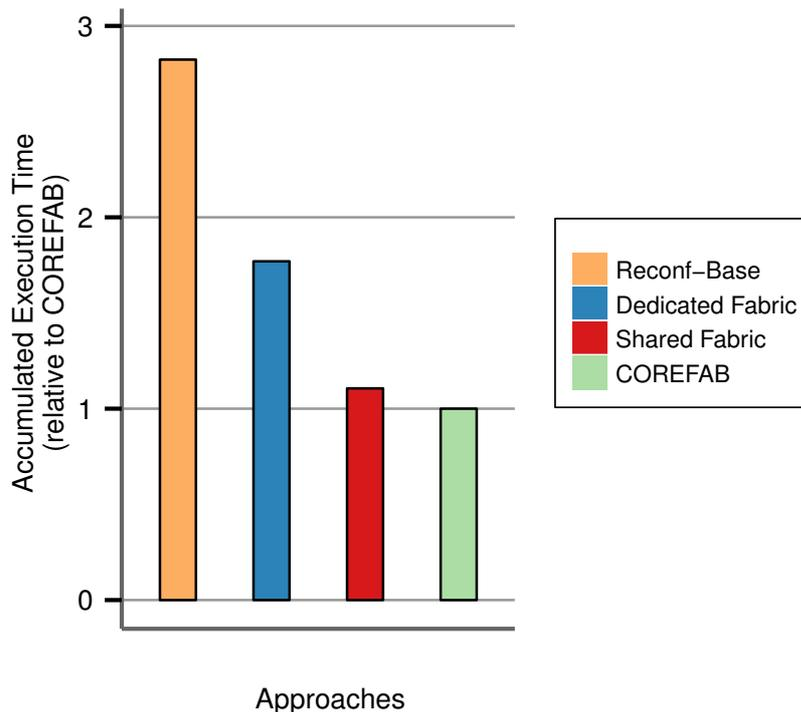
Figure 6.11: Accumulated execution time over all 4 cores (averaged over all workloads).
