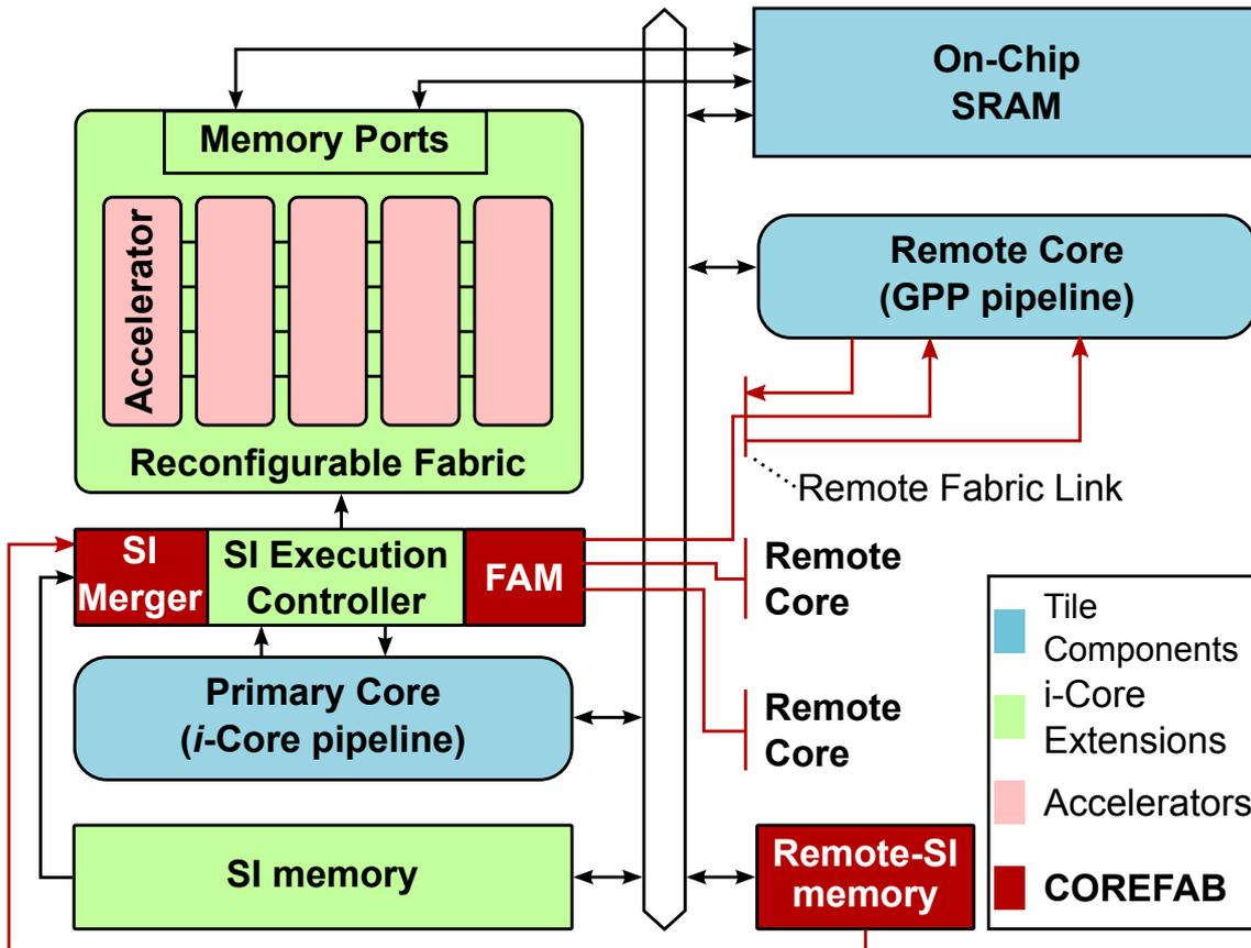
Figure 4.4: Multi-core architecture with shared reconfigurable fabric. COREFAB contributions are highlighted.
