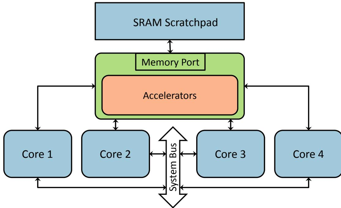
Figure 4.2: Multi-core architecture with one *shared fabric* between all cores.
