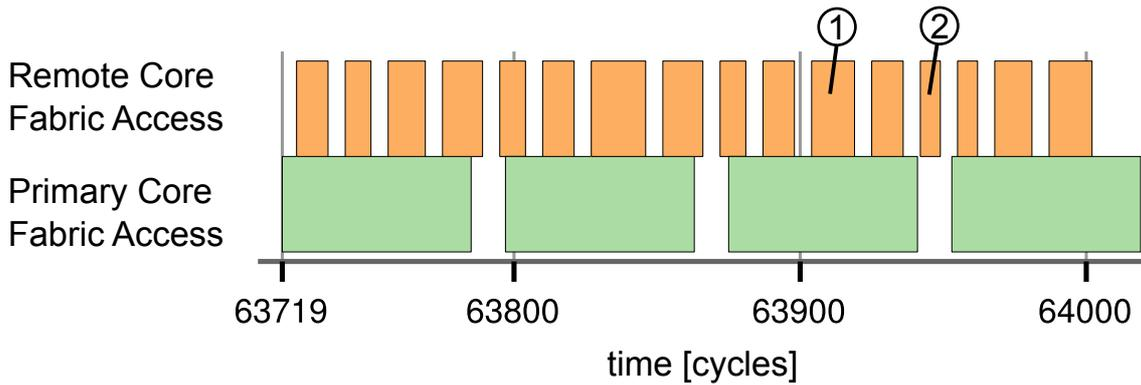
Figure 4.9: Trace of fabric accesses due to SIs from different cores.
