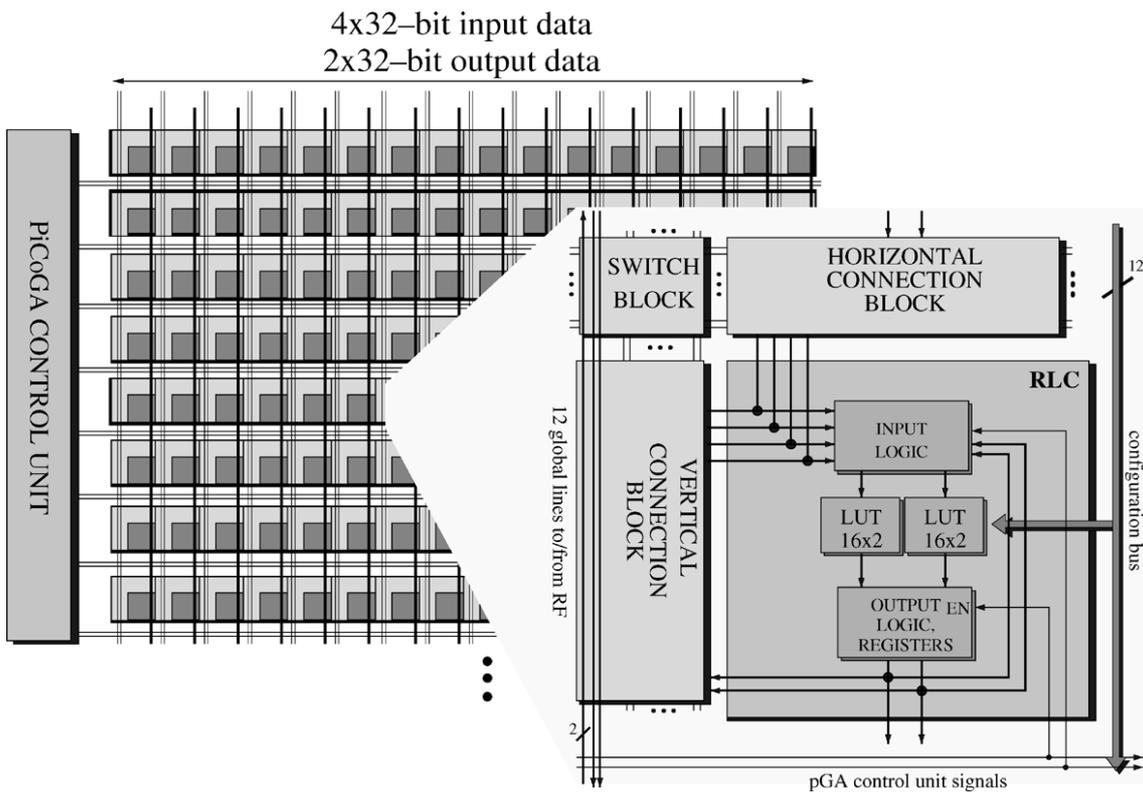
Figure 2.6: PiCoGa fine-grained fabric in the XiRisc processor (from [LCBM+06]). The XiSystem SoC [LCBM+06] adds the additional eFPGA fine-grained fabric.
