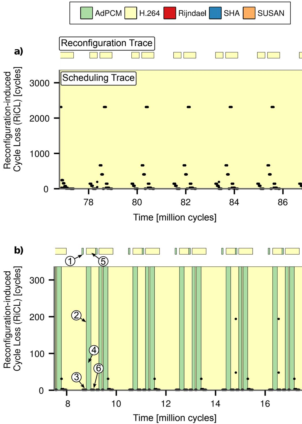
Figure 3.9: Scheduling and reconfiguration traces and RiCL of Taskset 2 using a) FCFS, and b) MORP scheduling. The range of the y-scale in a) is different than in b).
