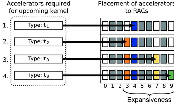
Figure 5.5: Example for placement of accelerators using Cluster Placement. Grey shaded RACs are in use and currently unavailable for placement. The expansiveness of the resulting SI variant is 6.
