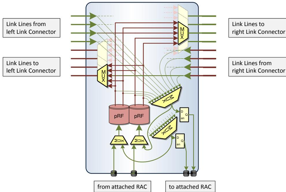
Figure 2.21: Link connector in the *i*-Core fabric, based on the RISPP Bus Connector (modified from [BH11]).
