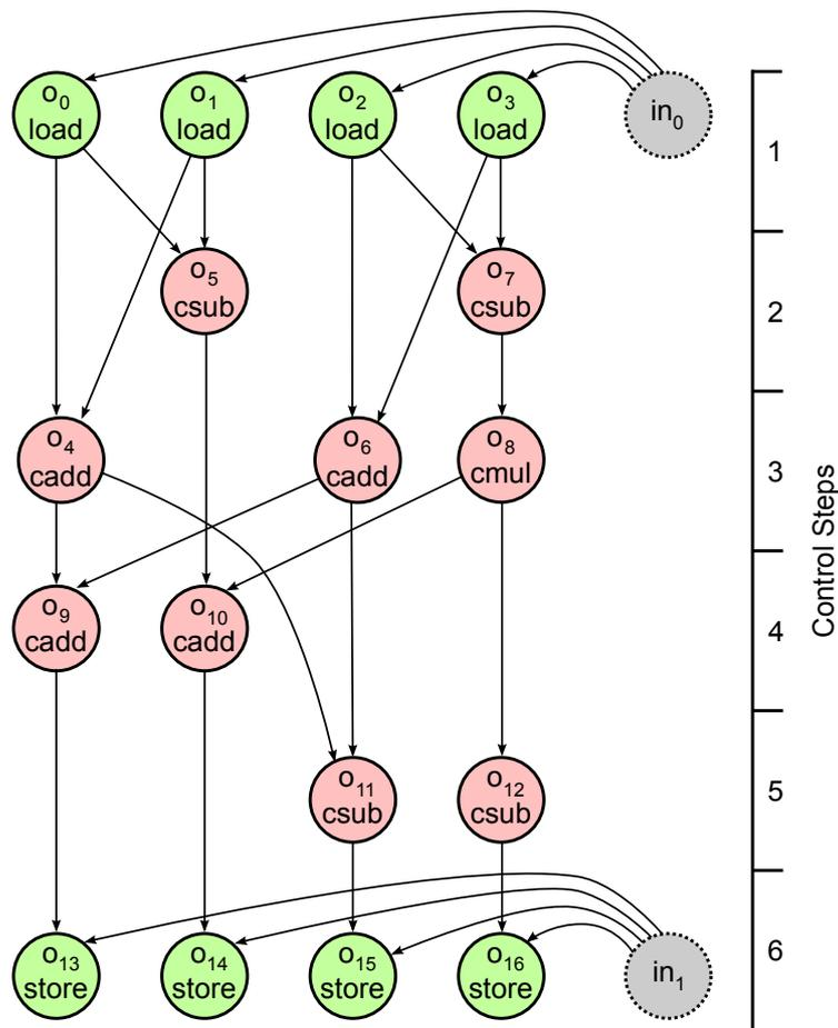
Figure 2.9: 4-input FFT SI scheduled under the resource constraint of 2 “cadd/csub” accelerators and 1 “cmul” accelerator. The resulting SI variant takes 6 control steps.
