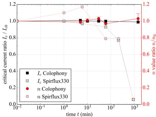
Figure 4.5: Critical current and  $n$ -value dependency of *REBCO* on colophony and Spirflux330®. Both reference values  $I_{c0}$  and  $n_0$  were measured for each tape before the flux treatment. Error bars indicate the standard uncertainty  $u$  for a sample size of 2. The solid lines are not physical, but serve as visual guide.
