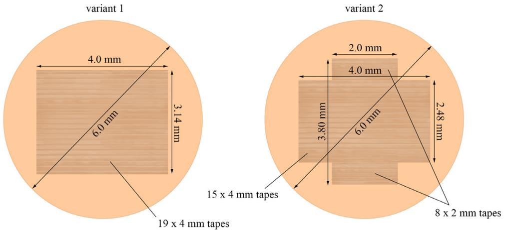
Figure 7.5: Comparison of both TSTC variants. The amount of conductor and the copper ratio is the same.
