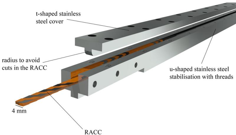
Figure 6.10: Stainless steel compaction for a 4 mm wide RACC cable. The pressure between the t-shaped cover and the u-shaped former is applied by stainless steel screws and induces a friction force of higher value than the expected Lorentz force inside the magnetic background field.
