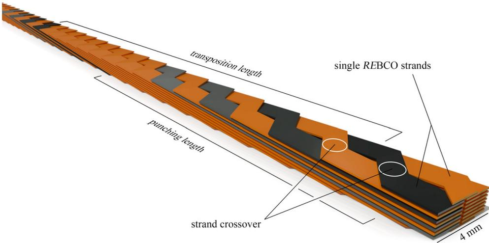
Figure 6.1: Schematic of a 16 strand RACC cable. The punched superconducting tapes were assembled to a Roebel composition. Over the length of two transpositions, each tape is visible once on the top and once on the bottom side. The transposition length is twice the punching length. Coloured strands help to guide the eye.
