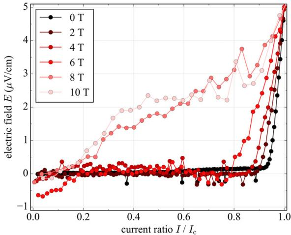
Figure 6.8: Measurement of a ten strand RACC cable at 20 K. The cable was mounted into the FBI facility with the superconductor  $c$ -axis parallel to the magnetic field lines. An increase of the magnetic field lead to irreversible cable damage. In order to compare the different functions of the electric field, the critical current was exceptionally estimated with a  $5 \mu\text{V}/\text{cm}$  criteria. Data from [Bar13].
