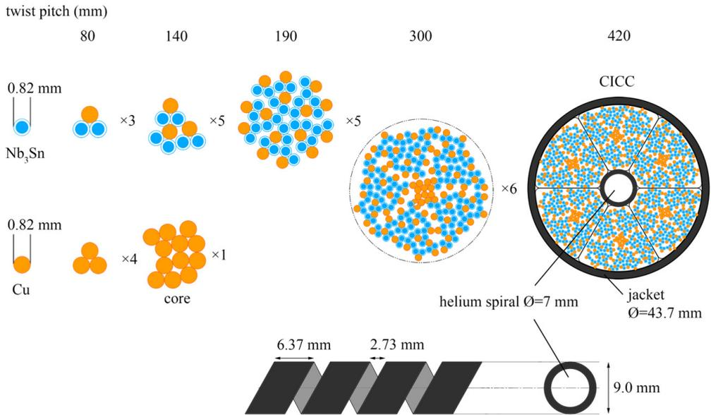
Figure 3.11: ITER Cable in Conduit Conductor (CICC). Twist pitch lengths from [BM08]. Picture after [ITE06].
