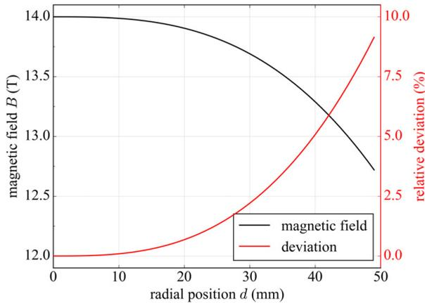
Figure 5.4: Magnetic field strength and relative deviation in the radial direction. The zero point represents the centre of the magnet. Fit function from [Oxf].
