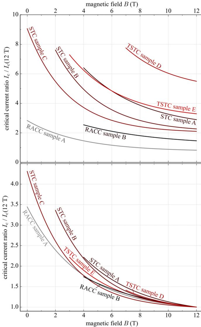
Figure 6.33: Comparison of the measured FBI samples at 4.2 K for different magnet background field values. All curves were obtained by fitting the FBI measurements with equation 6.3.
