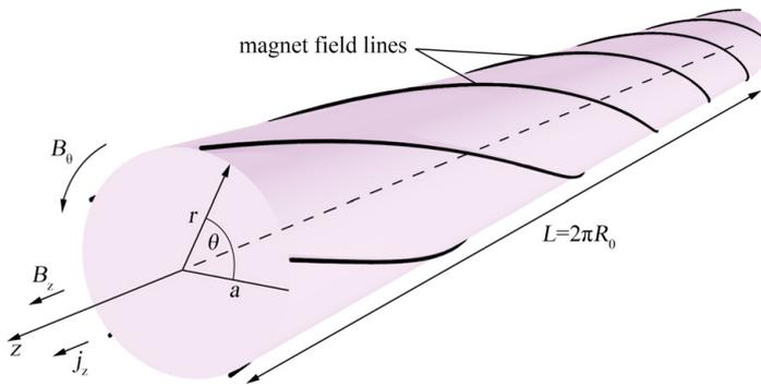
Figure 2.3: Helical magnetic confinement as superposition of the poloidal field  $B_\theta$  and the longitudinal field  $B_z$ .
