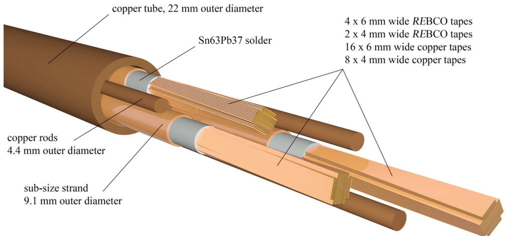
Figure 6.24: Schematic of the  $3 \times (4+4)$  full-size TSTC sample D. Three TSTC super-strands, which consist of 6 mm and 4 mm wide *REBCO* and copper tapes, are soldered in parallel orientation into a copper conduit. Additional copper rods prevent the super-strands from moving or bending inside the 12 T magnet background field.
