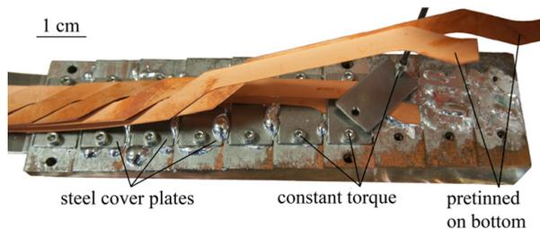
Figure 6.3: Solder joints for a 12 mm wide RACC. Each tape is soldered individually and afterwards fixed with stainless steel plates. Photo from [Bar13]
