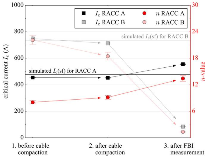
Figure 6.19: Critical current measurements at self-field of both RACC samples before and after the cables were compacted with the stainless steel former and after the FBI measurement. Horizontal lines mark the simulated critical current at self-field. The FEM simulation was executed in COMSOL.
