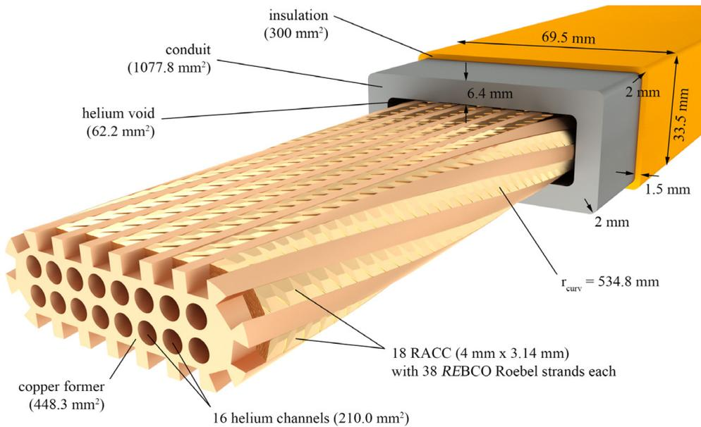
Figure 7.8: Schematic of a feasible DEMO full-size RACC cable.
