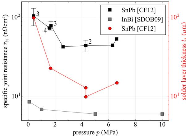
Figure 4.9: Specific joint resistance  $r_{js}$  and solder layer thickness  $t_s$ , depending on the applied pressure during soldering. The solder layer thickness was not measured for all tapes, but for random samples. Error bars indicate the standard uncertainty  $u$  and numbers the sample size. Data from [CF12, SDOB09].
