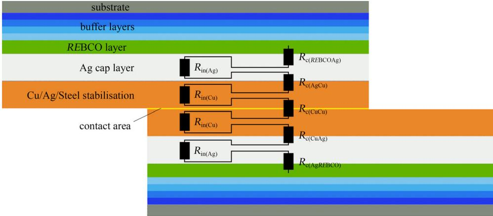
Figure 4.3: Intrinsic joint resistances  $R_{in}$  and contact resistances  $R_c$  for an HTS face-to-face lap joint.
