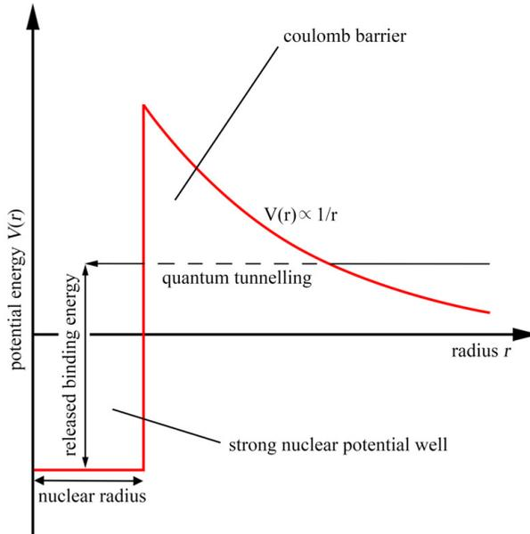
Figure 2.1: With increasing particle energy the probability for quantum tunnelling through the coulomb barrier increases. After penetrating the coulomb barrier, both nuclei are affected by the strong force and fuse to a larger nucleus. The difference between the binding energy of the separated and the combined nuclei is released.
