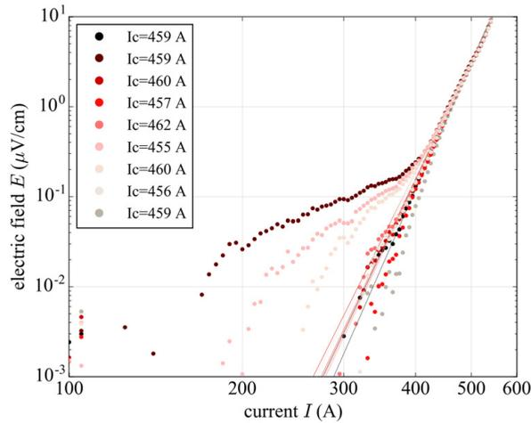
Figure 6.7: Homogeneous current distribution inside a RACC of ten strands. For each single tape, the voltage was measured separately. The current was taken from a shunt and therefore was measured for the overall cable. The power law was used to fit the data points. The electric field was calculated on basis of a  $1 \mu\text{V}$  criteria at the phase transition.
