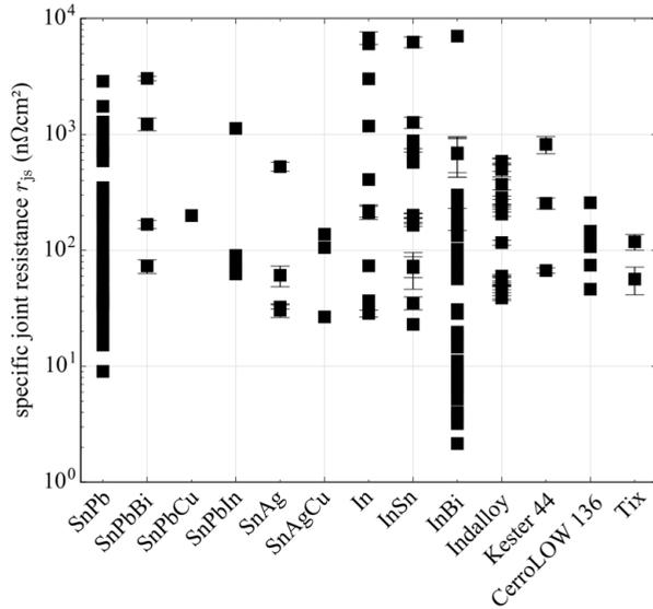
Figure 4.4: Specific joint resistances  $r_{js}$  of all collected publications on soft solder contacts between 2G high temperature superconductors, sorted by solder. Error bars indicate the standard uncertainty  $u$ . The source data of the plot can be found in table ?? in the annex A.1.
