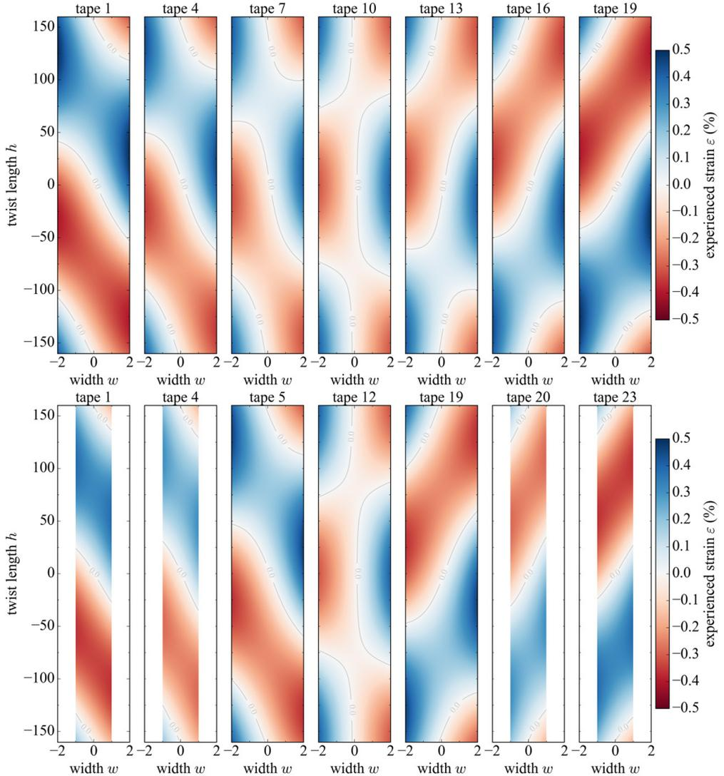
Figure 7.7: Strain calculation for variant 1 and variant 2 (top down) of the tapes inside the 18 twisted and bent REBCO stacks. For variant 1 the peak strain is 0.50% in tape 1 and tape 19. For variant 2 the peak strain is 0.47% in tape 5 and tape 19.
