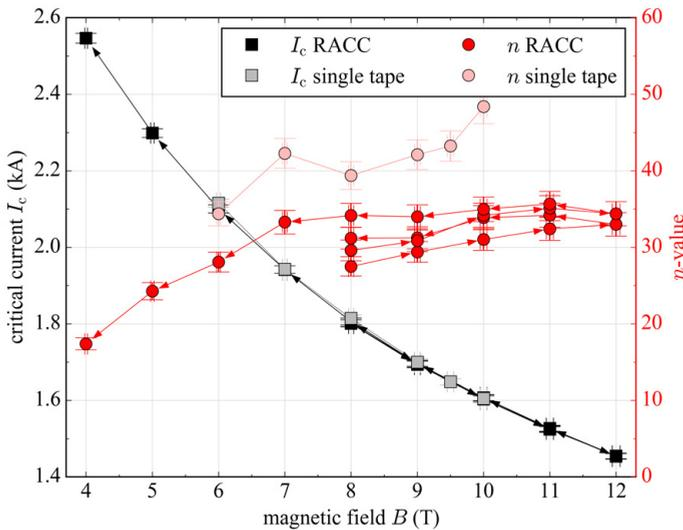
Figure 6.17: Performance of the 16 strand RACC sample B during measurement inside the magnetic background field of the FBI facility at 4.2 K. The magnetic field penetrates the sample parallel to the  $c$ -axis of the RACC. No degradation or training effect were observed. The  $I_c(B)$ -function of the RACC cable is perfectly in accordance with the single RACC tape measurement. Arrows illustrate the measurement sequence.
