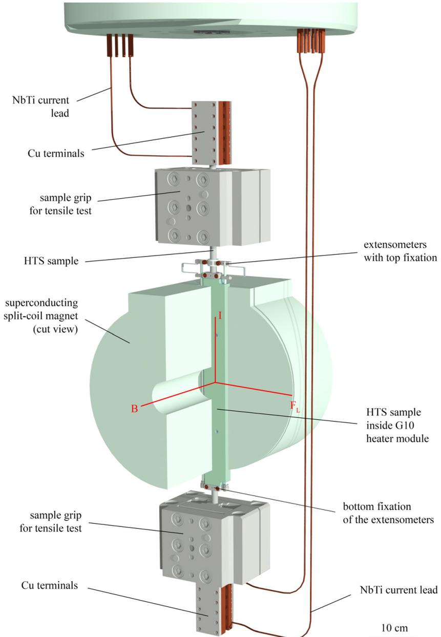
Figure 5.6: Schematic of the FBI-T sample section.
