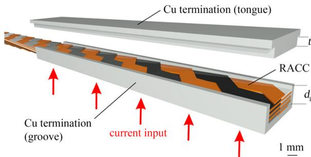
Figure 6.4: Copper termination for a 16 strand HTS RACC. The cable is soldered into the bottom copper groove, while the copper tongue serves to provide pressure during the solder phase. Coloured strands serve a better visualisation of the Roebel structure.
