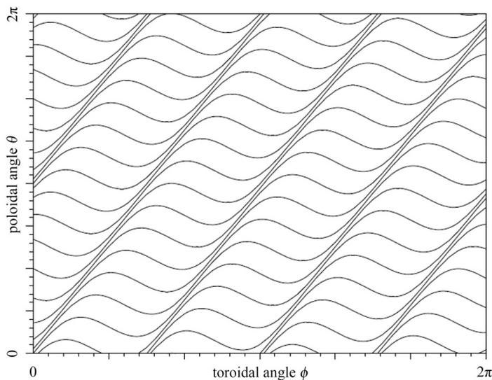
Figure 2.4: Multipole field of a stellarator. Picture from [WWZ10].
