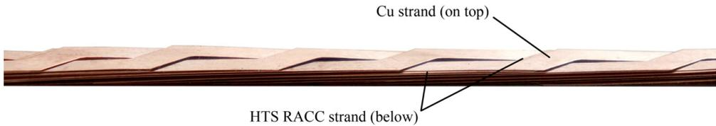
Figure 6.11: RACC sample 2 with 10 *REBCO* and 10 additional copper strands. Each copper strand covers the top side of one *REBCO* strand and serves as additional buffer layer against transversal pressure. Slight displacements between the copper and the superconducting strands are visible.
