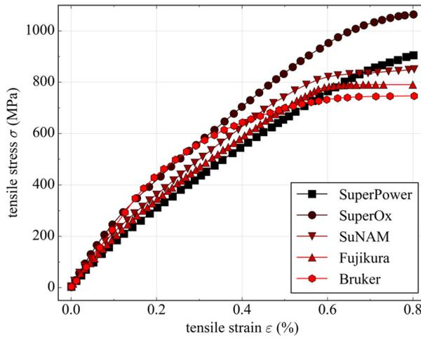
Figure 3.7: Tensile-stress-strain function for various commercial *REBCO* superconductor tapes at 4.2 K. Data from [BMS15].
