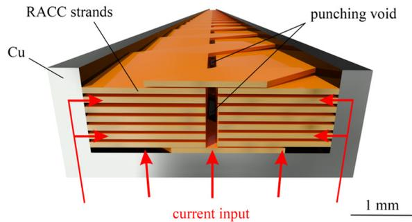
Figure 6.2: Schematic of a RACC cable inside a copper termination. The HTS tapes are oriented with the *REBCO* layer to the bottom side, to avoid the intrinsic resistance of the high ohmic stainless steel substrate. Voids between the tapes and the copper former are filled with soft solder.
