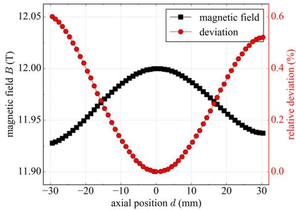
Figure 5.7: Magnetic field strength and relative deviation in the axial direction. The zero point represents the centre of the magnet. Data from [Oxf].
