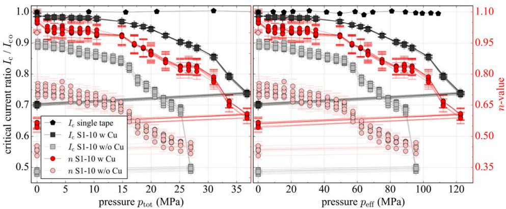
Figure 6.15: Comparison of sample 1, sample 2 and single tape data under transversal pressure at 77 K. The additional copper protects the RACC from degradation due to transversal pressure. Connecting lines serve to guide the eye. Data for the single tape from [TKO<sup>+</sup>07].
