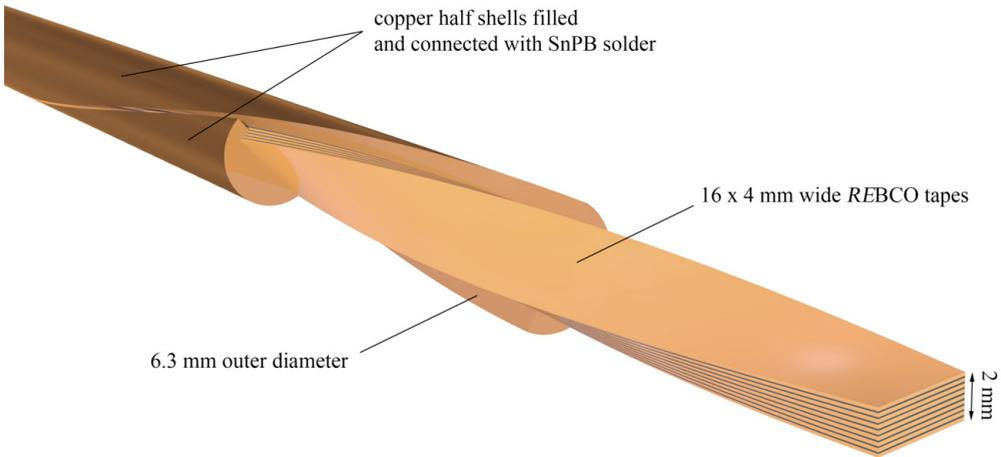
Figure 6.25: Schematic of the 16 tape TSTC sample E. The 4 mm wide superconductors are soldered into two copper half-shells and were afterwards precisely twisted. This sample is the super-strand model used for a 60 kA coated conductor cable prototype for fusion magnets, that was measured in the EDIPO facility.
