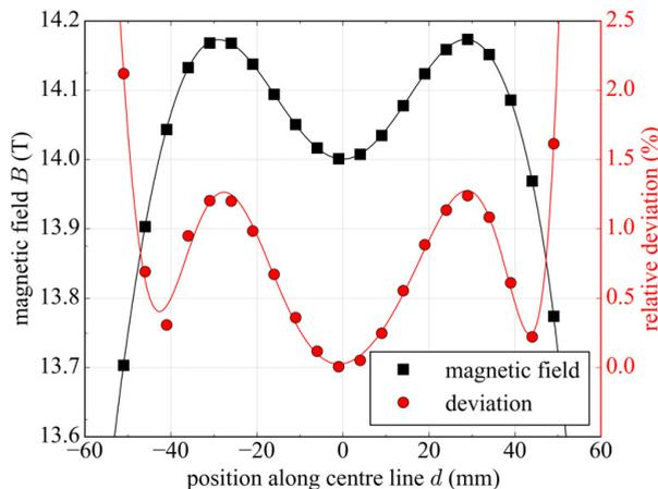
Figure 5.3: Magnetic field strength and relative deviation in the axial direction with polynomial fit function. The zero point represents the centre of the magnet. Data from [Oxf].
