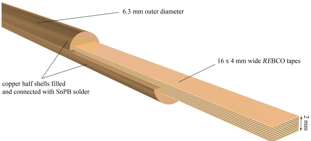
Figure 6.21: Schematic of the 16 tape stacked tape sample A inside its copper conduit which consists of two copper half-shells. The hole composition of tapes and copper half-shells is soldered together.
