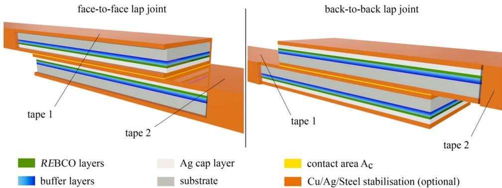
Figure 4.2: Cutaway drawing of a face-to-face and a back-to-back lap joint made of two HTS tapes.
