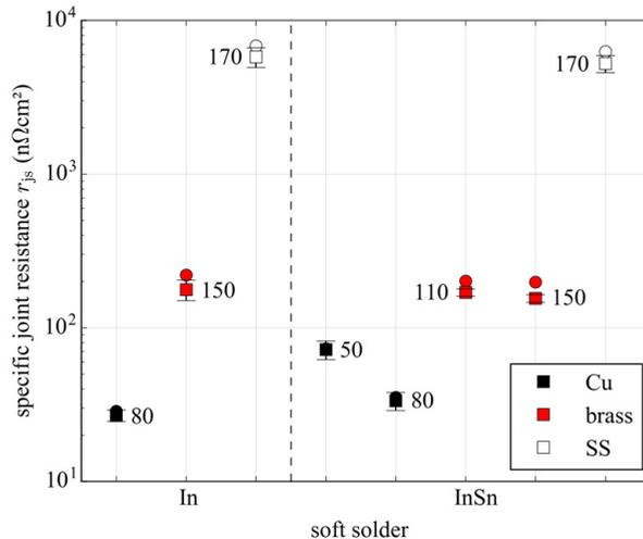
Figure 4.8: Specific joint resistance  $r_{js}$  for different electroplated metal stabilisations. Circles give the value before subtracting ohmic contributions due to the intrinsic resistance  $R_{in}$  of the stabilisation material. Squares give the corrected data including error bars which indicate the standard uncertainty  $u$ . Numbers give the stabilizer thickness in  $\mu\text{m}$ . The sample size is 6 for each data point. Data from [ZDHG11, DZG<sup>+</sup> 10].
