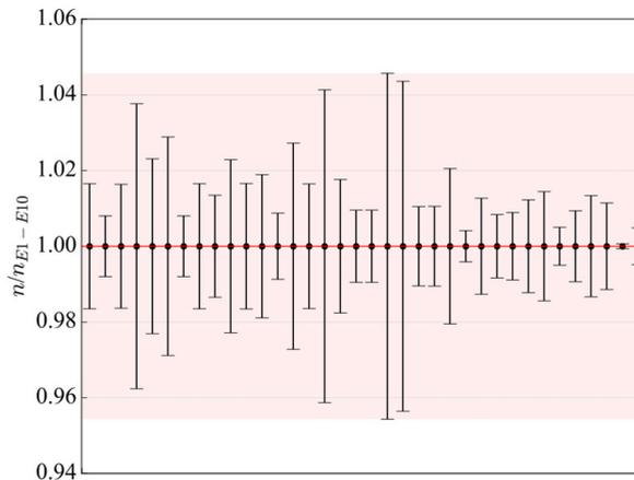
Figure 5.10:  $n$ -value calculations for 36 technical superconductor samples. The red line indicates the  $n_{E1-E10}$ -value. Error bars represent the average standard uncertainty due to the ten different considered intervals.
