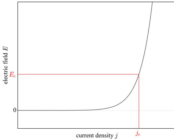
Figure 3.2: Schematic of a superconducting transition in a technical type II superconductor. The measured transition can be approximated for values close to the critical electric field  $E_c$  by the power law function.
