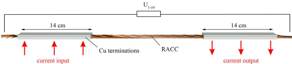
Figure 6.6: Four-terminal sensing of  $U(I)$  for a 10 strand 40 cm long RACC. Each tape of the RACC was measured individually. The voltage taps include the terminations. Coloured strands serve a better visualisation of the Roebel structure.
