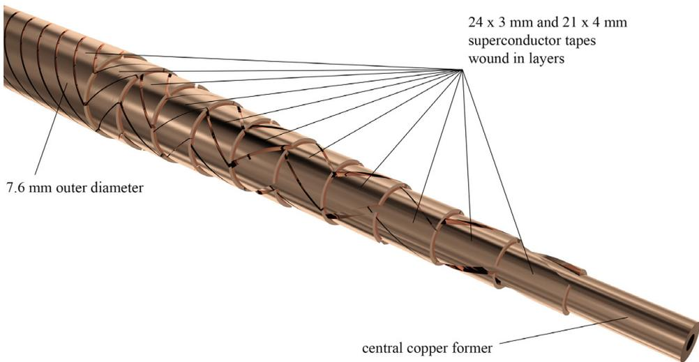
Figure 6.32: Schematic of the 24 tape CORC cable. The 4 mm wide superconductors are wound around a copper former and afterwards laminated with a thin foil.
