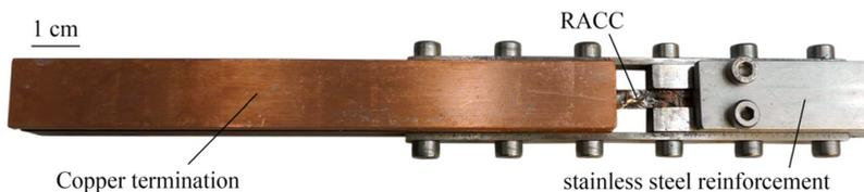
Figure 6.5: Finished termination for a RACC cable. The termination is oversized to allow for screws and threads which connect the termination to the stainless steel reinforcement for an in-field measurement. Inside toroidal field coil winding, the termination is supposed to be few millimetres wider than the cable width.
