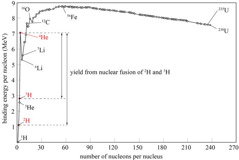
Figure 2.2: Binding energy depending on the number of nucleons. For iron and nickel the binding energy is maximal. Compared to any other hydrogen fusion reaction, the deuterium-tritium reaction is the reaction with the highest energy output and the lowest requirement to reach the Lawson criterion on earth.
