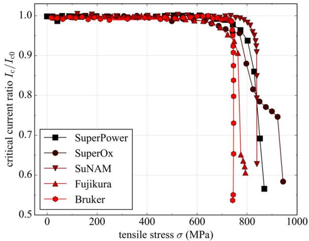
Figure 3.8: Current-tensile-strain function for various commercial *REBCO* superconductor tapes at 4.2 K inside a 19 T magnet background field. Data from [BMS15].
