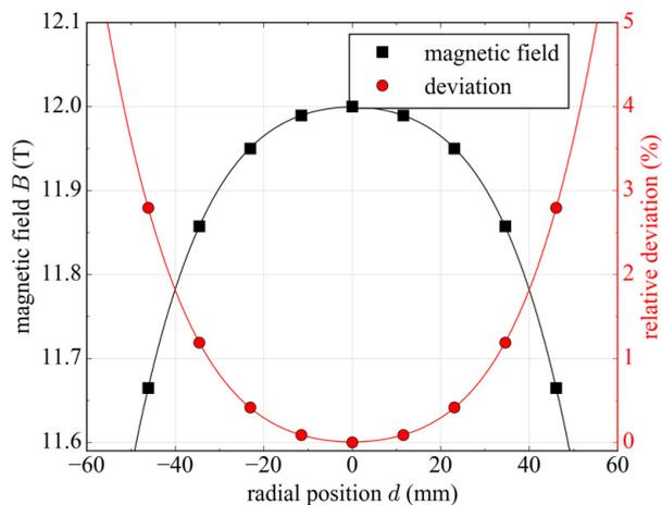
Figure 5.8: Magnetic field strength and relative deviation in the radial direction with polynomial fit function. The zero point represents the centre of the magnet. Data from [Oxf].
