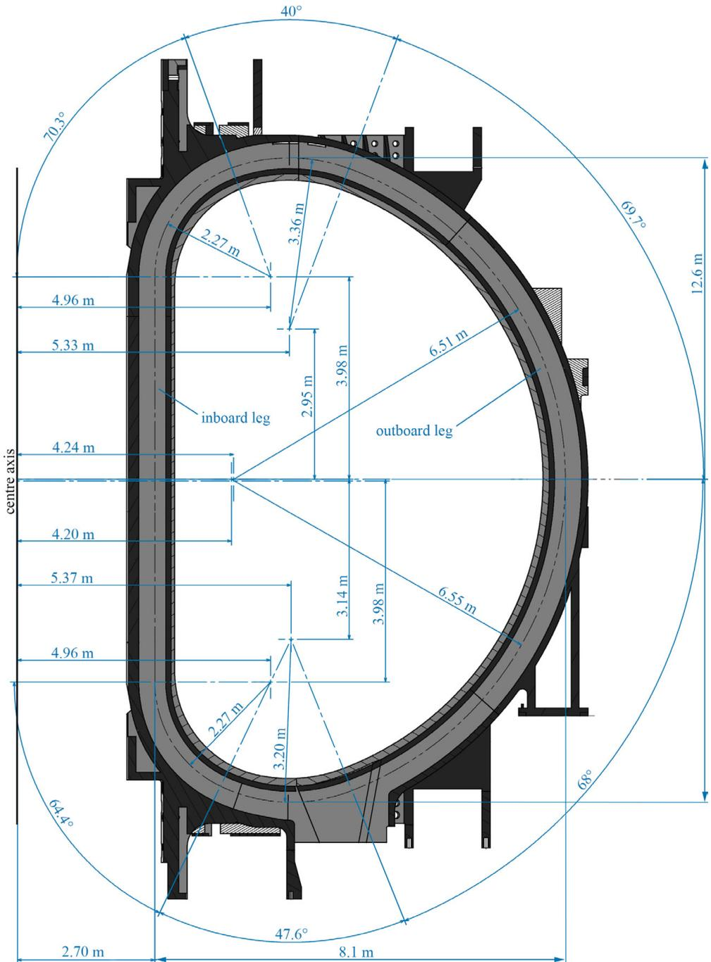
Figure 3.9: Dimensions of an ITER toroidal field coil. Picture after [ITE06].
