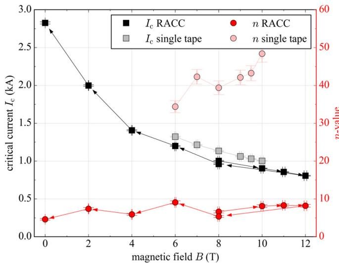
Figure 6.16: Performance of the ten strand RACC sample A during measurement inside the magnetic background field of the FBI facility at 4.2 K. The magnetic field penetrates the sample parallel to the  $c$ -axis of the RACC. A slight training during the first ramp to 12 T was observed. The difference between the critical current of the RACC and the up-scaled data of a single RACC tape is approximately 11%. Arrows illustrate the measurement sequence.
