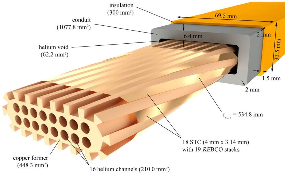
Figure 7.3: Schematic of a feasible DEMO full-size STC conductor.
