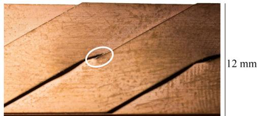
Figure 6.9: Measurement of a ten strand RACC cable at 20 K. The cable was mounted into the FBI facility with the superconductor  $c$ -axis parallel to the magnetic field lines. An increase of the magnetic field lead to irreversible cable damage. In order to compare the different functions of the electric field, the critical current was exceptionally estimated with a  $5 \mu\text{V}/\text{cm}$  criteria. Photo from [Bar13].
