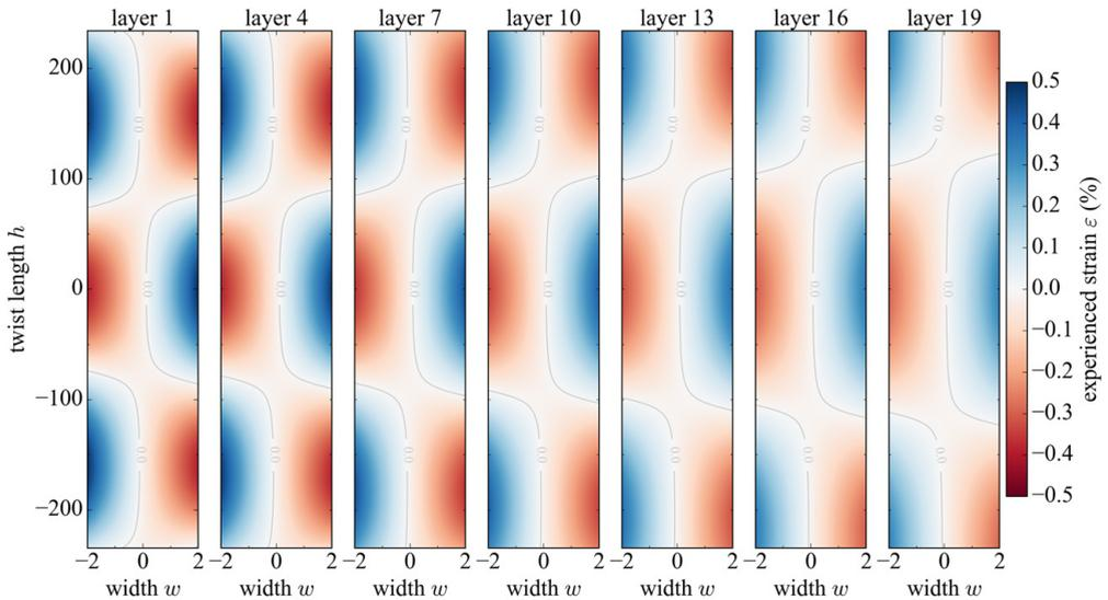
Figure 7.9: Strain calculation for seven of 19 layers inside the 18 twisted and bent RACC. The peak strain in the innermost layer 1 is 0.50%.
