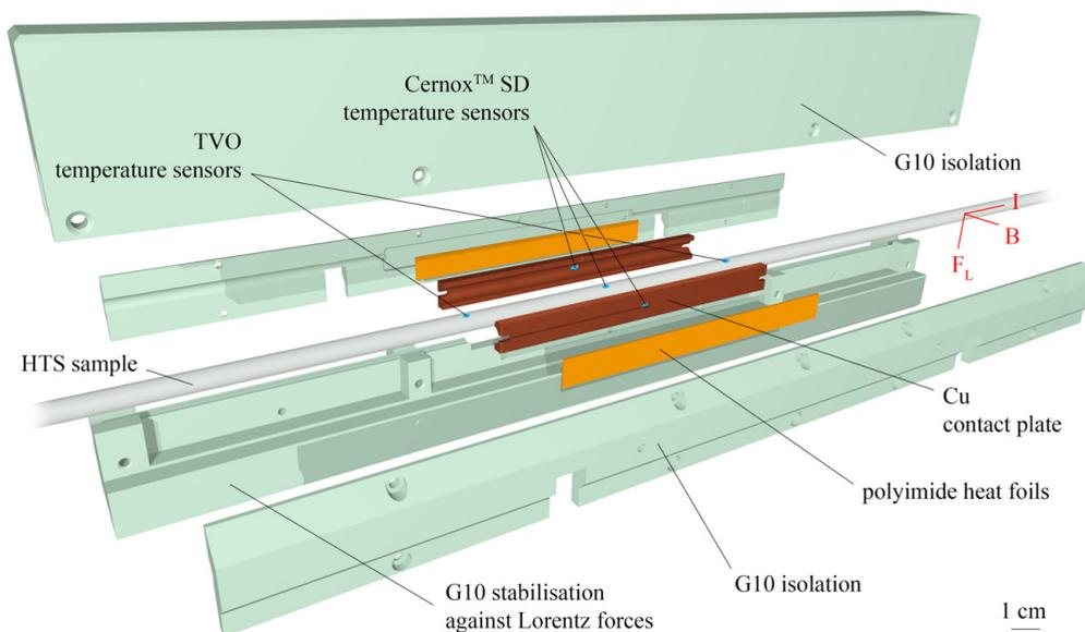
Figure 5.9: Exploded-view drawing of the G10 heater module.
