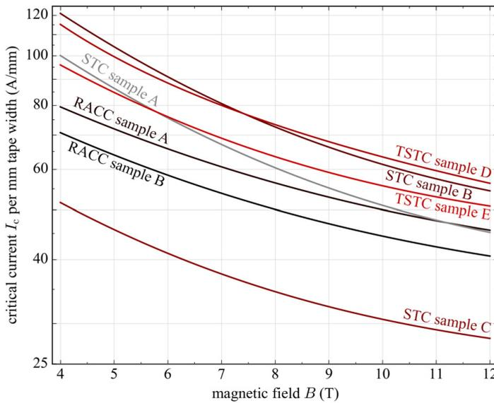
Figure 6.34: Comparison of the critical current per millimetre tape width for all measured sub-size cables at 4.2 K. All curves were obtained by fitting the FBI measurements using equation 6.3 and dividing the result by the number of tapes and the tape width.
