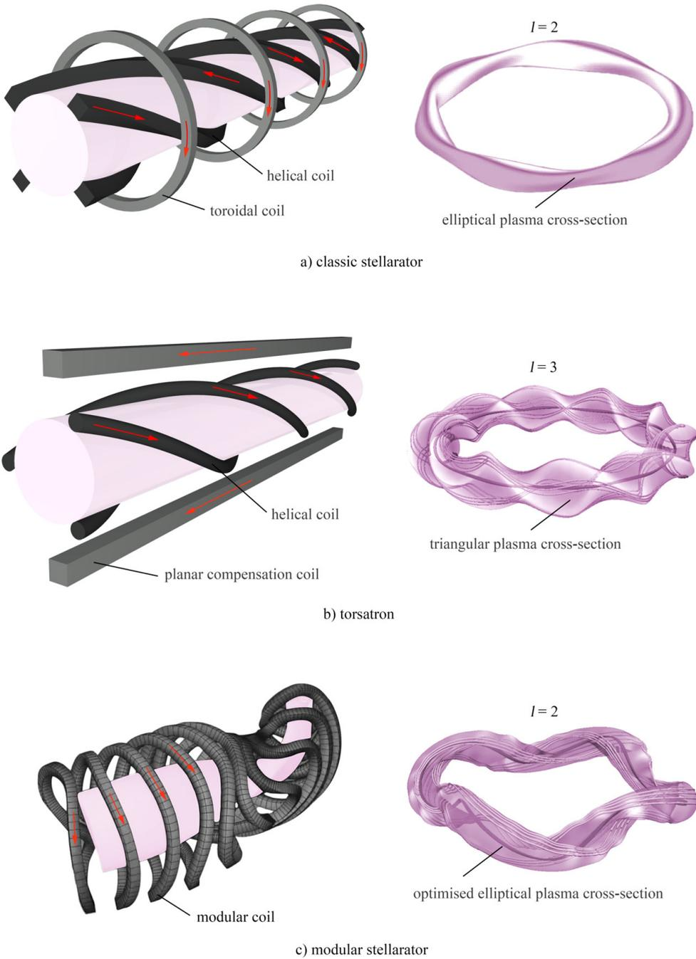
Figure 2.5: Magnet coils of the three different stellarator designs with the corresponding  $l$ -times folded magnetic field. Red arrows mark the current direction. Original plasma shape of the torsatron and the modular stellarator are taken from [Spo15].
