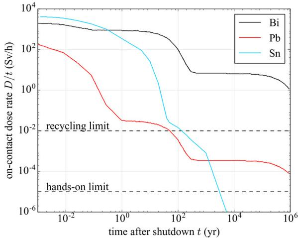
Figure 4.10: Time dependant decrease of the on-contact dose rates of constituent elements in soft solder joints after a nuclear activation of five years by ITER first wall dose (FWD). Data from [Sim16].
