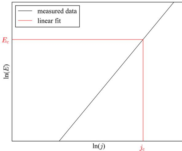
Figure 3.3: Schematic of a superconducting transition in a technical type II superconductor. Both, electric field  $E$  and the current density  $j$  are scaled logarithmically. The expected polynomial fit around the critical electric field  $E_c$  is of first order.
