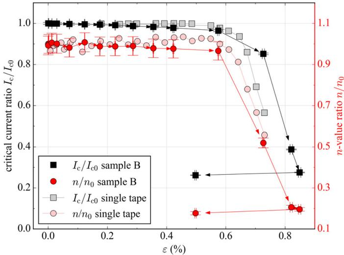
Figure 6.30: Critical current ratio and  $n$ -value ratio of sample B, depending on the longitudinal cable strain. The measurement was performed at 4.2 K inside a 12 T background field. Arrows show the measurement chronology. The single tape data is taken from [Bar15].
