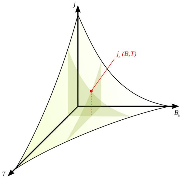
Figure 3.1: Schematic function  $j_c(B, T)$  depending on the magnetic irreversibility field  $B_{irr}$  and the conductor temperature  $T$  for a rare-earth-barium-copper-oxide (REBCO) superconductor.
