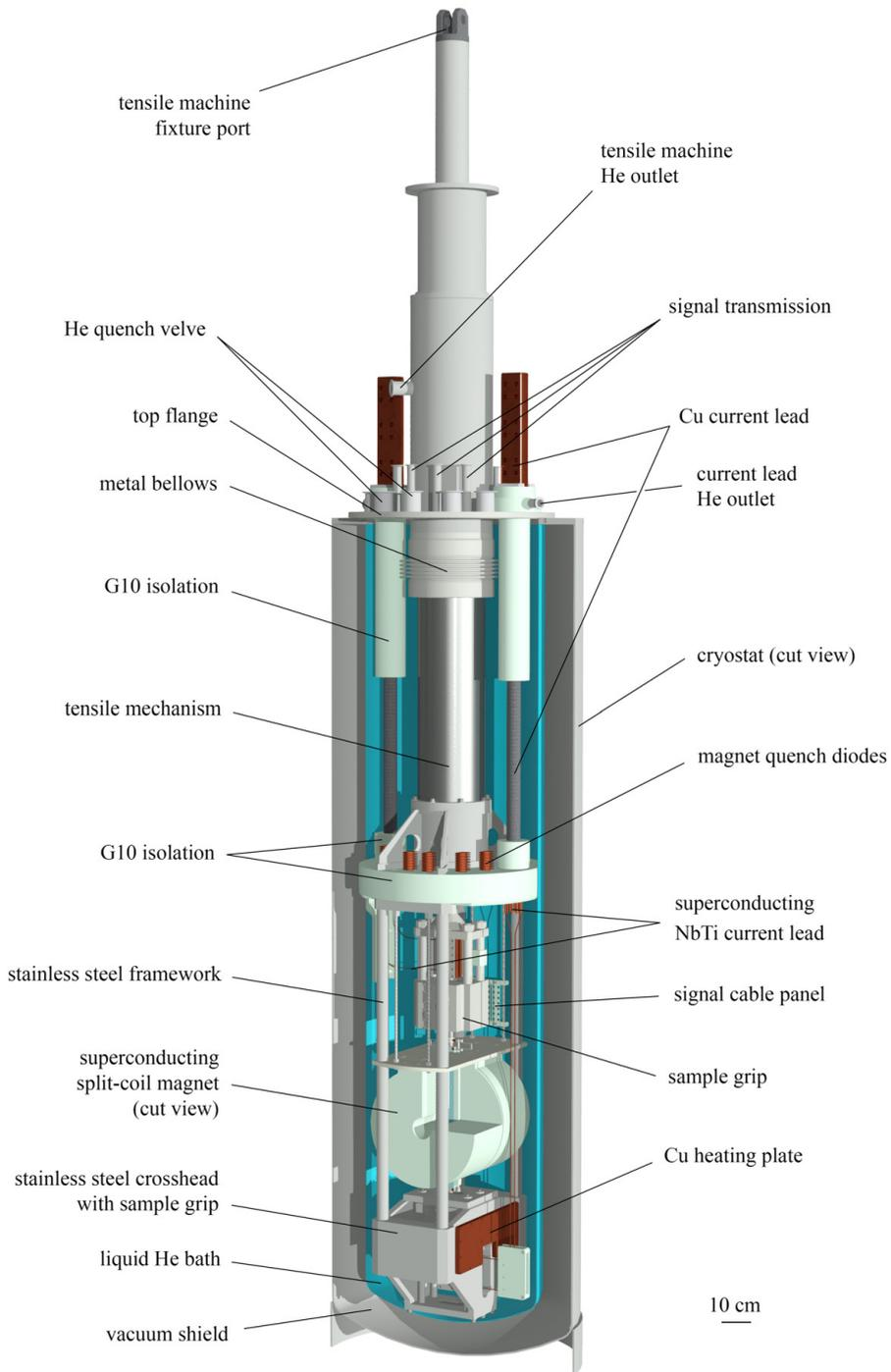
Figure 5.5: Cutaway view of the FBI-T measurement facility.
