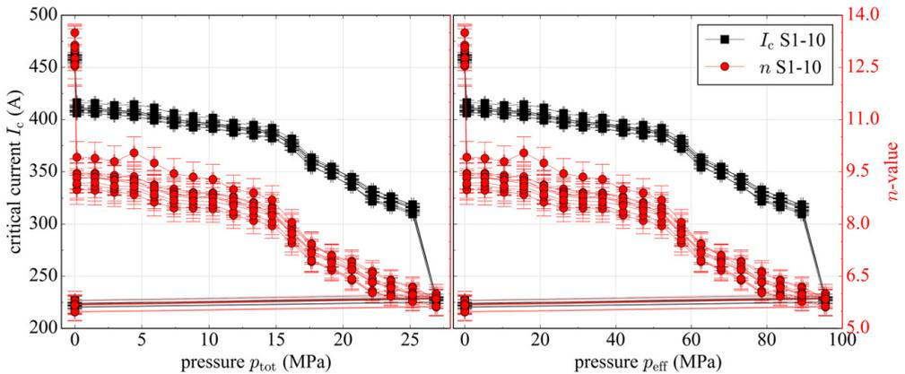
Figure 6.13: Performance of sample 1 at 77 K in liquid nitrogen depending on the total pressure  $p_{\text{tot}}$  and the effective pressure  $p_{\text{eff}}$ . The cable immediately degrades by 11% after applying slight transversal pressure. The second significant drop is reached for  $p_{\text{eff}} > 90$  MPa. The cable damage is irreversible. Connecting lines serve to guide the eye.
