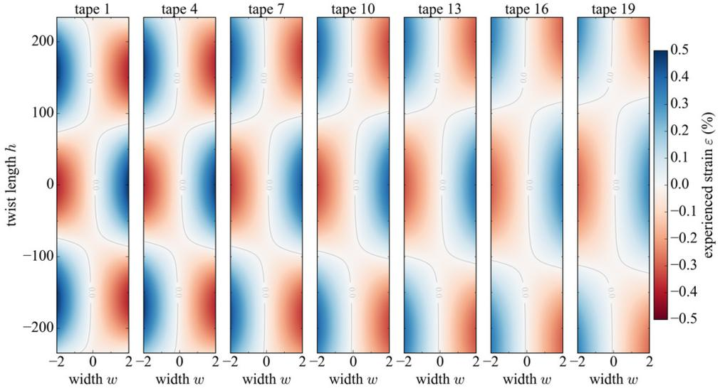
Figure 7.4: Strain calculation for seven of 19 tapes inside the 18 twisted and bent REBCO stacks. The peak strain in the innermost tape 1 is 0.5%.
