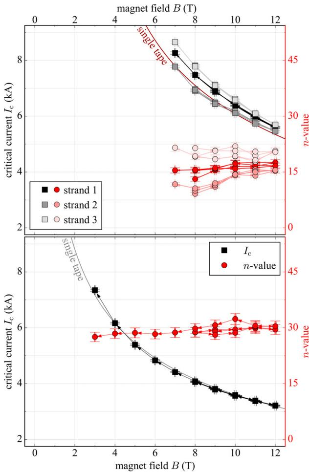
Figure 6.28: In-field performance of sample D and E (top down) at 4.2 K.
