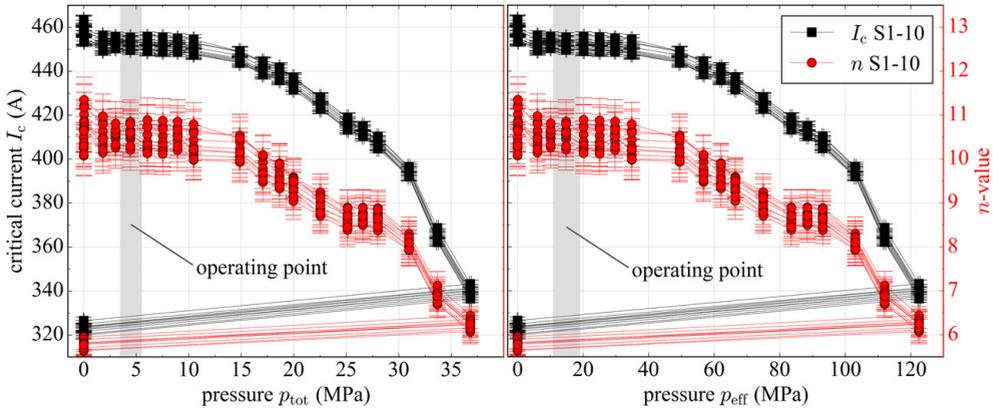
Figure 6.14: Performance of sample 2 at 77 K in liquid nitrogen depending on the total pressure  $p_{tot}$  and the effective pressure  $p_{eff}$ . The cable damage after the measurement is irreversible. Connecting lines serve to guide the eye.
