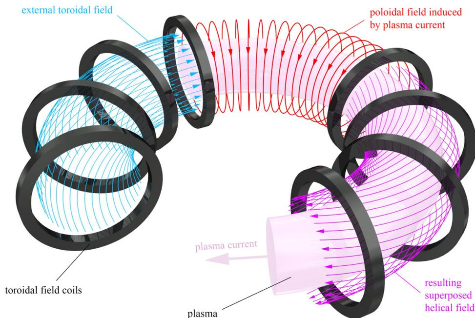
Figure 2.7: Magnetic plasma confinement of a tokamak. The helically wound, magnetic torus yields from superposition of toroidal and poloidal magnetic fields.
