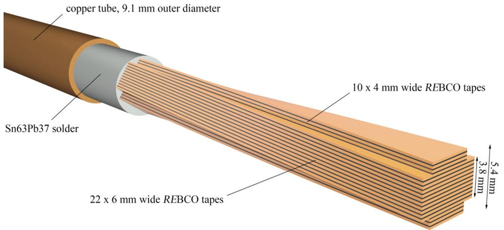
Figure 6.26: Schematic of the 32 tape TSTC sample F. The 4 mm and 6 mm wide superconductors are stacked, wound with solder wire, compacted inside a copper tube and afterwards twisted around its longitudinal axis.
