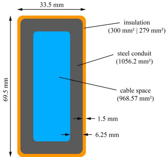
Figure 3.14: Dimensions of the DEMO cable conduits.
