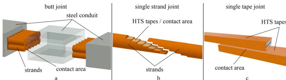
Figure 4.1: Schematic of a cable butt joint, a single strand joint and a single tape joint.
