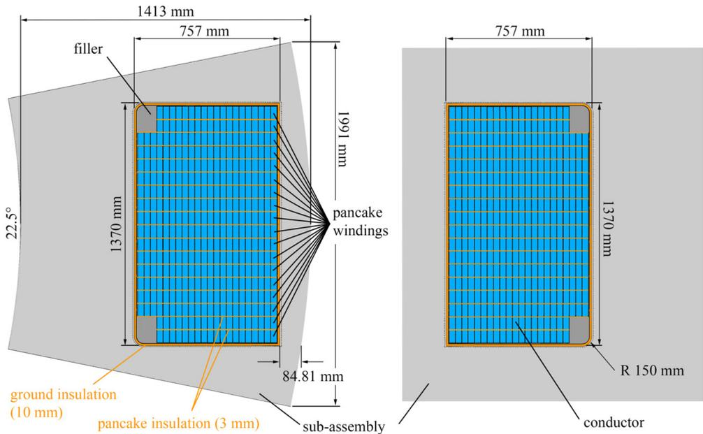
Figure 3.13: DEMO winding pack for inboard (left) and outboard leg (right).
