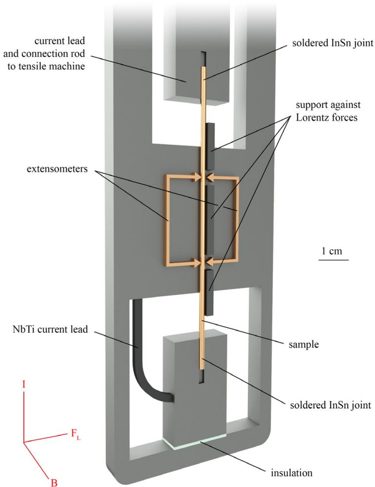
Figure 5.2: Schematic of the FBI sample holder. Picture from [Sch15].
