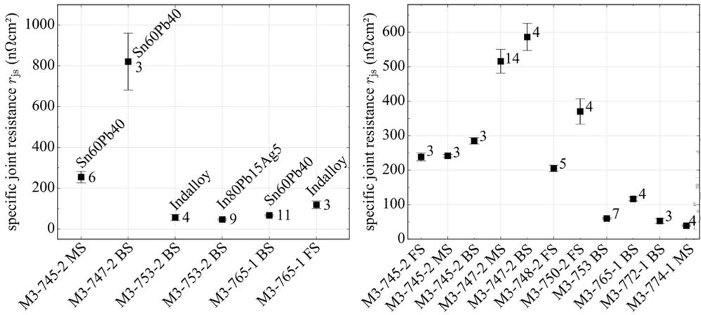
Figure 4.7: The production batch is highly influencing the specific joint resistance  $r_j$  for both, pre-tinned and non-pre-tinned solder joints. Although the same soldering procedure is performed for all measurements, the results deviate for different spool IDs. Error bars indicate the standard uncertainty  $u$  and numbers the sample size. Data from [KBL<sup>+</sup>13].
