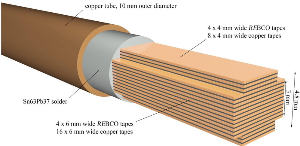
Figure 6.22: Schematic of the 4+4 tape stacked tape sample B inside its copper conduit which consists of a solder-filled copper tube. The cross design increases the ratio of superconductor to electro-mechanical stabilisation.
