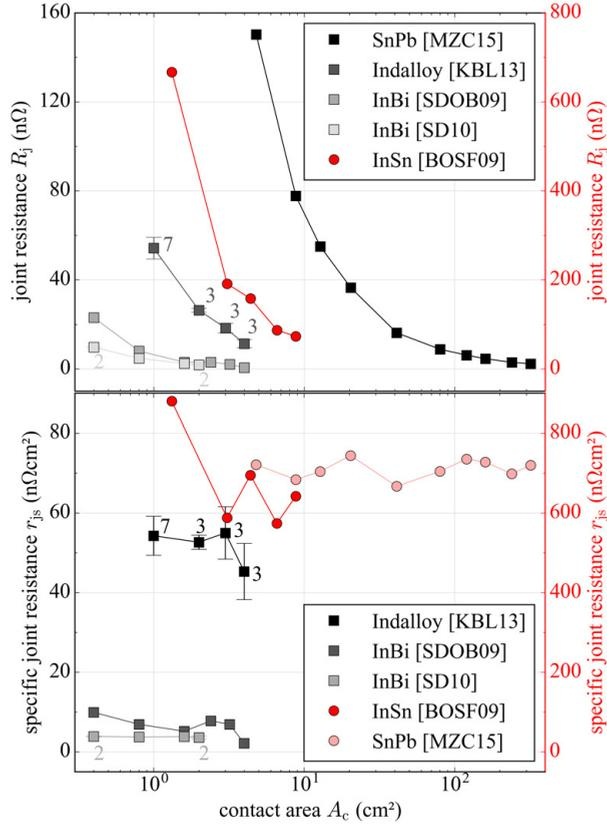
Figure 4.6: Joint resistance  $R_j$  and specific joint resistance  $r_{js}$  over the contact area  $A_c$  per meter conductor length. While the joint resistance decreases with a  $\frac{1}{A_c}$  proportionality, the specific joint resistance remains constant. The sample size is given by numbers. Solid lines are not physical, but indicate the physical trend. Error bars indicate the standard uncertainty  $u$  and numbers the sample size.
