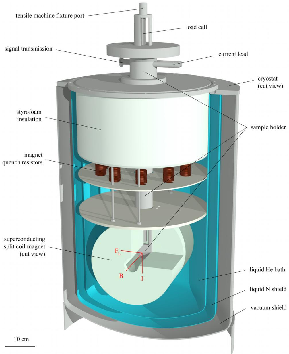
Figure 5.1: Cutaway view of the FBI measurement facility.
