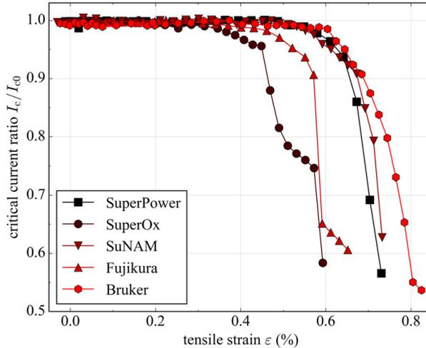
Figure 3.6: Current-tensile-strain function for various commercial REBCO superconductor tapes at 4.2 K inside a 19 T magnet background field. Data from [BMS15].
