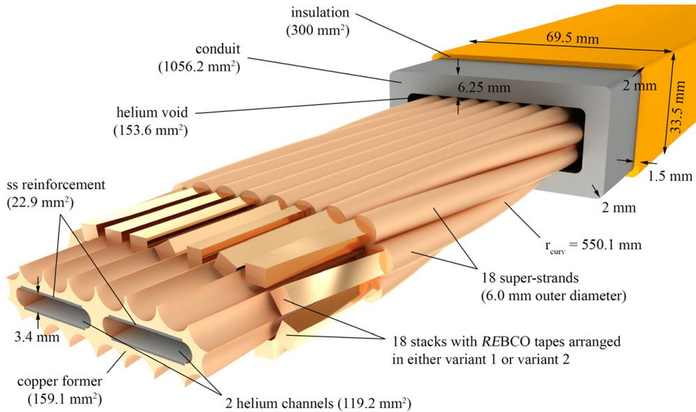
Figure 7.6: Schematic of a feasible DEMO full-size TSTC conductor.
