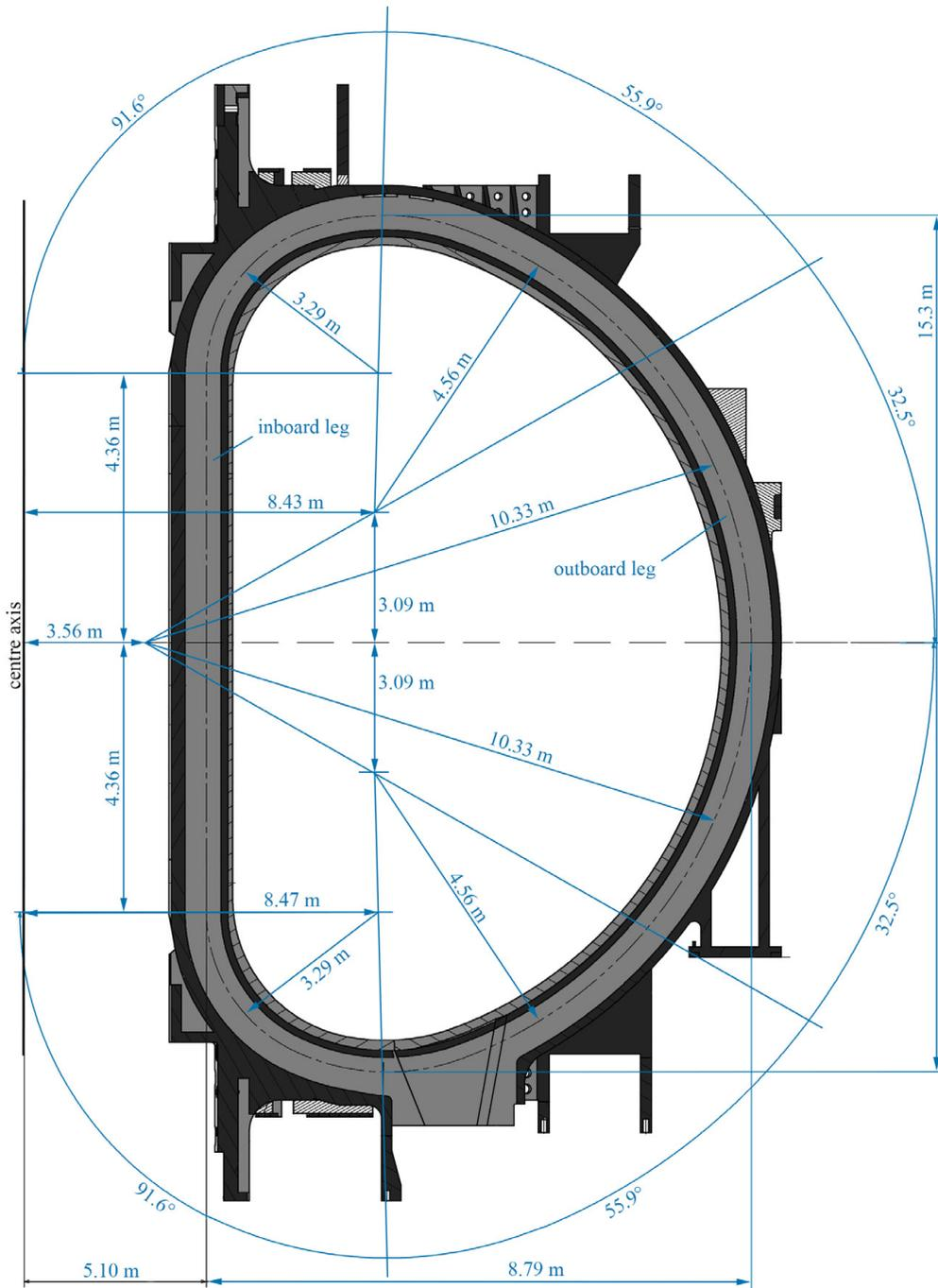
Figure 3.12: Dimensions of the DEMO toroidal field coil according to the adjusted DEMO July 2012 design [GBB<sup>+</sup>14, Gad16]. Although the dimension are correctly denominated, the drawing is not true to scale.
