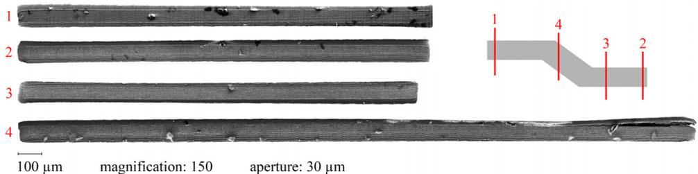
Figure 6.20: Scanning electron microscope (SEM) view of four RACC tapes taken from sample B. All of the 16 strands were cut by laser and checked for delamination effects. Four random represents from different tape sections are illustrated above. Figure from [BGB<sup>+</sup>16]
