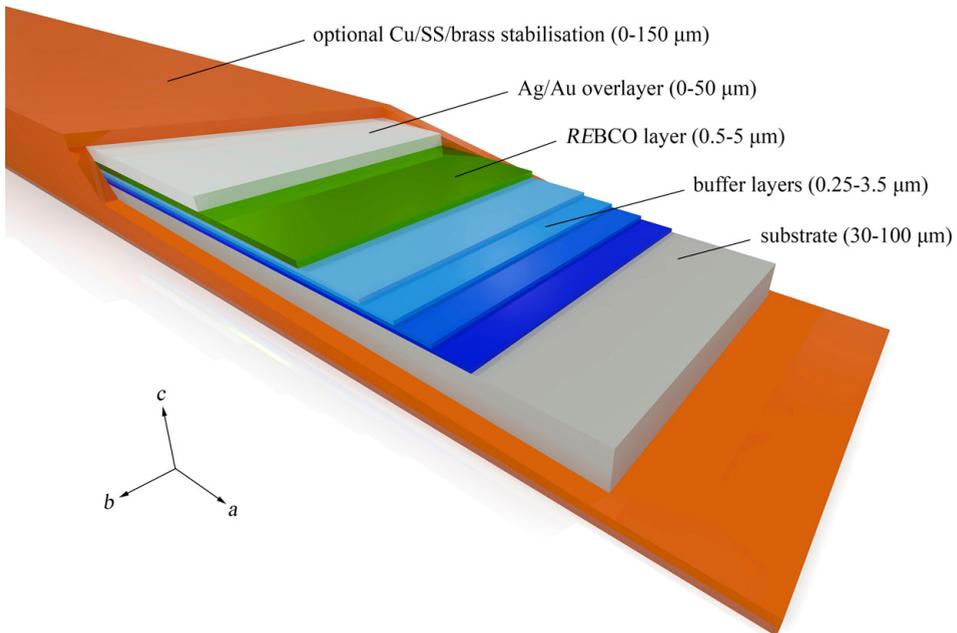
Figure 3.5: Tape structure of a REBCO coated conductor.
