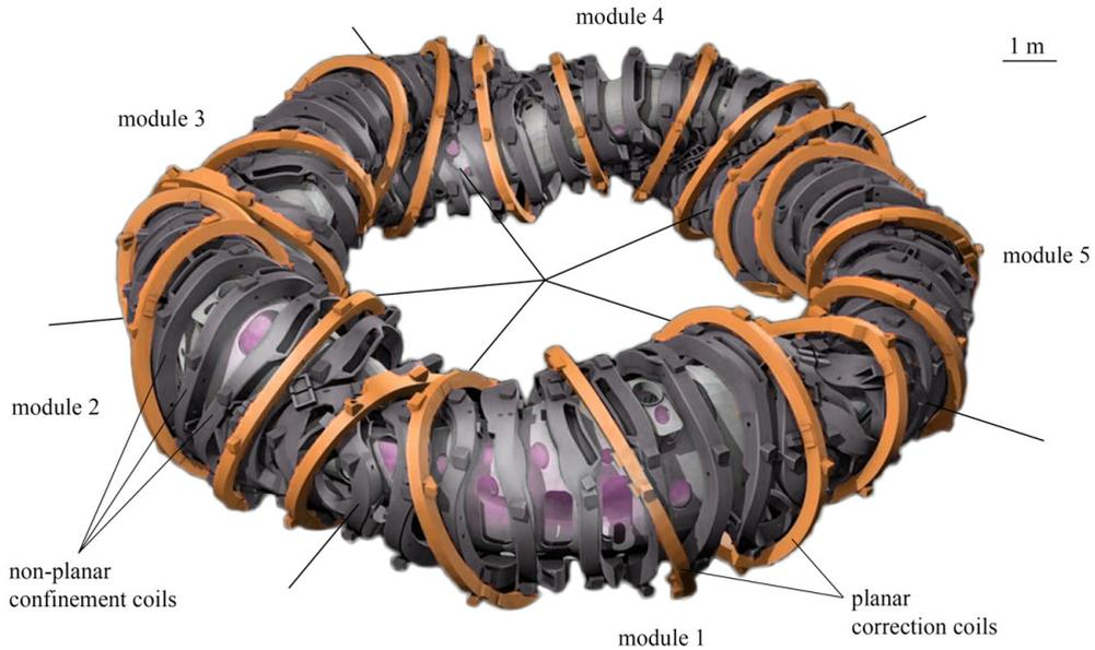
Figure 2.6: Modular magnet structure of Wendelstein 7-X with 50 non-planar confinement- and 20 planar correction coils. Original picture from [Bra].
