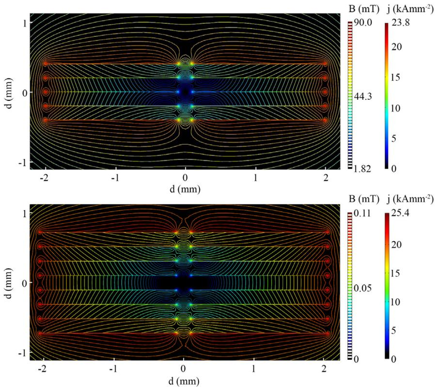
Figure 6.18: Finite element simulation of the magnetic self-field and the current density of the 10 strand RACC sample A and the 16 strand RACC sample B at 77 K. Figure from [BGB<sup>+</sup> 16]
