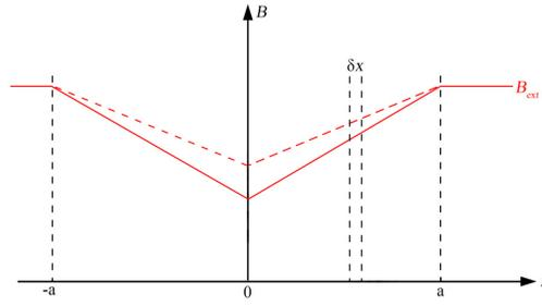
Figure A.3: External magnetic field penetrating a superconductor before (continuous line) and after the flux jump (dashed line).
