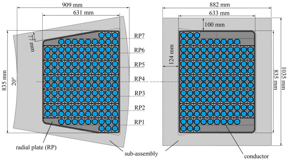
Figure 3.10: ITER winding pack for inboard (left) and outboard leg (right). Picture after [ITE06].
