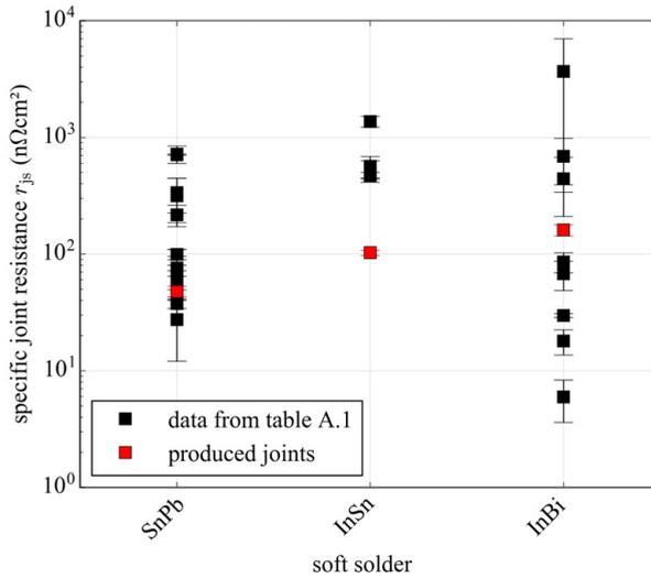
Figure 4.11: Specific joint resistances  $r_{js}$  of reproduced joints compared to data from collected publications on soft solder contacts between 2G high temperature superconductors (table ??). Error bars represent the standard uncertainty  $u$ . The source data of the black markers can be found in in the annex A.1.
