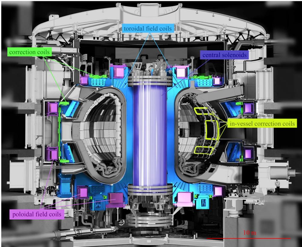
Figure 2.9: Magnet components of ITER. The entire system consists of 18 toroidal, 6 poloidal, 18 correction and 27 in-vessel correction coils and 6 stacked central solenoids. Except for the  $\text{Nb}_3\text{Sn}$  toroidal and central magnets, all coils are made from NbTi. Original picture from [Cre].
