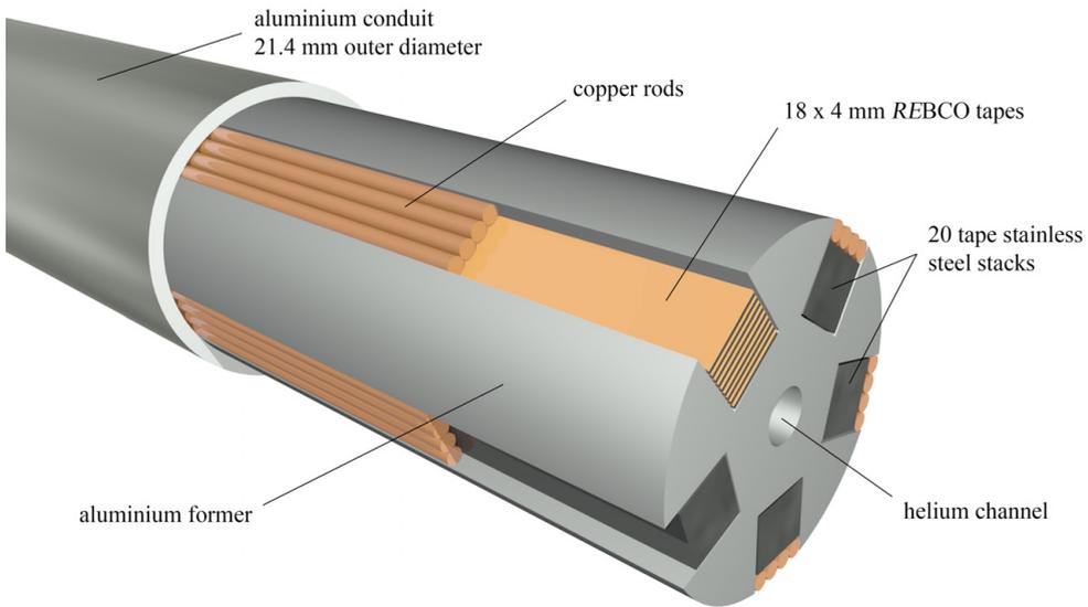
Figure 6.23: Schematic of the 18 tape full-size cable sample C. Only one of the five grooves was equipped with *REBCO* high temperature superconductors.
