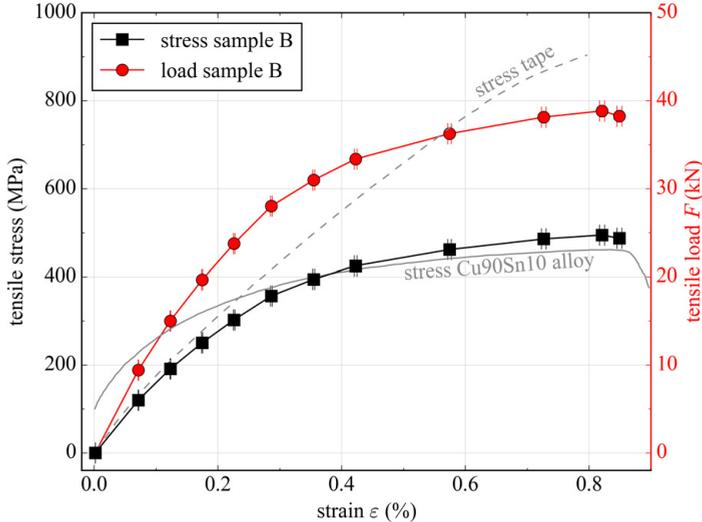
Figure 6.31: Load-strain and stress-strain diagram for sample B. The measurement was performed at 4.2 K inside a 12 T background field. The single tape data is taken from [Bar15, Cop].
