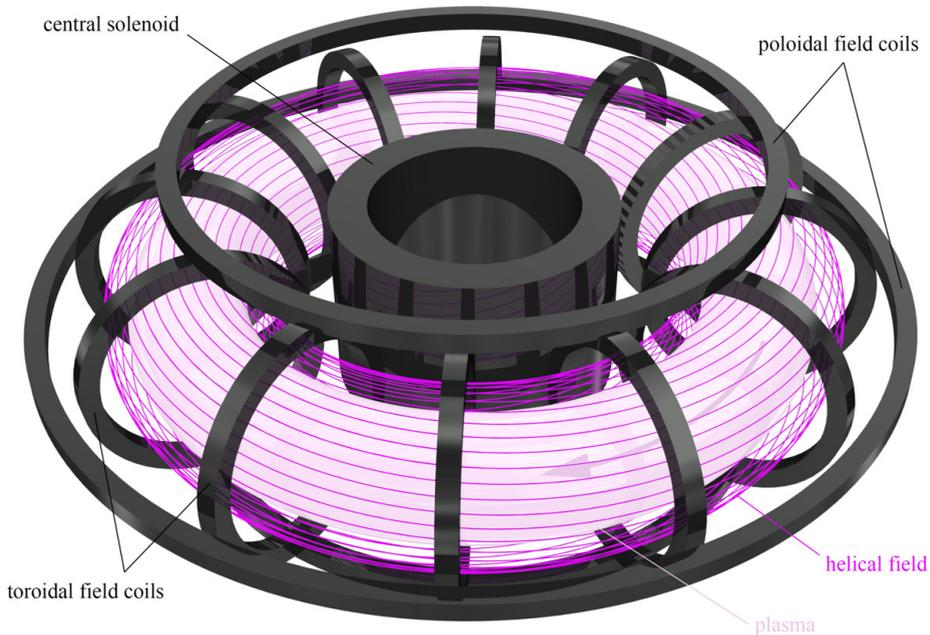
Figure 2.8: Magnetic plasma confinement of a tokamak. The helically wound, magnetic torus yields from superposition of toroidal and poloidal magnetic fields.
