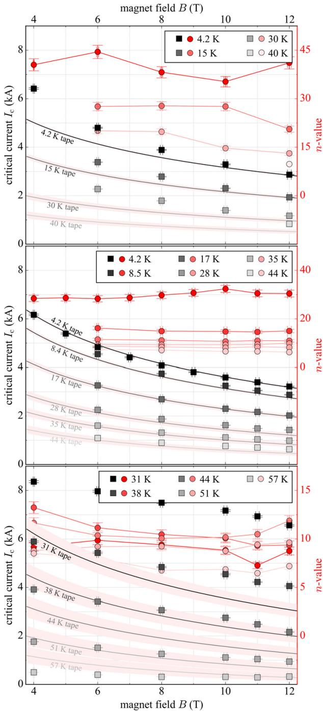
Figure 6.29: In-field performance of sample A, E and F (top down) at various temperatures.
