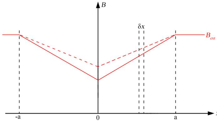
Figure 7.1: External magnetic field penetrating a superconductor before (continuous line) and after the flux jump (dashed line).
