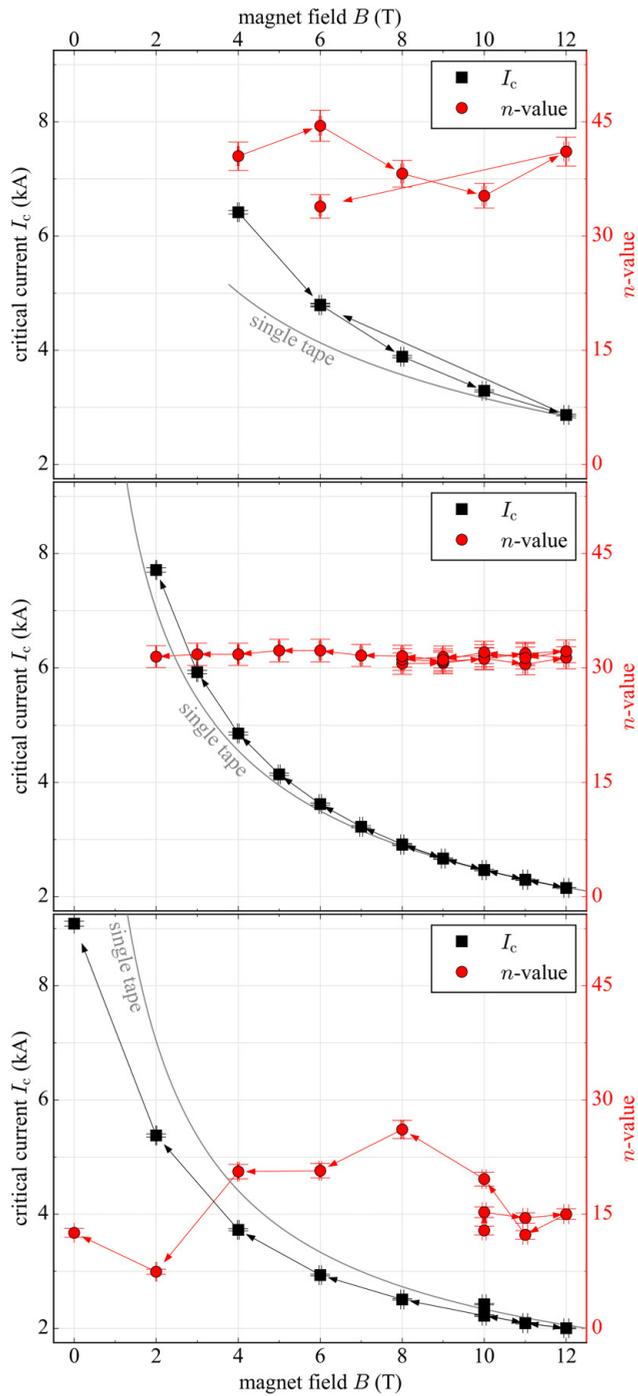
Figure 6.27: In-field performance of sample A, B and C (top down) at 4.2 K.
