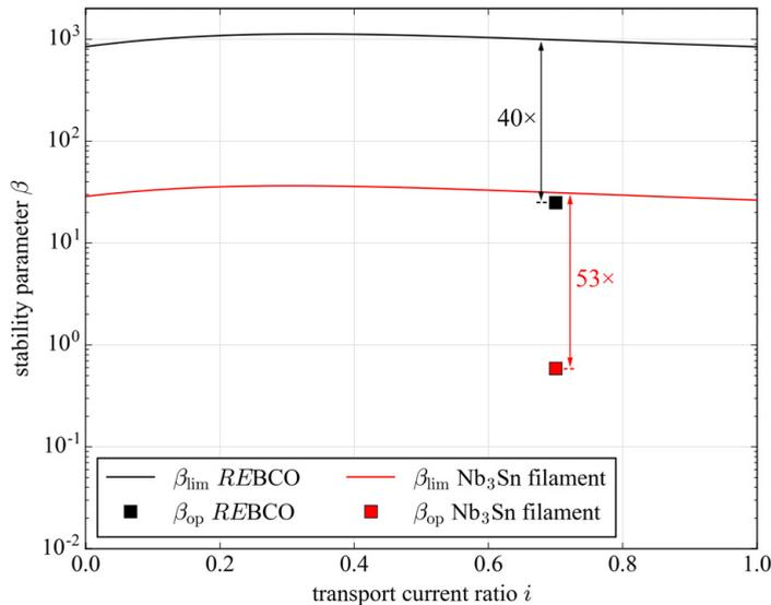
Figure 7.2: Stability parameters of a 0.2 mm wide  $Nb_3Sn$  filament and a 4 mm wide  $REBCO$  tape depending on the ratio of transport current to critical current. For DEMO, the point of operation is at  $i = 0.7$ .
