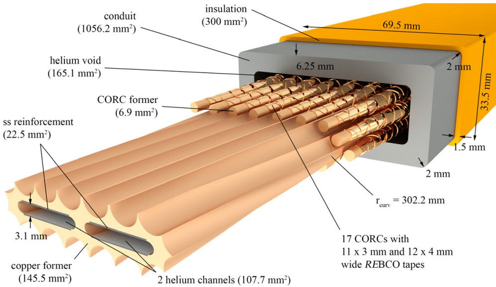
Figure 7.10: Schematic of a feasible DEMO full-size CORC cable.
