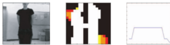
Fig. 10: Johnson and Higgins' navigation aid: the real situation (left), calculated depth map (middle), and the corresponding signals sent to the 14 vibration motors (right)
