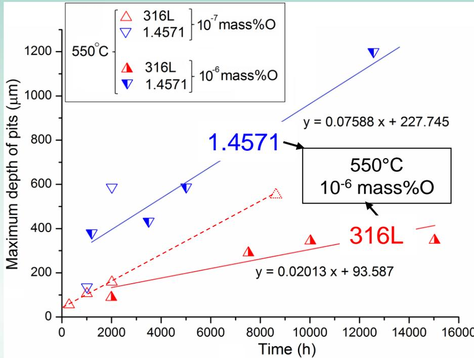
Maximum depth of pit-type corrosion attack on austenitic steels tested in flowing LBE (~ 2 m/s) depending on temperature and oxygen concentration in the melt.
