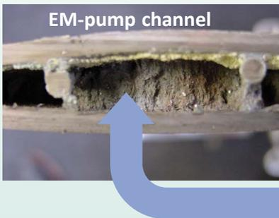
Risk for precipitation of corrosion products  $\rightarrow$  tube plugging
