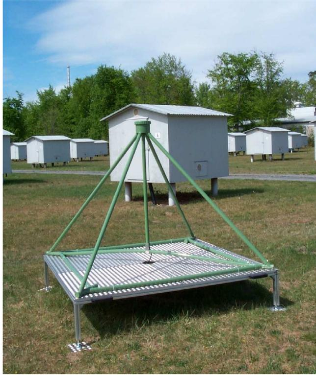
Figure 3.3: Inverted-V-shaped dipole antenna used for most LOPES setups.
