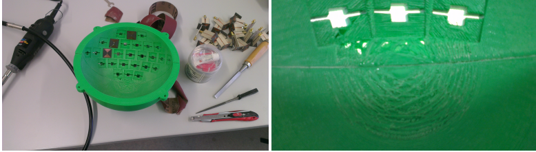
Figure 7.11: The array produced with the 3D-Printer. Unfortunately, the precision of the device was limited, so the work piece had hols and protrusions (left image). Hence, a rework was necessary.
