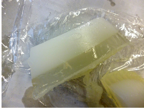
Figure 6.3: Investigations on mixtures containing oil, corn flour, gelatin and water. The part containing oil was separating before the mixture could solidify.
