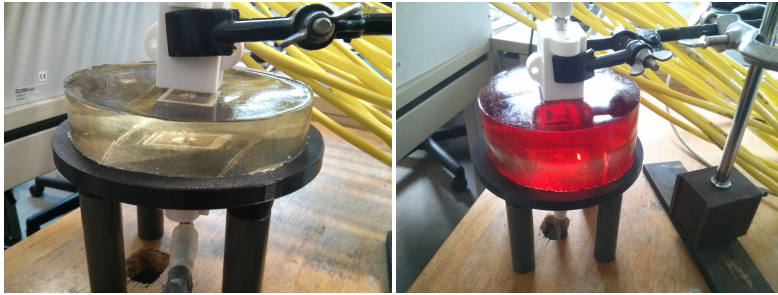
Figure 7.8: The experimental setup of the two setups measured to examine if the feeding could be neglected in simulations. In the left image there is the setup used for the comparison with the simulation containing the feeding and in the right image there is the setup for comparing with the simulation where the feeding was neglected.
