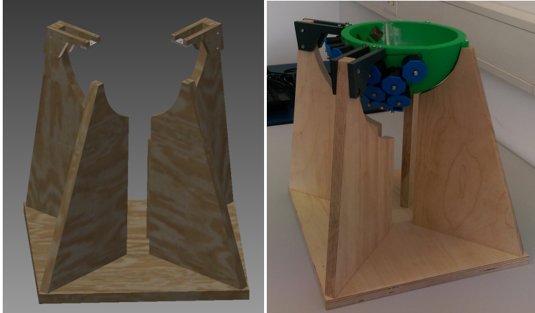
Figure 7.12: The developed holder, which was able to hold the array and the phantom. It was stable enough to endure a great number of experiments. The holder was designed using the CAD software Inventor from Autodesk Inc..
