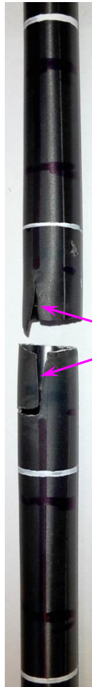
rod #7: stress concentration in the opening middle (similar fracture: rod #1)
