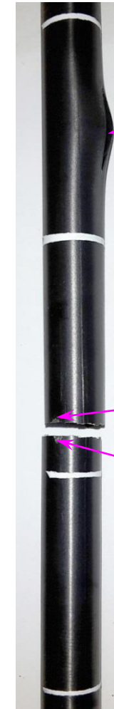
rod #4: not prototypical fracture at TC weld (similar fracture: rod #2)
