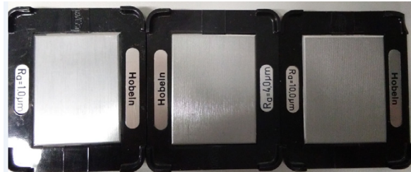
Figure 3: Calibration standards with the different roughness R_a = 1 \mu\text{m} , R_a = 4 \mu\text{m} and R_a = 10 \mu\text{m} (HALLE Praez.-Kalibriernormale GmbH).
