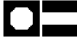
Figure 2: The proposed box filter \mathbf{K}^{Blob} on the left and \mathbf{K}^{Line} on the right for the feature extraction in the CCM images.
