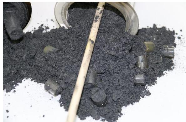
Fig. 2: Carbon powder accumulation in the upper part of the reactor after 14 days of operation.
