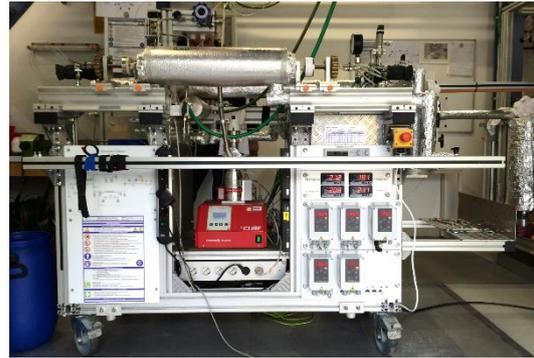
Fig. 2: Mobile testing unit for the investigation of physical fluid properties under reservoir conditions
