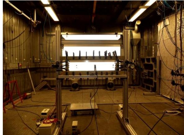
Fig. 3: Experimental set-up for investigating transient flame behavior coupled to flexible walls using transparent walls and optical measurement techniques in HYKA Test Chamber Q160.
