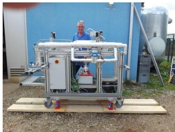
Fig. 4: In-situ measurement of specific heat, density and kinematic viscosity of geothermal brines, developed by the Energy and Process Engineering Group.
