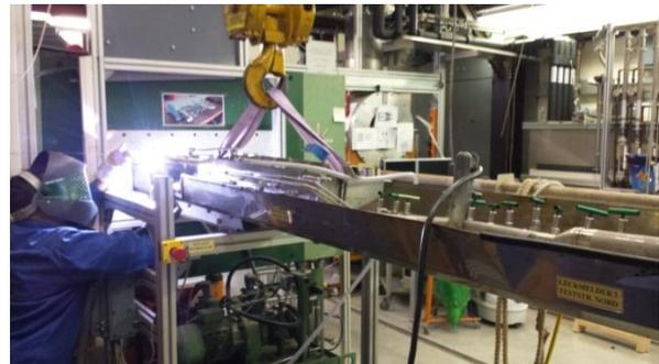
Fig. 6: Magneto-hydrodynamic flow test of a blanket module mock-up in the MEKKA laboratory.
