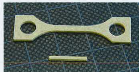
Printed tensile and bending test specimen
