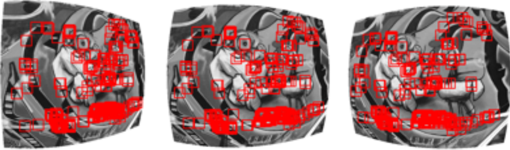
Figure 5.7. Images with 200 tracked ORB features. Depicted are image 1, 7 and 10 from the radial distortion image set. Fisheye images are not displayed here.
