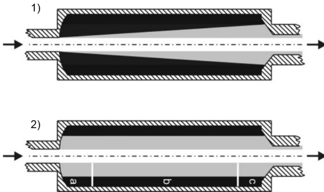
Figure 2: Scheme of sediment distribution within a tubular centrifuge for products with different rheological behavior: 1) with a high yield stress, 2) with a low yield stress (Stahl et al., 2008)
