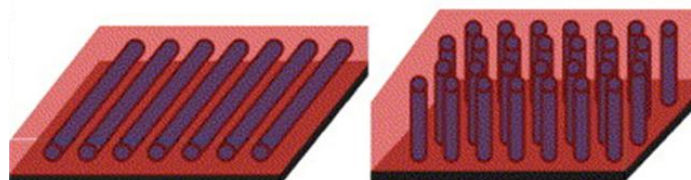
Figure 2.13 Schematic illustration of parallel orientation of a cylinder forming BCP (Left), perpendicular orientation of cylinders (Right). Adapted with permission from ref [168]. Copyright © 2005 Elsevier B.V. All rights reserved.
