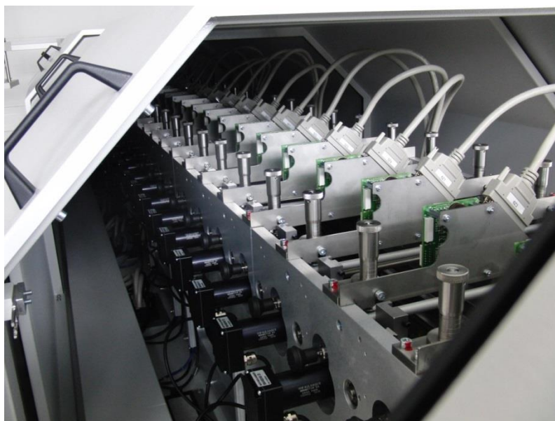
Figure 5: View inside the laser printer used to produce peptide arrays by the xerographic method showing the different cartridges. Image © PEPperPRINT, reproduced with permission. 50
