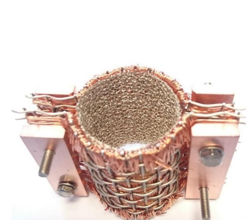
SS mesh with Cu wires + Ni foam
