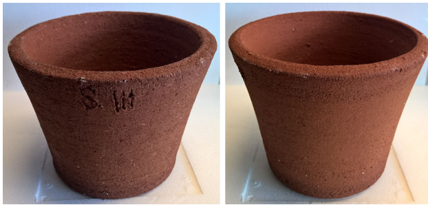
Fig. 8 Ceramic filter pots made of local clay mixed with 40 % rice husks (left) and 40 % sawdust (right)
