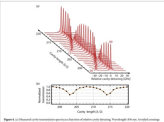
Figure 4. (a) Measured cavity transmission spectra as a function of relative cavity detuning. Wavelength: 856 nm. Avoided crossing: between the fundamental mode and the fourth order modes 04 and 13 are visible. (b) Maximal transmission of each of the spectra shown in (a), normalized to the largest value.
