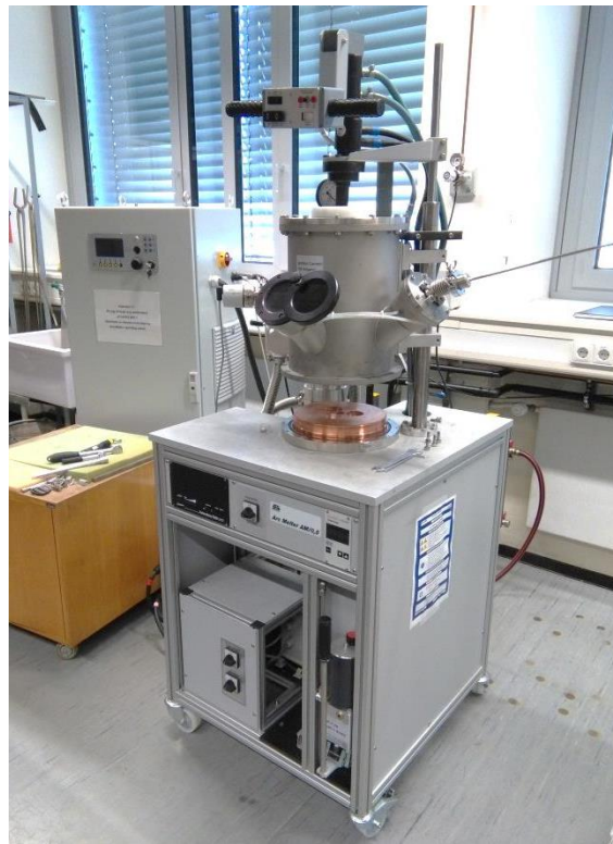
Fig. 3-1 Arc-melting furnace (AM0.5, Edmund Bühler) used in the present work.
