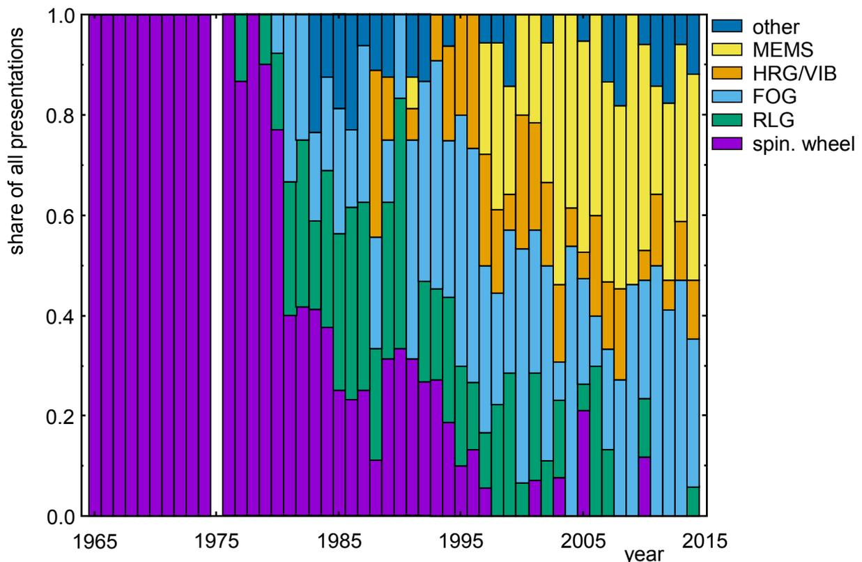
Figure 4. Different types of gyros as presented from 1965 through 2014.
