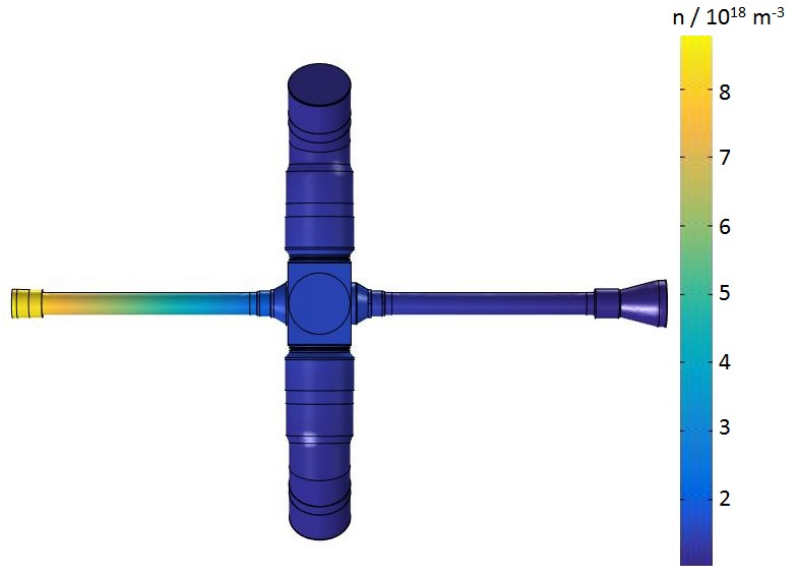
Figure 4.17.: Three-dimensional density distribution of the second pump port of the DPS1 and adjacent beam tubes.
