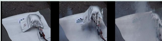
Pouch bag cell during overcharging without protection
