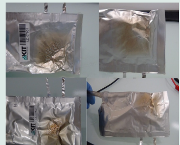
Pouch bag cell after thermal runaway test
