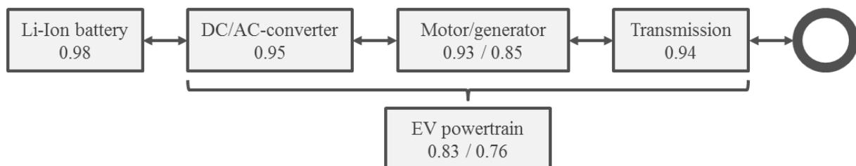
Figure 2: EV powertrain with average measured component efficiency at recorded speed values
