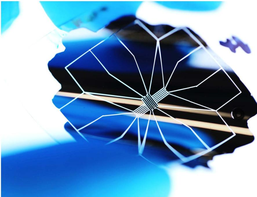
Figure 7.1.: Fully printed flexible photodiode array comprising 36 pixel with dimensions of  $45 \times 175 \mu\text{m}^2$ .
