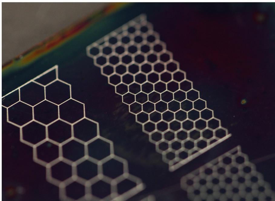
Figure 5.1.: Photograph of a P3HT:PCBM solar cell comprising AJ printed hexagonal Ag grids.
