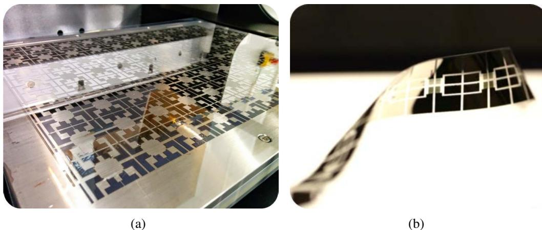
Figure 6.19.: a) Inkjet printed Ag contact pads on PET. b) PET stripe comprising several fully AJ printed OPDs.
