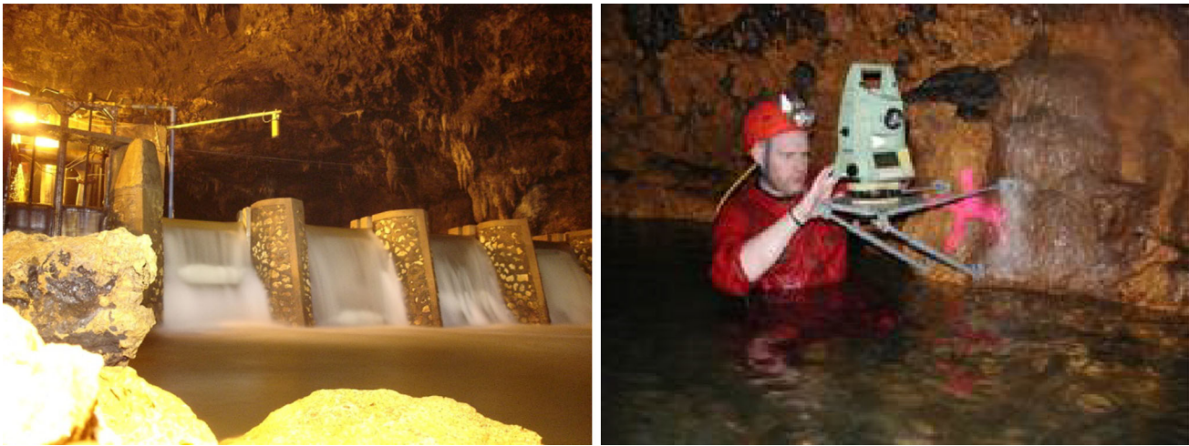
Fig. 6 Continuous discharge monitoring using a radar sensor for contact-free water level measurement ( left ), mapping of the cave using laser-tachymetry ( right )
