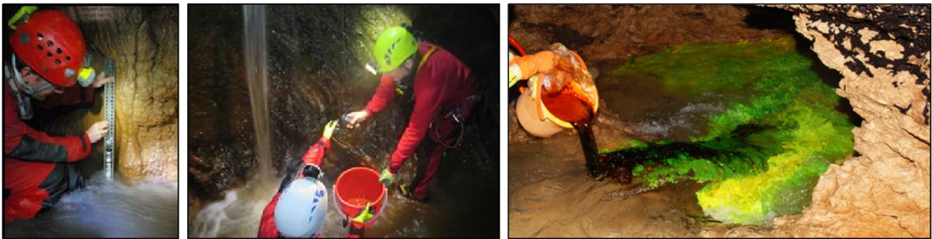
Fig. 11 Installation of pressure sensors for automated water level resp. discharge monitoring in a karst cave ( left ), manual discharge measurement for data validation ( middle ), multi-tracer-test with fluorescence dyes ( right )
