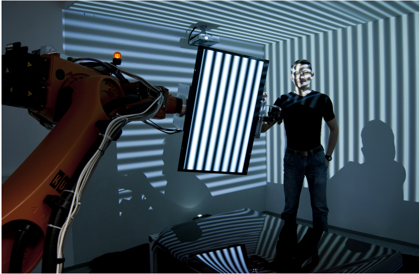
Figure 1.5: Stationary platform: KUKA robot hand for autonomous deflectionometric inspection of varnish coating at IES laboratory [Leh11].
