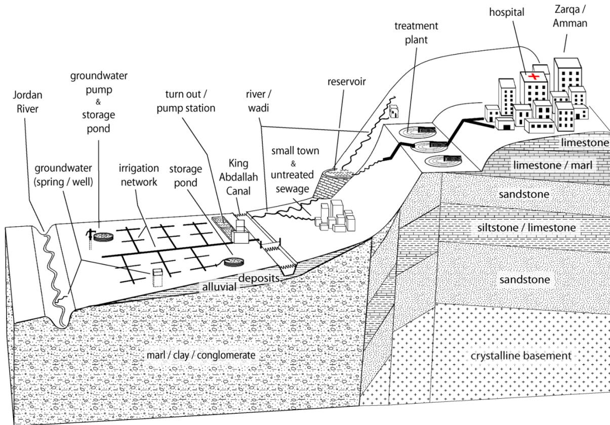
**Figure 13: Schematic block diagram illustrating all relevant water sources, local distribution processes for irrigation, and a simplified geological setting (not to scale).**
