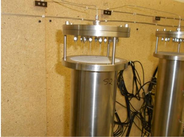
**Figure 6: Trickling of treated wastewater via cannulas on the column surface.**
