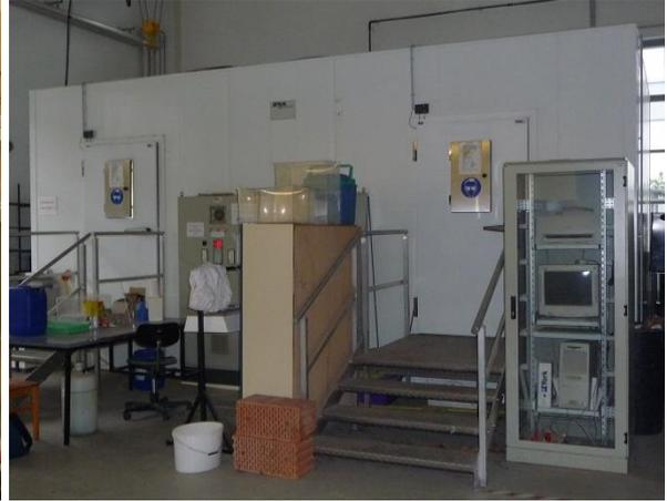
**Figure 7: Climatic chamber.**
