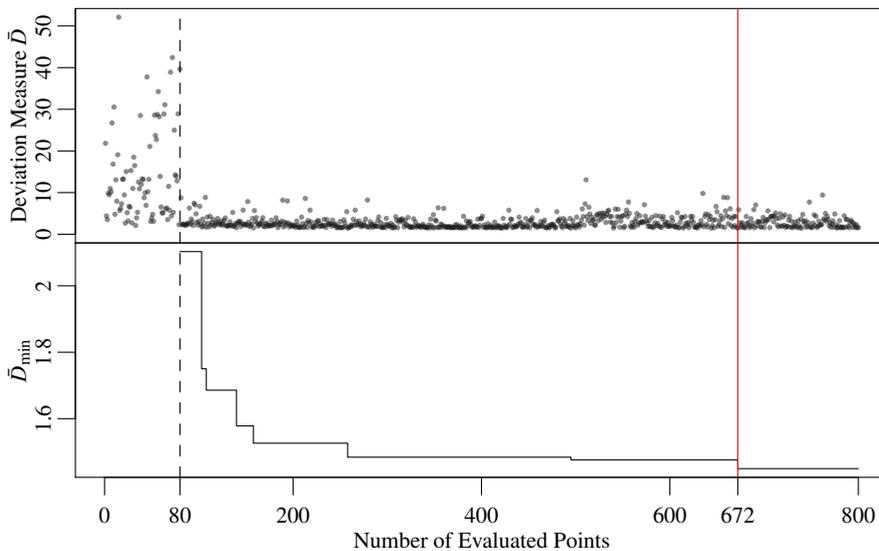
**Fig. 13** Optimization course for the speed combination  $v_c = 270 \frac{m}{min}$ ,  $v_f = 7 \frac{mm}{min}$ . Upper Figure: Deviation measure  $\bar{D}$  for the 800 parameter combinations of  $\theta$ . Lower Figure: Minimal deviation measure from the first 80 evaluations (initial design) to all 800 evaluations. Red line marks the evaluation with the best found parameter combinations of  $\theta$ .
