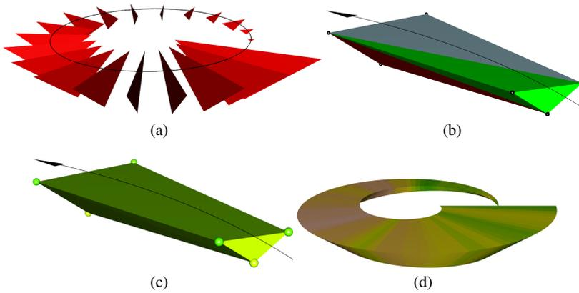
**Fig. 9** (a) Scratch track triangles for the first revolution and (b) tessellation of one scratch track part into three simplexes (red, green and blue), (c) Scratch track part with sampled heterogeneity values for the six points represented by different color shades for the points and the mean value (color of track part) and (d) scratch track of the first revolution with  $v = 100$  observations (scratch track parts) with assigned heterogeneity values.
