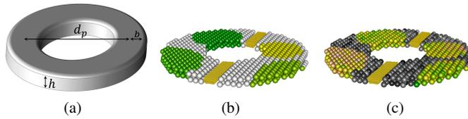
**Fig. 6** (a) Basic shape, (b) coarse grid with steel points (yellow), cement points (grey) and basalt points, (c) coarse grid after point elimination and (d) coarse grid with values (represented by different color shades) from sampled Gaussian random fields
