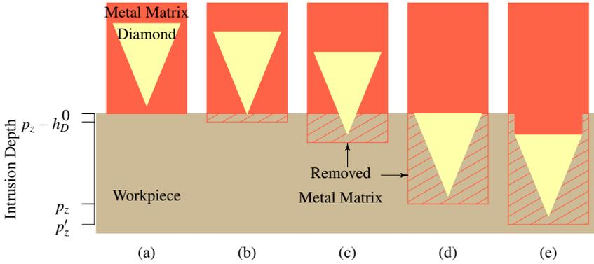
**Fig. 10** (a) First segment workpiece contact with a diamond (yellow) inside the metal matrix (red), (b) First diamond workpiece contact at a cutting depth of  $p_z - h_D$ , (c) Diamond in the intrusion period, (d) Diamond at the end of the intrusion period at a cutting depth of  $p_z$ , (e) Last position of the diamond before break out at  $p'_z$ .
