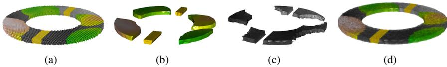
**Fig. 7** (a) Finer grid with interpolated point values, (b) tessellation of basalt grains and reinforced bar, (c) tessellation of cement points and boundary points of the objects and (d) complete workpiece.
