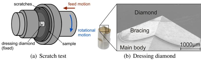
**Fig. 3** Experimental setup for single diamond scratch test.
