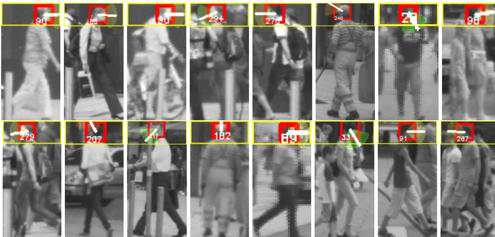
Figure 3.51: Pedestrian head pose estimation results in inner-city scenarios. Color gradient goes from green (frontal pose, i.e., less critical situation) to red (back poses, i.e., dangerous situation).
