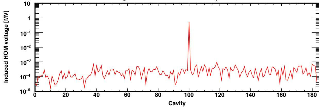
HOM voltage in cavities after beam pulse
