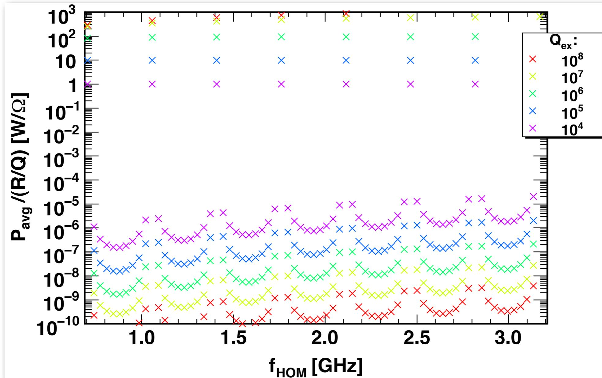
■ Power dissipation is only high at a resonance
