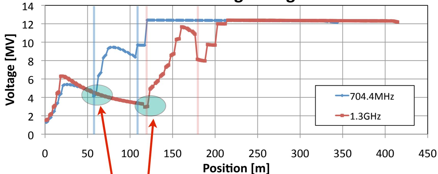
In both cases power per cavity is limited to **0.9 MW** ( $\hat{=} 12\text{MV}@75\text{mA}$ ).
