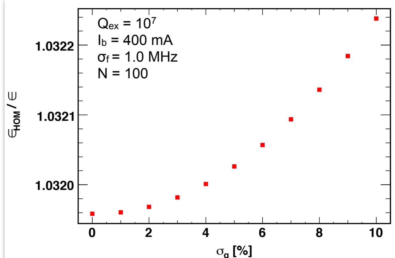
► **Bunch charge scatter drives HOM in longitudinal plane**
