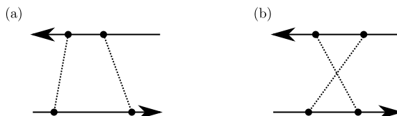
Figure 3.4.: Two exemplary second order contributions to the self-energy \Sigma . In the situation (a) the diagram is reducible, whereas diagram (b) denotes an irreducible second order process. Diagrams are regarded to be reducible if one can cut vertically without crossing a dashed line.
