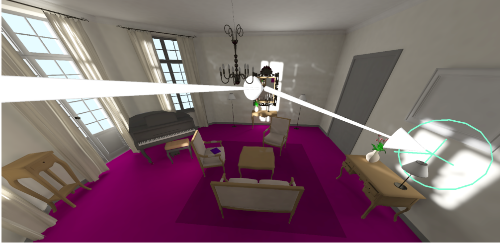
Figure 9.2: The light path inspection tool visualizes the source of the caustic formed by a reflection of the sunlight off a mirror at the back wall. Adapted from [Reiner et al. 2012].
