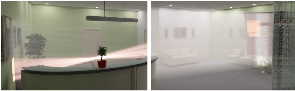
Figure 9.3: Volumetric inspection set to visualize only specular caustics (left), and all lighting components (right). Note how selective inspection emphasizes lighting phenomena. Adapted from [Reiner et al. 2012].
