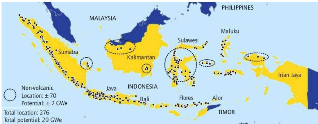
Figure 1. 2: The distribution of geothermal areas in Indonesia [dena, 2012]: 276 geothermal areas and 29 GWel of potential geothermal resources. Circular dashed lines is the symbol for non-volcanic geothermal.
