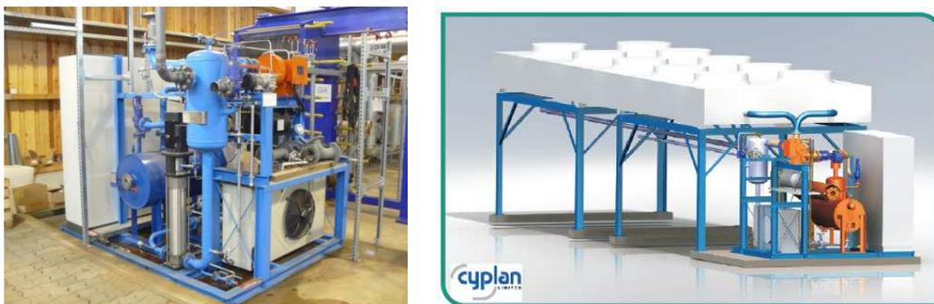
Figure 3. 7: The 60 kWel Groß-Schönebeck ORC system comprises the preheater, evaporator, turbine, air-cooled condensers, hot well, and feed pump. The additional auxiliary component includes lubricant cooler. Courtesy of Durr-Cyplan [2011].
